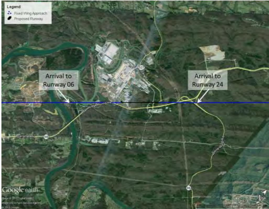
Figure 3-1. Fixed-wing Approach Flight Tracks
