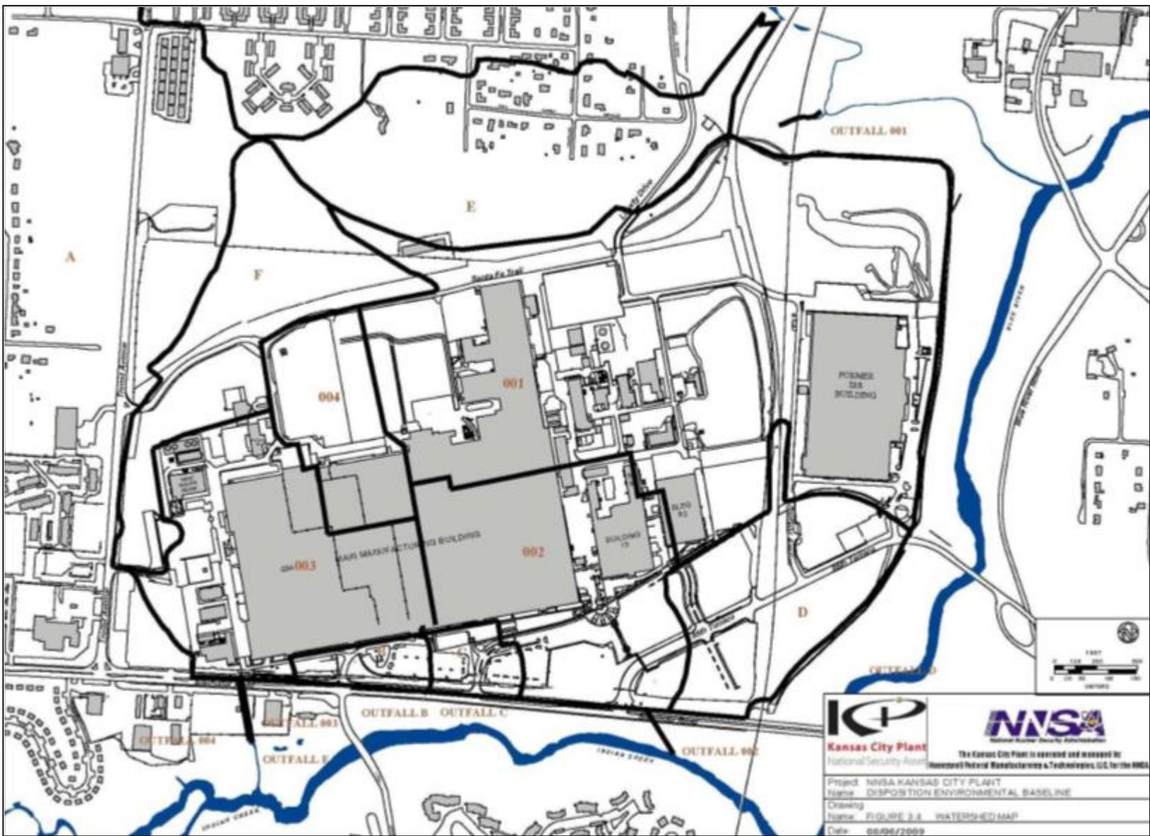
Figure 3-8. Drainage Areas on the BFC and the Outfalls to which They Drain (Source: Honeywell 2013)
