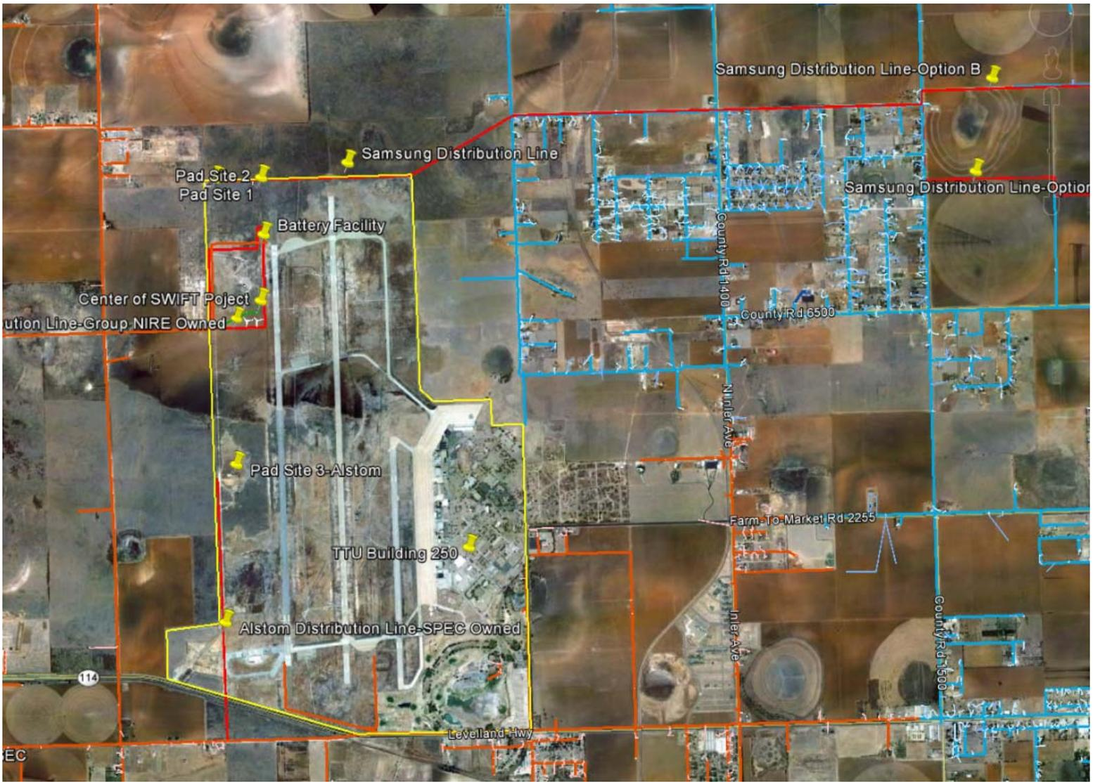
**Figure 2-2.** Vicinity map showing general location of the RTC and the location of the proposed distribution lines storage battery facility, and wind turbines (©Google and NIRE 2012).
