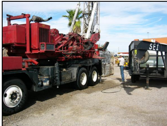
Photograph 2-6 Example of a Auger Rig
