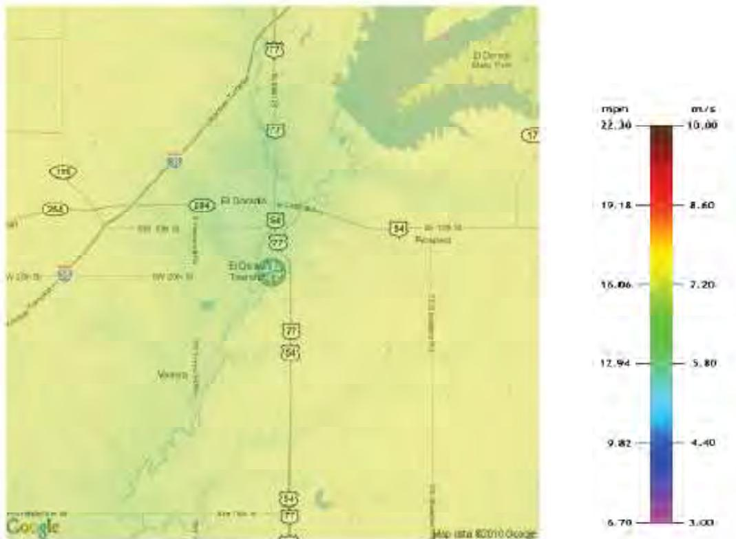
Figure 2.3.1a: Mean annual wind speed at 60m height
