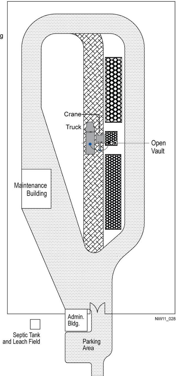
Figure 2-2. Conceptual remote-handled low-level waste facility layout.
