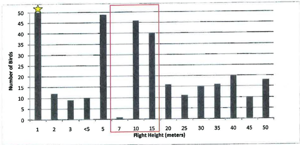
The yellow star represents a total of 183 birds at one meter high. The red box shows the approximate height range of the turbine rotor. Source: Kennedy 2012.
