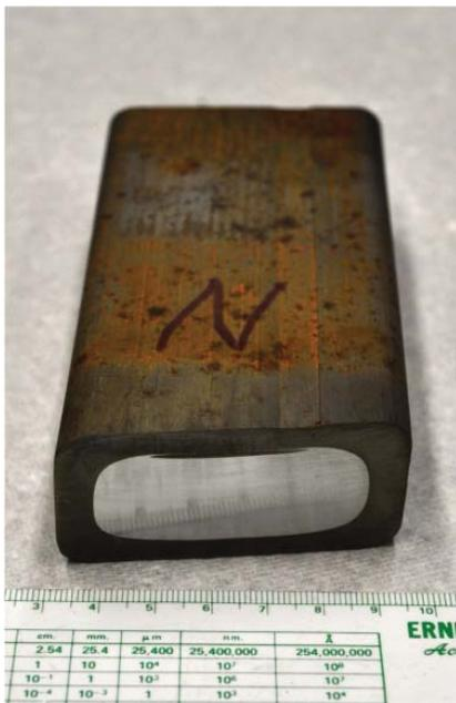
Figure 1. A 2.4-kilogram extruded bar of 14YWT advanced ODS alloy.
