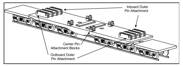
Figure 1. Atlas Railcar Standardized Attachment Components.
