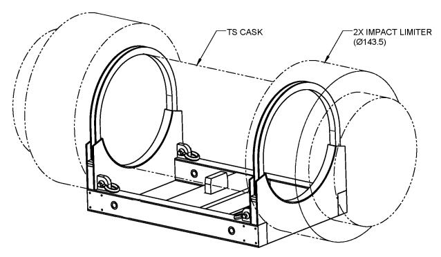
Figure D-3. Family 3 EnergySolutions TS125 Conceptual Cradle Design.
