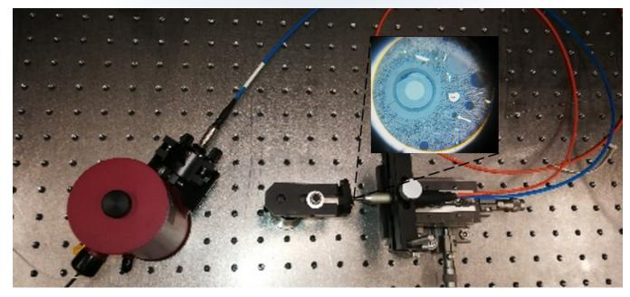
Figure 1. Proof of concept system using a fiber-optic to collect black body irradiation associated with transient laser heating. The inset shows an optical micrograph of the fiber end facing the sample.
