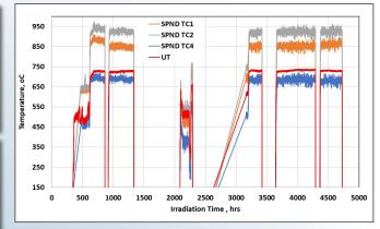
Figure 2. Temperature data from UT and thermocouples from ATR irradiation.
