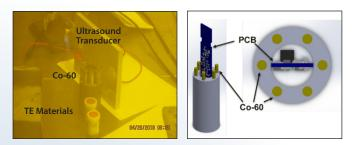
Figure 4. Gamma radiation test in hot cell at Westinghouse.
