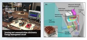
Figure 1. The prototype system of the self-powered ultrasound data communication and sensing (upper-left) and illustration of its installation in the nuclear canisters (lower-right).
