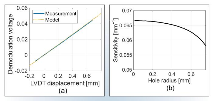
Figure 4 (a) Comparison of modeled and measured sensor performance. (b) LVDT sensitivity versus central hole radius.
