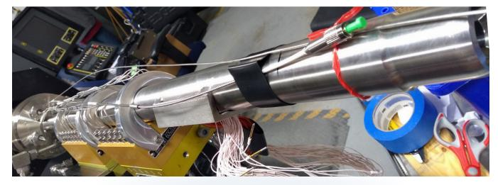
Figure 2. Top: Schematic of optical fiber sensor. Bottom: One of the FBG sensors installed in the HDG-1 experiment.
