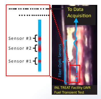
Figure 1. Concept diagram for Sapphire single-mode fiber optic development towards high-temperature radiation-resilient sensors. (Right) a frame from a CEN-224T 450 cal/gm transient test of LWR Fuel in TREAT at INL taken from https://www.youtube.com/watch?v=h0o4P\_F4s9s.
