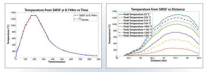
Figure 3. (Left) Temperature determined from spectral shift by a third order fit during descending temperature shift measured by Luna's OBR 4600 versus time at the point of peak furnace temperature is shown in blue. The dotted yellow line is the reading of a type-B thermocouple co-located at this point. (Right) Furnace temperature as a function of distance during several times as determined by the SMSF measurements. There are 30 gauges shown along this length of fiber.
