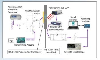
Figure 2. Schematic of ultrasound text transmission.
