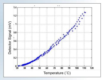
Figure 2. Signal improved by more than 100 times with elevated temperature (from room temperature to 110 °C). Good repeatability was observed from heating up and cooling down procedure.
