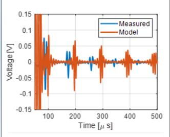
Figure 4. Voltage across the AC coil induced by acoustic echoes at room temperature. (Both experimental measurements and finite element simulation results).
