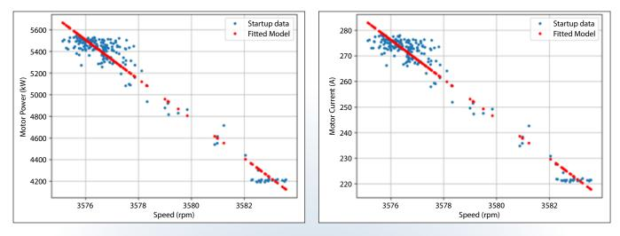
Figure 3. Calibration of motor input power model (left) and motor current model (right).
