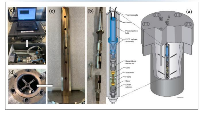
Figure 1 – (a) schematic of the Creep Test Rig inside autoclave, (b) actual parts of the Creep Test Rig with SS 304 sample, (c) Creep Test Rig all together and ready for testing, (d) Creep Test Rig positioned in static autoclave, (e) NI data acquisition system for recording TC and LVDT signals. [3,5].
