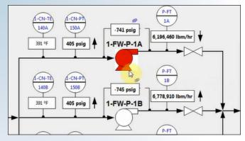
Figure 2. Process and instrument diagram for feedwater pump system.
