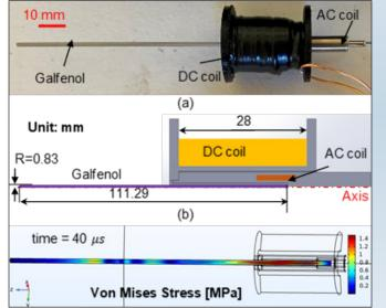
Figure 3. (a) Physical assembly of the pulse-echo mode ultrasonic thermometer with an additional DC bias coil. (b) 2D axisymmetric model layout in COMSOL Multiphysics. (c) Simulated compressive wave propagating in the Galfenol wire (40 µs after excitation).
