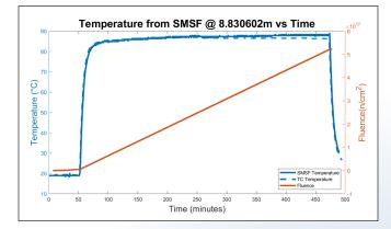
Figure 4. SMSF determined temperature as a function of time irradiated along with collocated thermocouple measurement.
