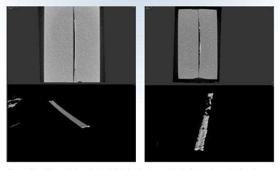
Figure 3. X-ray CT scan of the melt wires (left) before heating, and (right) after heating to 1000°C inside a furnace. The upper images show a cross section of the entire chip, and the lower images show just the meltwire.
