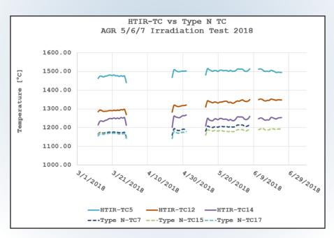
Figure 1. A small window of data for the AGR 5/6/7 results of HTIR-TCs and Type N TCs; showing the HTIR-TCs outlasted and outperformed the Type N TCs in near vicinity.
