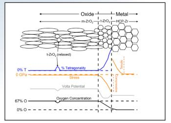
Figure 3. Schematic summarizing the different parameters for each zirconia and zirconium phase.
