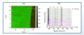
Figure 2. Ramen mapping for Zr alloy: (a) Co localized mixed intensity maps presenting tetragonal, T1 (red) and monoclinic, M4 (green) peaks. (b) Waterfall of Raman spectra near the metal/ oxide interface, corresponding to the dotted line in the mixed intensity map.
