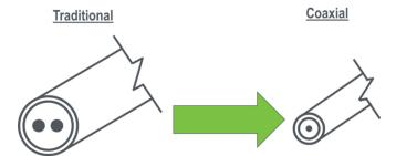
Figure 2. Traditional HTIR-TC mineral insulated metal sheathed cabling versus the optimized "coaxial" cabling. The coaxial cable provides builds with longer lengths, smaller diameters, and more robust performance.
