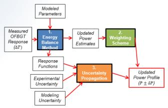
Figure 5. OFBGT data analytic methodology.
