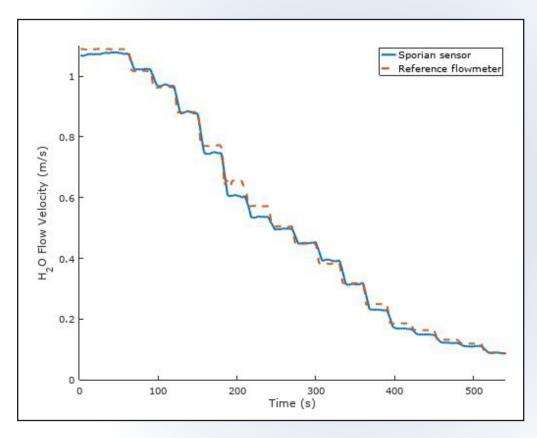
Figure 2. Sporian thermal sensor vs commercial turbine flowmeter, with a transition to turbulence above 0.5 m/s.
