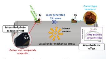
Figure 3. Laser assisted stress sensor [9].
