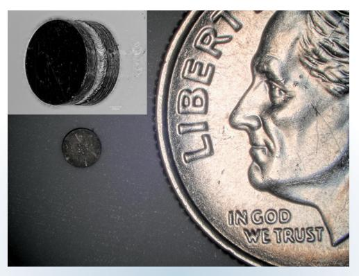
Figure 2. 2-mm-diameter melt wire sensor chip alongside a dime. The inset shows clear view of laser welded chip.
