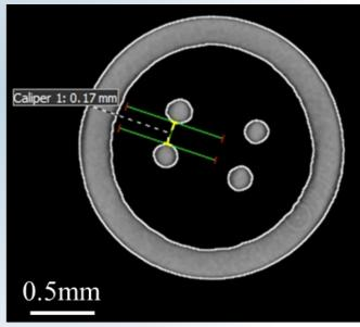
Figure 1. Cross section of the sample and needle probe geometry.
