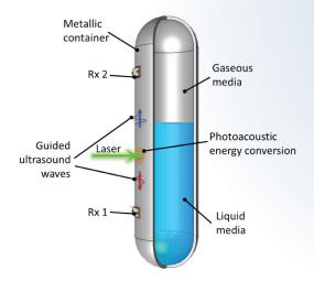
Figure 4. Laser-assisted HT liquid level sensor.
