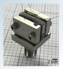
Figure 2. Vibration sensor for NPP application [8].
