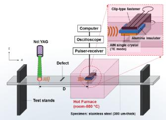
Figure 5. Laser-assisted HT damage detector [10].
