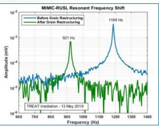
Figure 2. Resonant frequency before and after grain restructuring.
