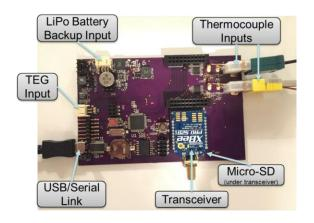
*Thermoelectric generator powered wireless sensor node prototype.*
