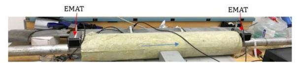
Setup of Lamb Wave EMAT to EMAT signal transmission along a stainless steel schedule-160 pipe with thermal insulation.
