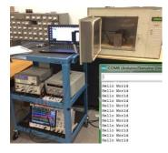
*The experiment setup for throughwall communication at 300°C.*
