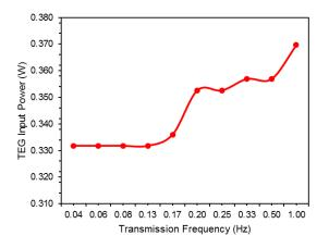
*TEG input power versus frequency of data transmission.*
