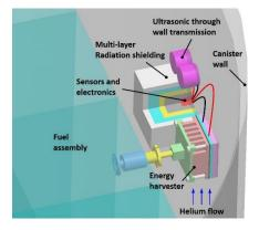
*Energy harvesting for sensing and communicating system powering.*
