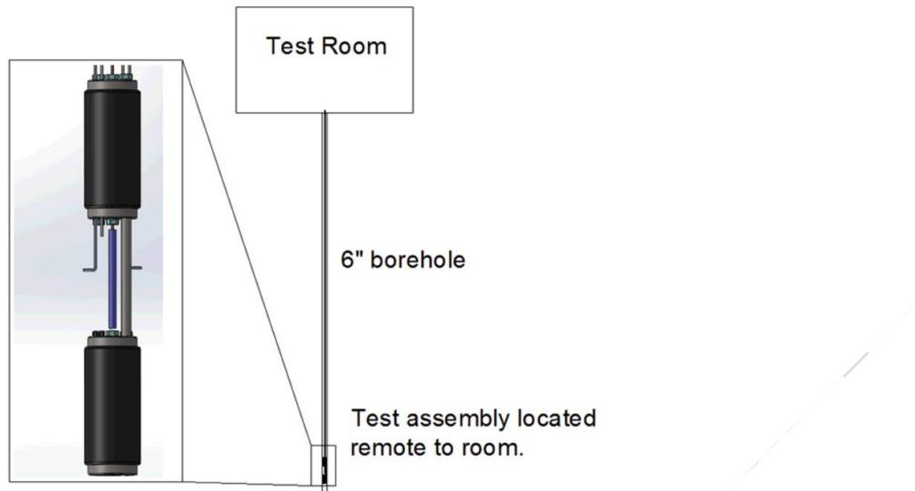
**Figure 3.** Schematic of a Standardized Vertical Borehole Heater Test in Salt.
