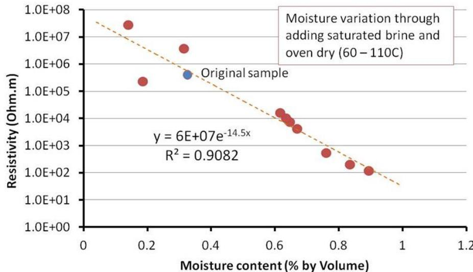
Figure 32. Correlation between Resistivity (1Hz) and Moisture Content
