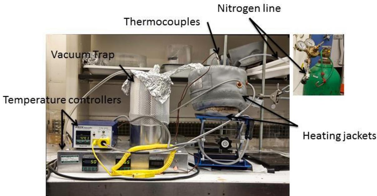
**Figure 28. Testing Deuterium Spiked Water Fractionation in Salt.**
