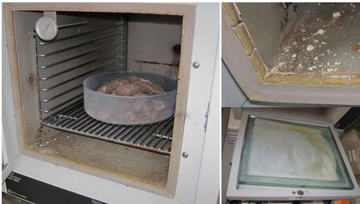
**Figure 27.** Oven Corrosion after Heating WIPP salt from Clay Seam F to 360 °C.
