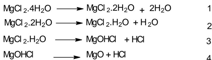
Figure 25 shows HCl generation is expected from  $\text{MgCl}_2 \cdot 4\text{H}_2\text{O}$  in the temperature range 210–445 °C and then from 450–650 °C. The data in Figure 25 were obtained under ambient pressure and water vapor conditions in an open cylindrical oven and reflect the temperature regime under which these processes could be relevant under ambient pressure conditions in the life cycle of a salt repository and could have significant implications for choice of the backfill
