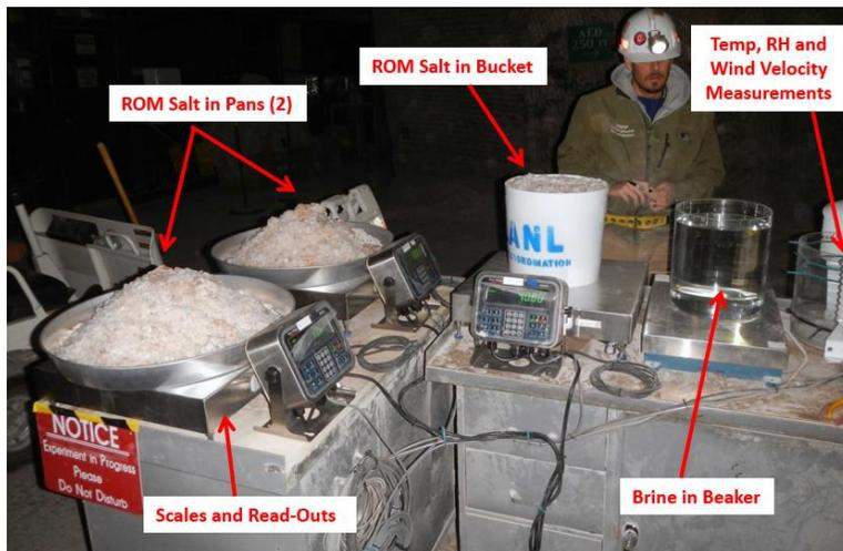
**Figure 24.** Brine and RoM Evaporation Experiments in WIPP.
