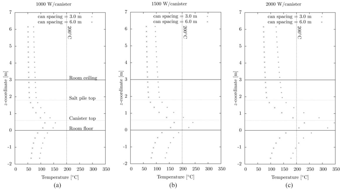
**Figure 18.** Steady state vertical temperature profiles for 1000W, 1500W, and 2000W canisters at 3 m and 6 m spacings (from Harp et al., 2014). Note: Temperatures far in excess of 200°C would probably not be considered in an actual design but are included here to illustrate the sensitivity of maximum temperature to the combination of spacing and thermal load.
