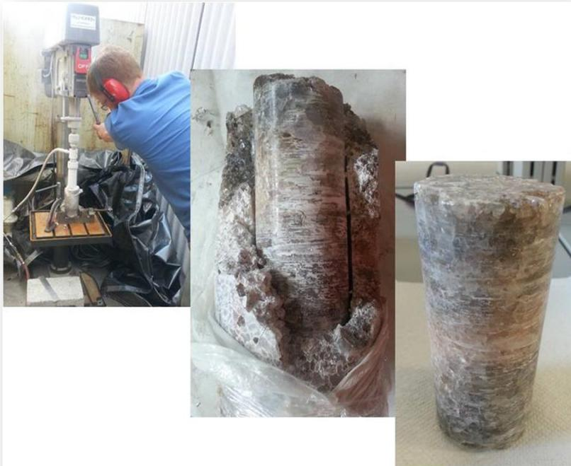
**Figure 29.** ERT Test Core Extraction Images.
