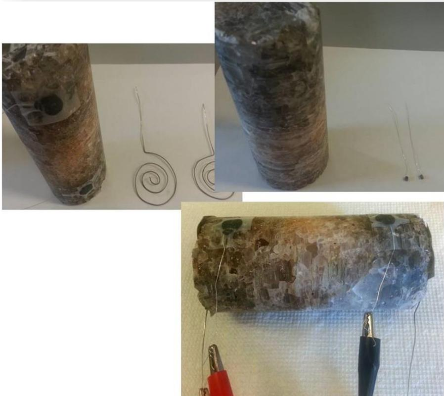
**Figure 30.** ERT Measurement Setup
