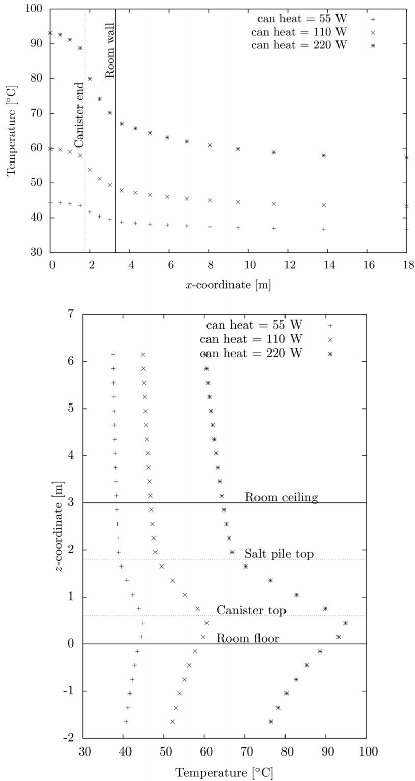
**Figure 16.** Steady-state horizontal (top) and vertical (bottom) temperature profiles for closely spaced canisters (0.9 m or 3 ft center-to-center spacing) in the defense waste repository model (from Harp et al., 2014)
