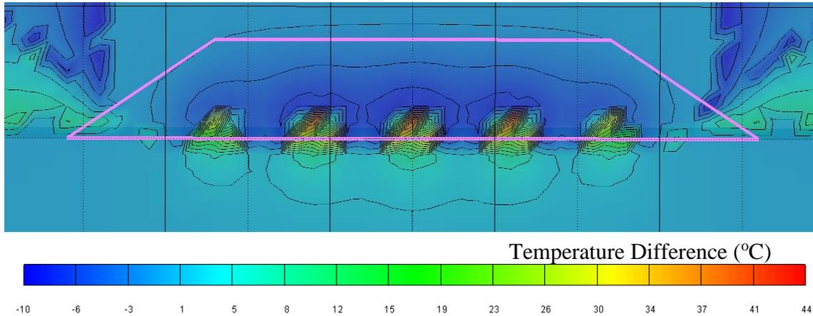
**Figure 19.** Temperature difference between a conduction-only and coupled TH simulation after 2 years (from Stauffer et al., 2012). This plot records the difference between the conduction-only temperature and the coupled TH temperature at each location. Red colors represent a higher (by as much as 44°C) temperature in the conduction-only model.
