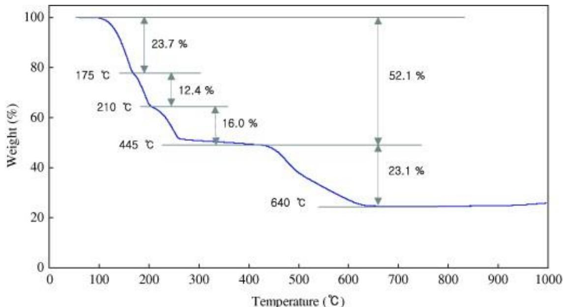
**Figure 25.** Thermogravimetric (TGA) Curve Showing the Dehydration of Magnesium Chloride in Air (Hyoung-Choon, 2010).
