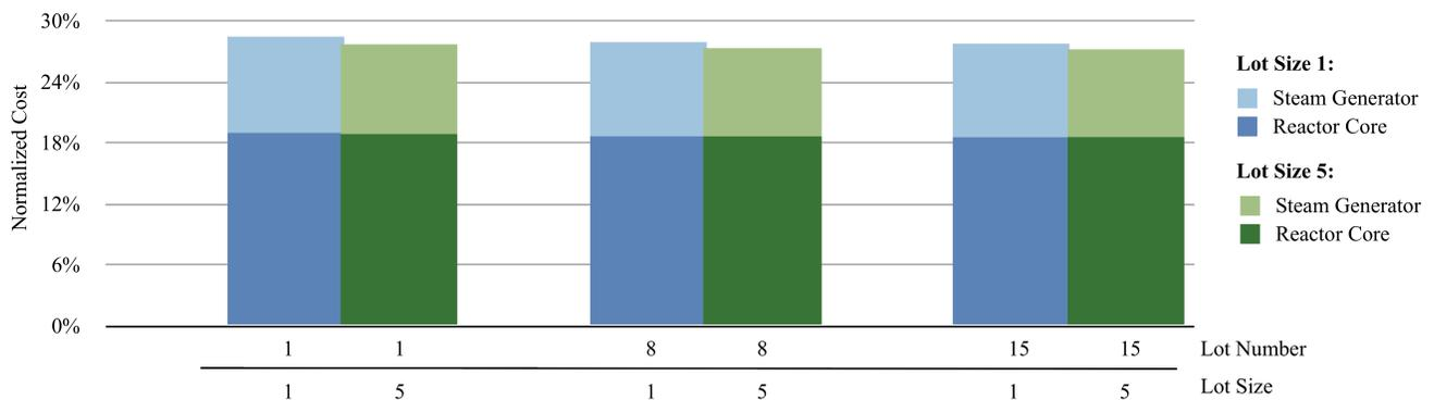
Figure 4: Normalized Cost Contributions – Reactor Core and Steam Generator Subcomponents.
