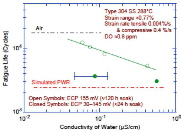
Figure 19. Effects of conductivity of water and soaking period on fatigue life of Type 304 SS in high-DO water.<sup>8,39</sup>
