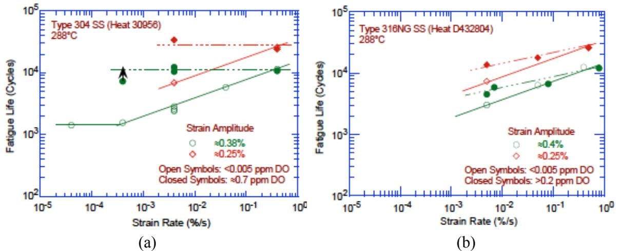
Figure 18. Dependence of fatigue life of Types (a) 304 and (b) 316NG stainless steel on strain rate in high- and low-DO water at 288°C. <sup>8,39,41</sup>
