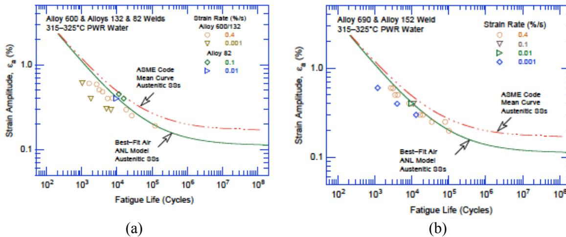
Figure 25. Fatigue  $\epsilon$ -N behavior for Alloys 600 and 690 and their weld alloys in simulated PWR water at 315 or 325°C.<sup>34,85</sup>
