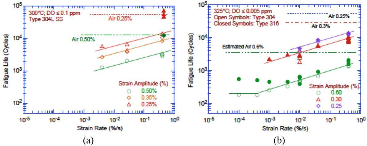
Figure 17. Dependence of fatigue lives of austenitic stainless steels on strain rate in low-DO water. <sup>8,39,41,69</sup>
