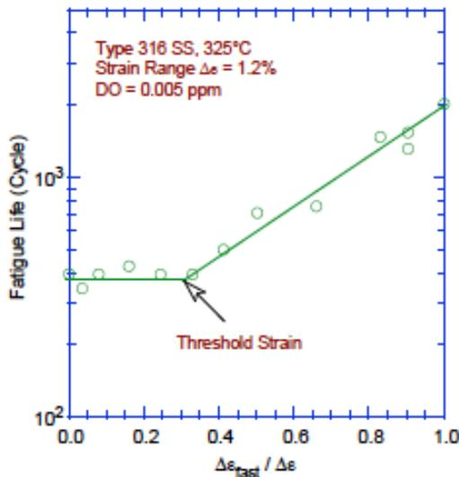
Figure 15. Results of strain rate change tests on Type 316 SS in low-DO water at 325°C. Low strain rate was applied during only a fraction of tensile loading cycle. Fatigue life is plotted as a function of fraction of strain at high strain rate (Refs. 25,30).
