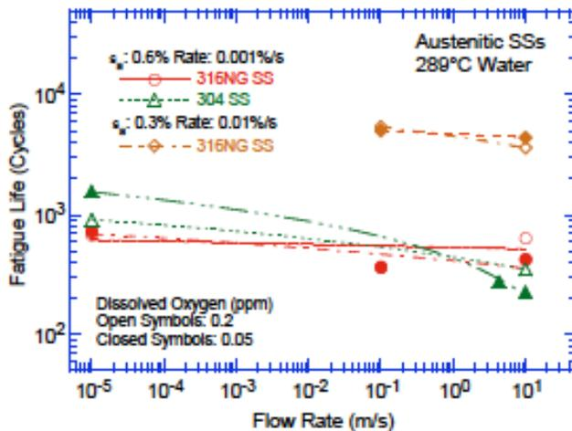
Figure 22. Effect of water flow rate on the fatigue life of austenitic SSs in high-purity water at 289°C.<sup>21</sup>
