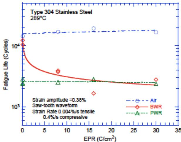
Figure 21. The effect of material heat treatment on fatigue life of Type 304 stainless steel in air, BWR and PWR environments at 289°C,  $\approx 0.38\%$  strain amplitude, sawtooth waveform, and 0.004%/s tensile strain rate.<sup>41</sup>
