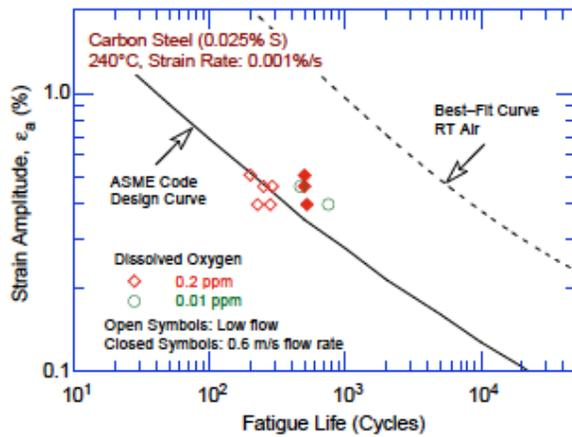
Figure 10. Effect of flow rate on low-cycle fatigue of carbon steel tube bends in high-purity water at 240°C.<sup>72</sup> RT = room temperature.
