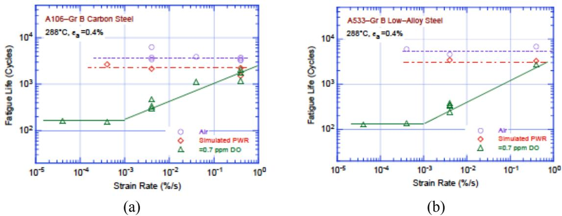
Figure 2. Dependence of fatigue life of carbon and low-alloy steels on strain rate.<sup>5, 18</sup>
