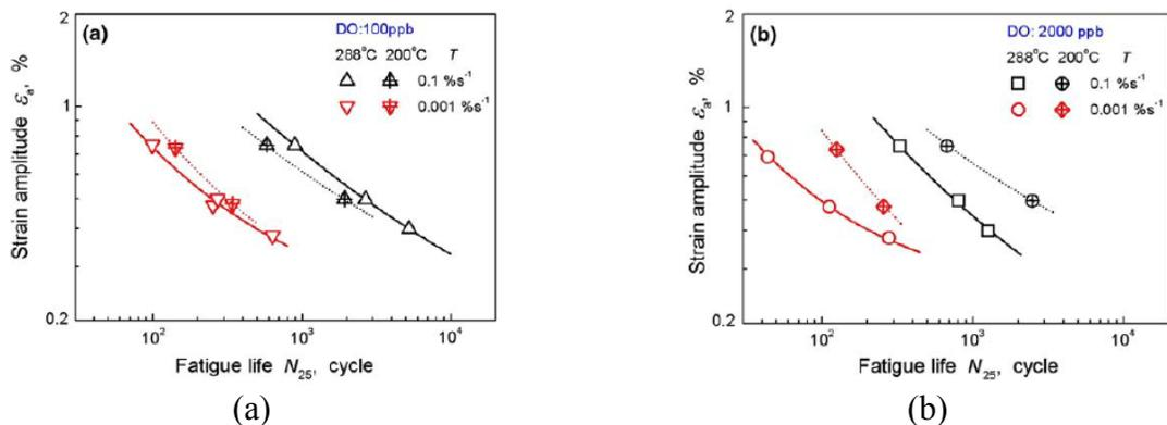
Figure 4. The relationship between fatigue life and applied strain amplitude in high temperature water. (a) DO =100 ppb, (b) DO =2,000 ppb.<sup>67</sup>
