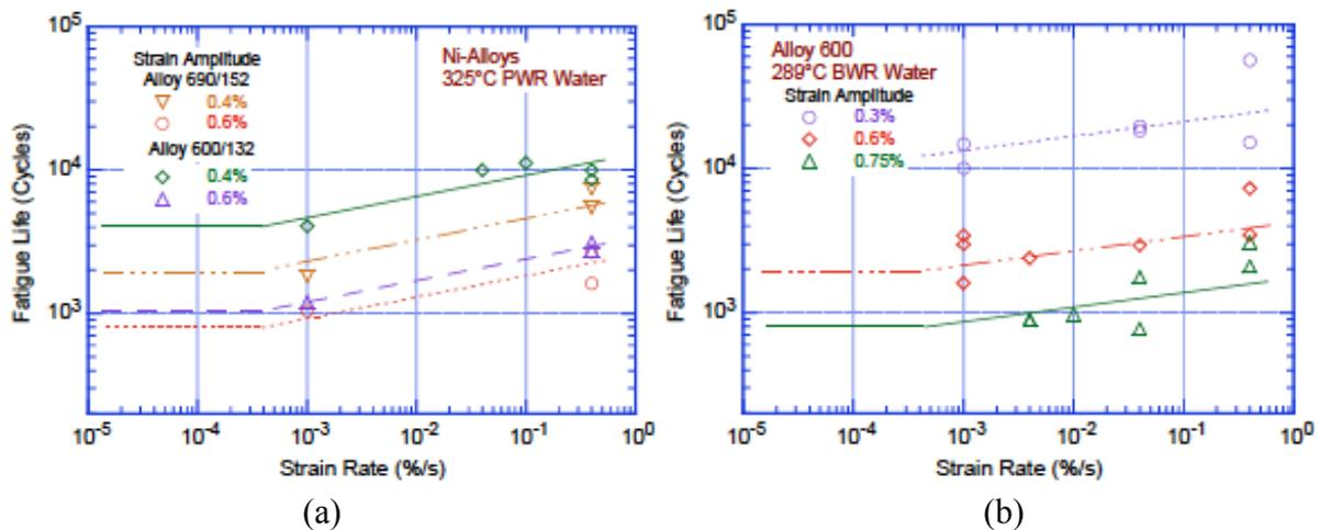
Figure 26. Dependence of fatigue lives of Alloys 690 and 600 and their weld alloys in PWR water at 325°C and Alloy 600 in BWR water at 289°C. <sup>34,85</sup>
