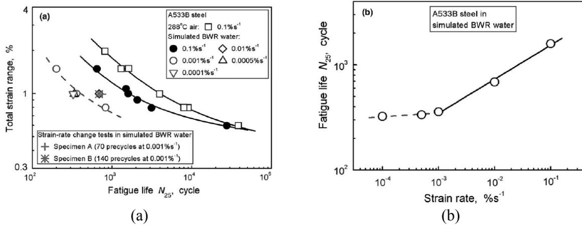
Figure 3. (a) S–N curves of A533B steel in simulated BWR water and 288\_C air and (b) strain-rate dependence of fatigue life in simulated BWR water.<sup>66</sup>
