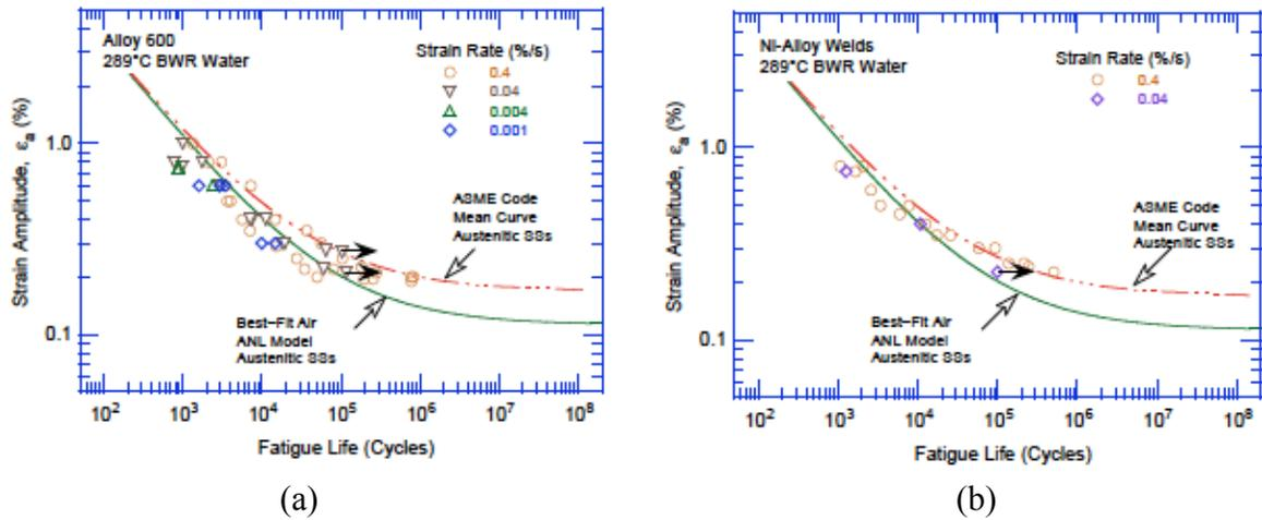
Figure 24. Fatigue  $\epsilon$ -N behavior for Alloy 600 and its weld alloys in simulated BWR water at  $\approx 289^\circ\text{C}$ .<sup>34</sup>
