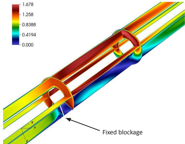
Fig. 3. Flow velocity contours from high-fidelity Nek5000 simulations of flow through the annular test section of the SIBERIA flow blockage experiment.
