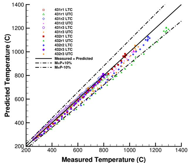
Fig. 4. Comparison of BISON predictions with actual measurements of BOL temperatures in IFAs 431 and 432. (The solid line is where modeled and measured values are equal.)
