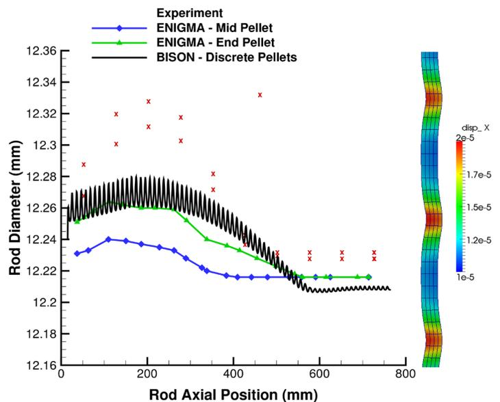
Fig. 6. Simulation of PCMI results from the Risø GE7 experiment: (left) cladding diameter after power ramp (rod position is with respect to the rod bottom) and (right) section of simulated cladding exaggerated to show the "bamboo" effect.
