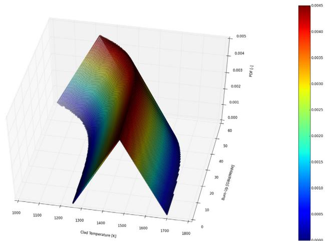
Fig. 10. Probability distribution function of the cladding failure temperature as a function of burnup.
