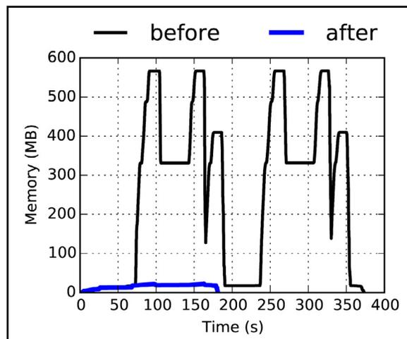
Fig. 4. Comparison of MOOSE memory use and processing speed before and after optimization.
