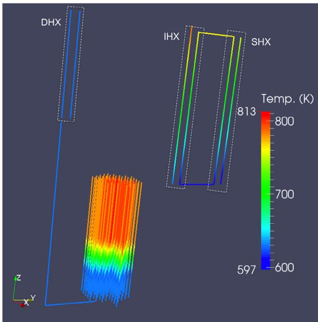
Fig. 5. Temperature distribution in the ABTR during a protected-loss-of-flow transient.
