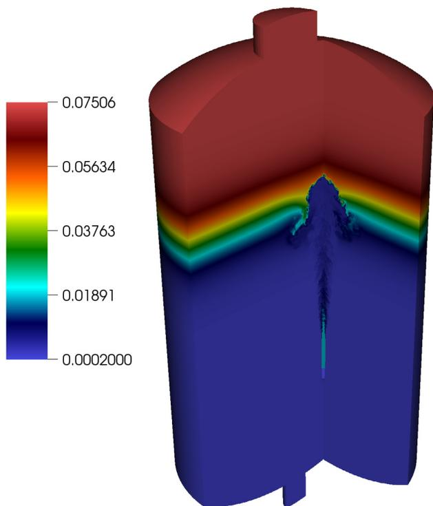
Fig. 8. Pseudocolor plot of helium mass fraction at early times of PANDA simulation with low-Mach number approximation. A vertical jet of larger helium fraction (light blue) has penetrated the initial stratification layer separating the helium-rich region (red) from the air-rich region (blue) of the vessel.
