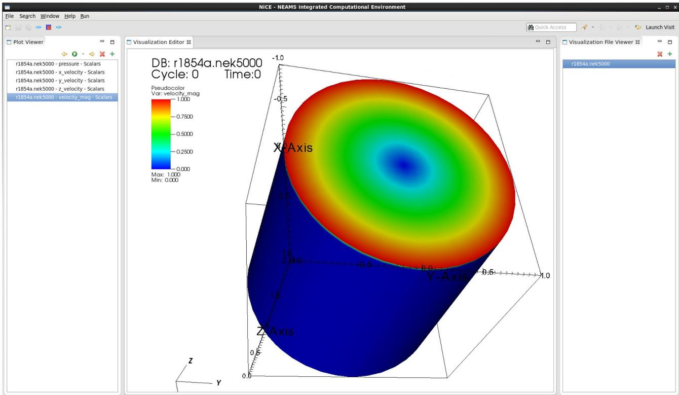
Fig. 13. Screen shot of the updated NiCE user environment with embedded VisIt visualization of multidimensional fuel pellet data.
