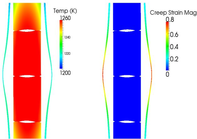
*Fig. 2. Ballooning of zircaloy cladding under LOCA conditions using an enhanced creep model.*
