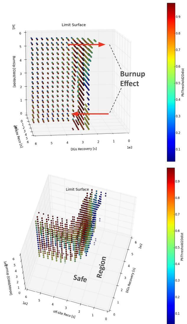
Fig. 11. Limit surface delimiting safe from unsafe region in the input space. (See text for explanation.)
