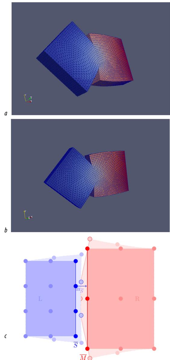
Fig. 1. BISON simulation of two contacting tetrahedral meshes: (a and b) two views of the full mesh and (c) detail showing node-to-node interaction.
