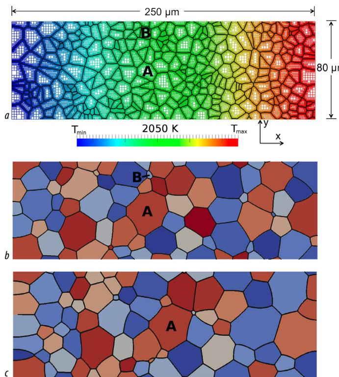
Fig. 3. MARMOT simulations of grain growth: (a) initial fine microstructure, (b) growth under isothermal conditions, and (c) growth under a thermal gradient. Note the growth of grain A at the expense of other grains, such as B.
