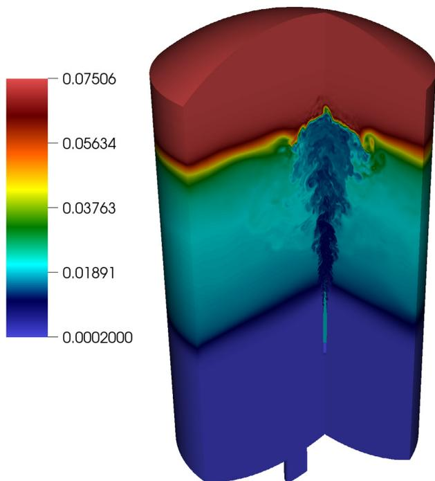
Fig. 9. Pseudocolor plot of helium mass fraction at the final simulation time of PANDA simulation with Boussinesq approximation. Helium from the pipe inlet (light blue) has filled a significant portion of the vessel, eroding the initial stratification layer. The geometry is simplified to speed up the simulation.
