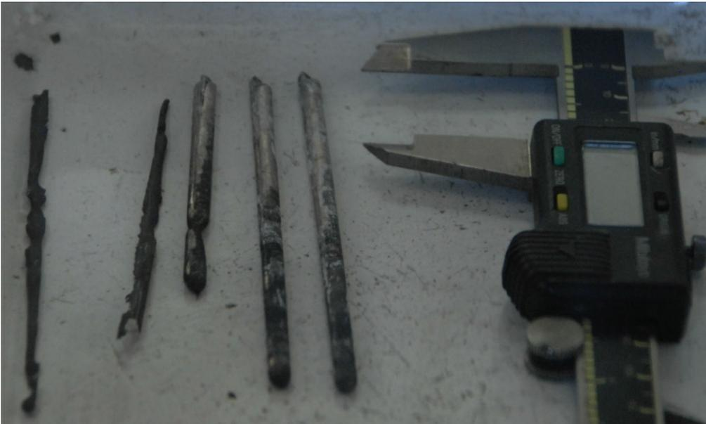
Figure 3. Resuting pins and drips from the U-TRU-Zr casting experiment (calipers are set at 25.4mm)
