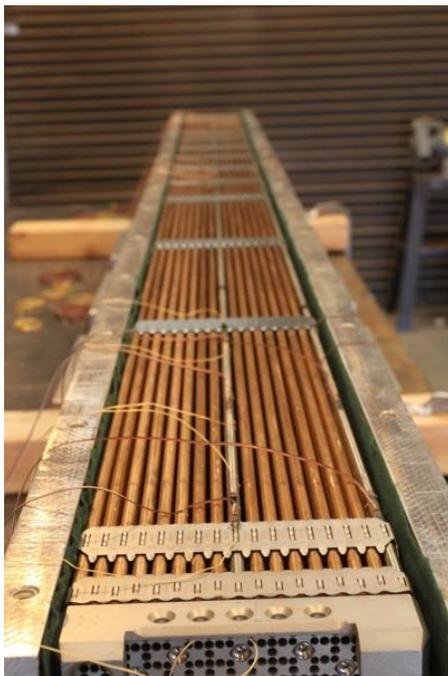
Figure 1. Surrogate PWR assembly with instrumented rods within the basket.
