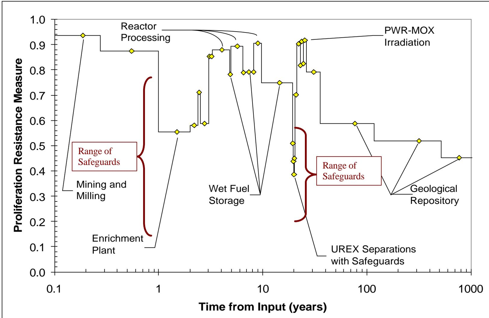
Figure 5 – Proliferation Resistance Measure of a Single Fuel Assembly for All Steps in the Fuel Cycle with UREX and Neptunium Doping
