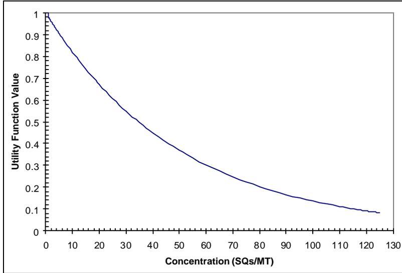
Fig. 3. Concentration of fissile material utility function.
