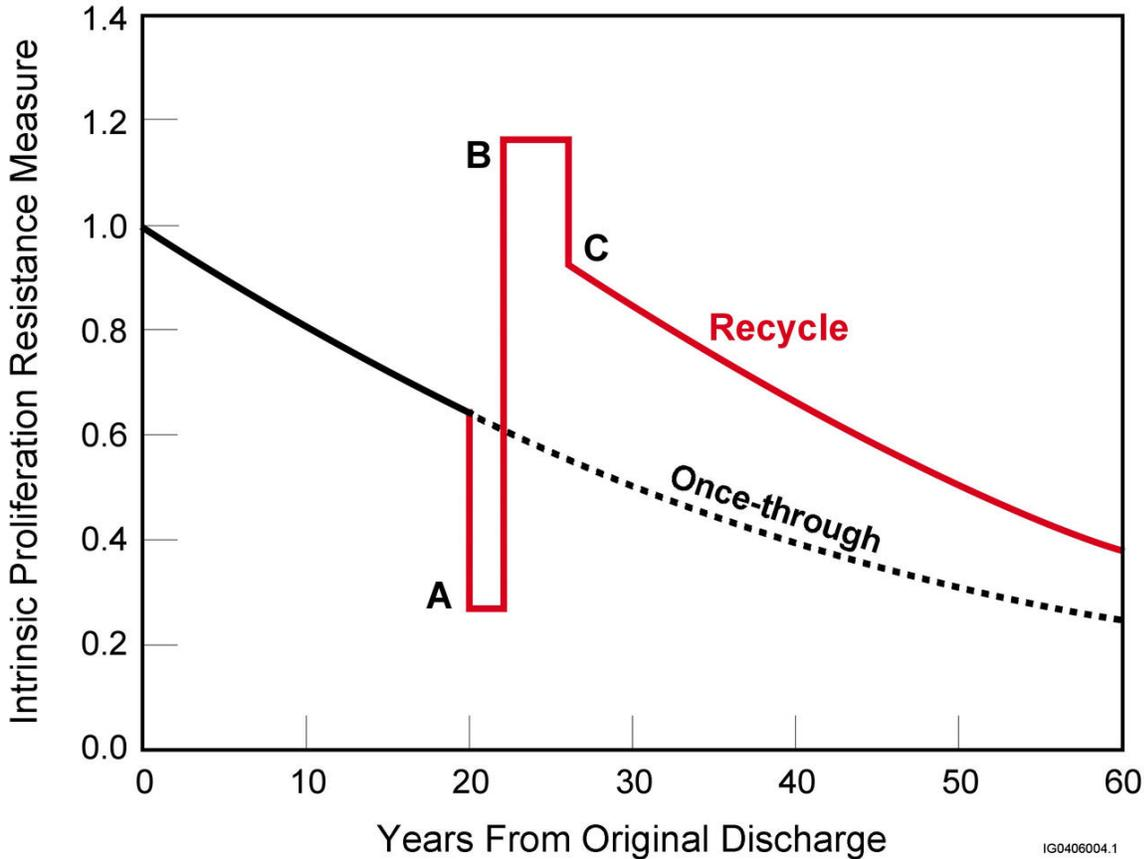
**Figure 1 – Intrinsic Time-Dependent Proliferation Resistance Measure of a Single Fuel Assembly**
