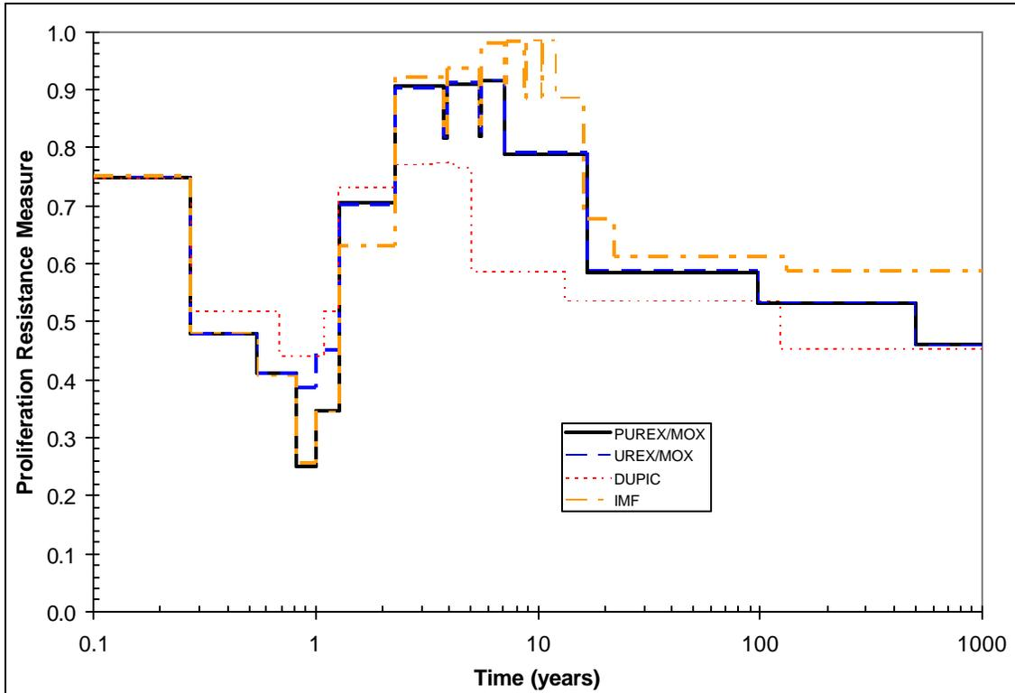
Figure 4 – Proliferation Resistance Measure of a Single Fuel Assembly as a Function of Time for Four Fuel Cycles
