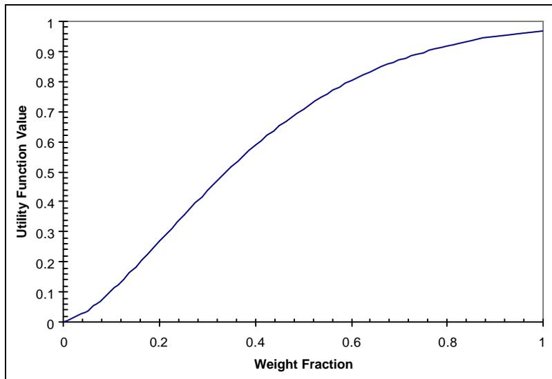
Fig. 2. Weight fraction of even Pu isotopes utility function.
