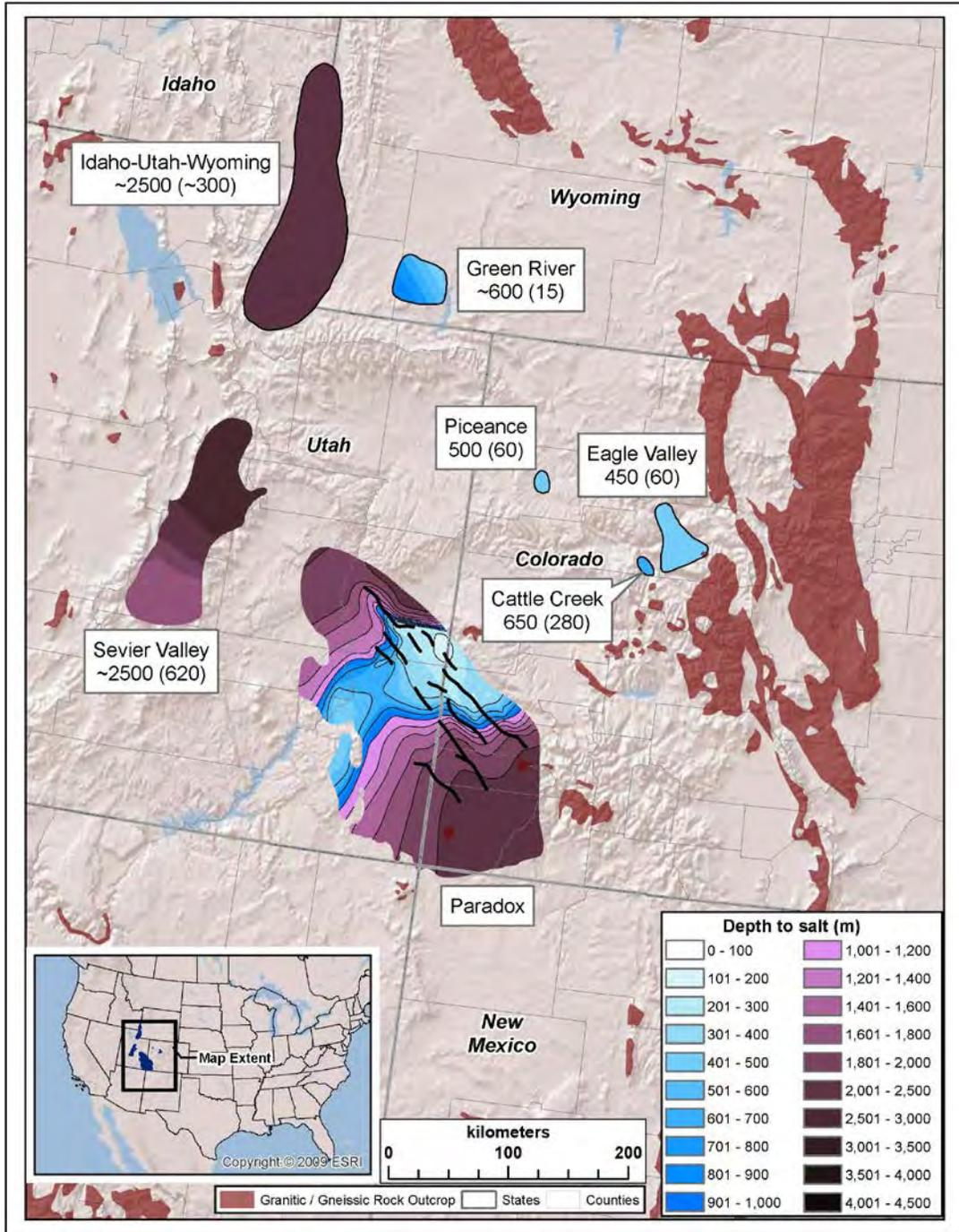
**Figure 4-28.** Location of salt bodies in Colorado, Utah and Wyoming. Depth to top and maximum thickness (in parentheses) of each salt body is listed in units of meters. More detailed information for the Paradox salt is illustrated in Figure 4-8. Data for approximate depths and thicknesses are from Johnson and Gonzales (1978) and Ege (1985), except for salt in the Paradox Basin.
