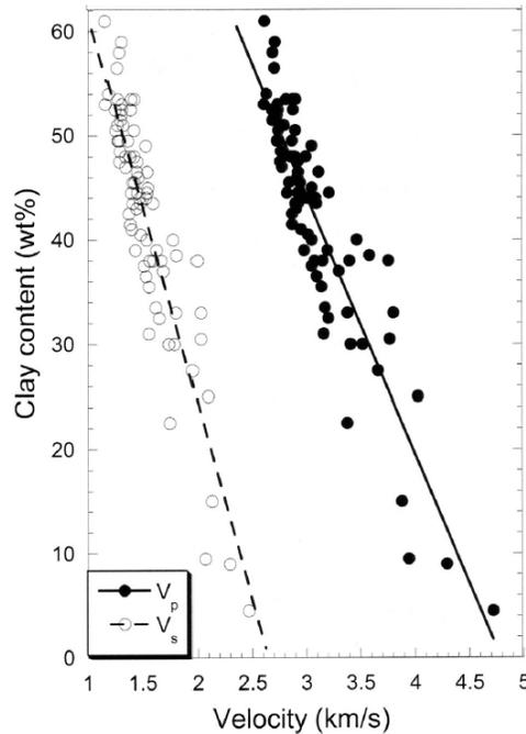
**Figure 6-3.** Correlation between clay content and sonic and shear velocities for the Callovo-Oxfordian clay. Solid line is for Equations (6-5) (for  $V_p$ ) and dotted line for (6-6) (for  $V_s$ ). (Cosenza et al., 2014).
