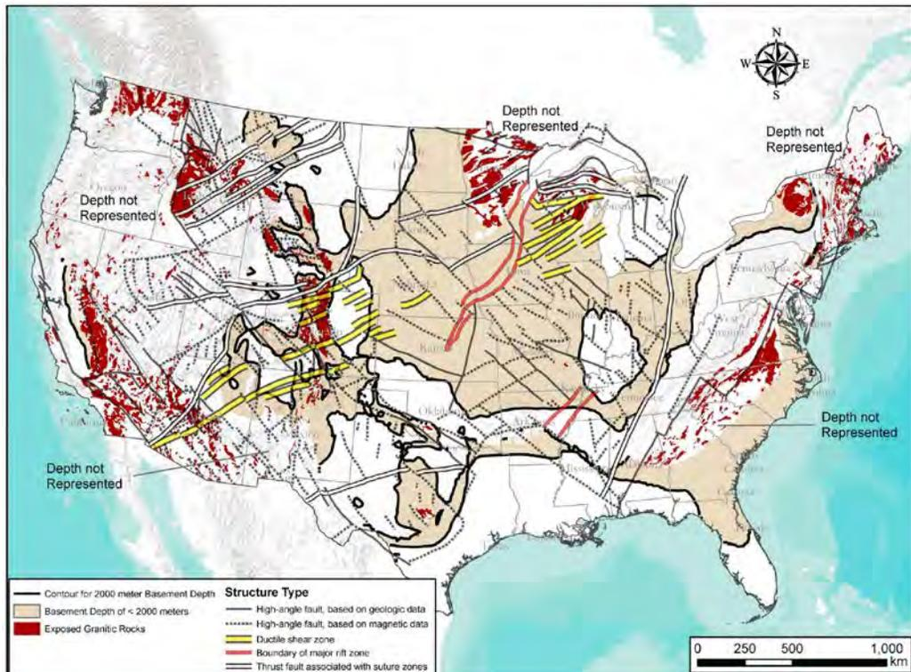
**Figure 6-17.** Crystalline basement at a depth of less than 2000 meters in the contiguous US displayed with the type and location of structural features within crystalline basement (structures from Sims et al., 2008).
