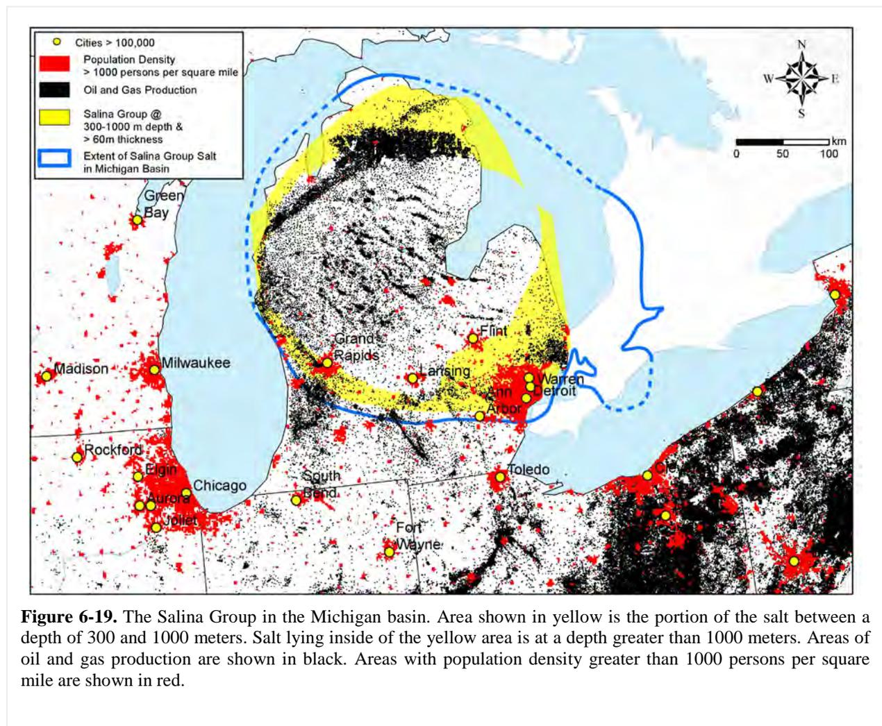
**Figure 6-19.** The Salina Group in the Michigan basin. Area shown in yellow is the portion of the salt between a depth of 300 and 1000 meters. Salt lying inside of the yellow area is at a depth greater than 1000 meters. Areas of oil and gas production are shown in black. Areas with population density greater than 1000 persons per square mile are shown in red.
