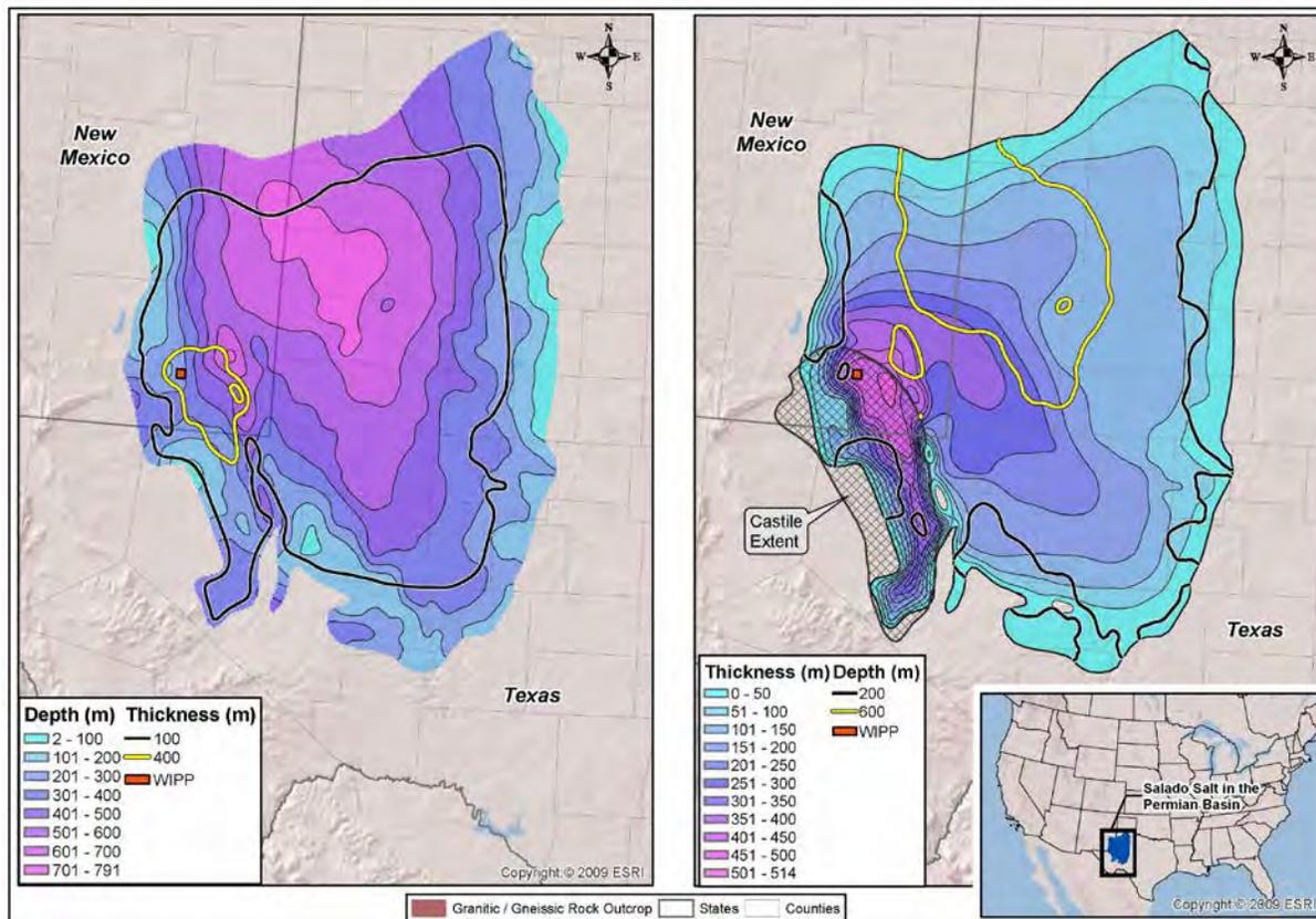
**Figure 4-24.** Depth to top and aggregate thickness of the salt in the Permian Salado Formation in the Delaware, Midland and Palo Duro Basins. Extent of the Castile Formation and the location of the WIPP site (red square) are shown for reference.
