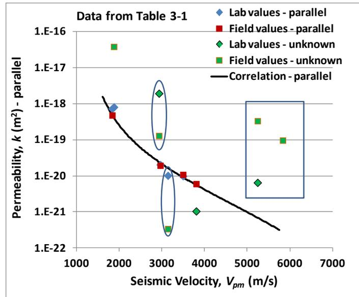
**Figure 5-11.** Permeability correlation parallel to bedding (using Equations 5-2, 5-3, and 5-4 and 5-6) compared with measurements. Note: see text near end of this section concerning ovals and rectangle.
