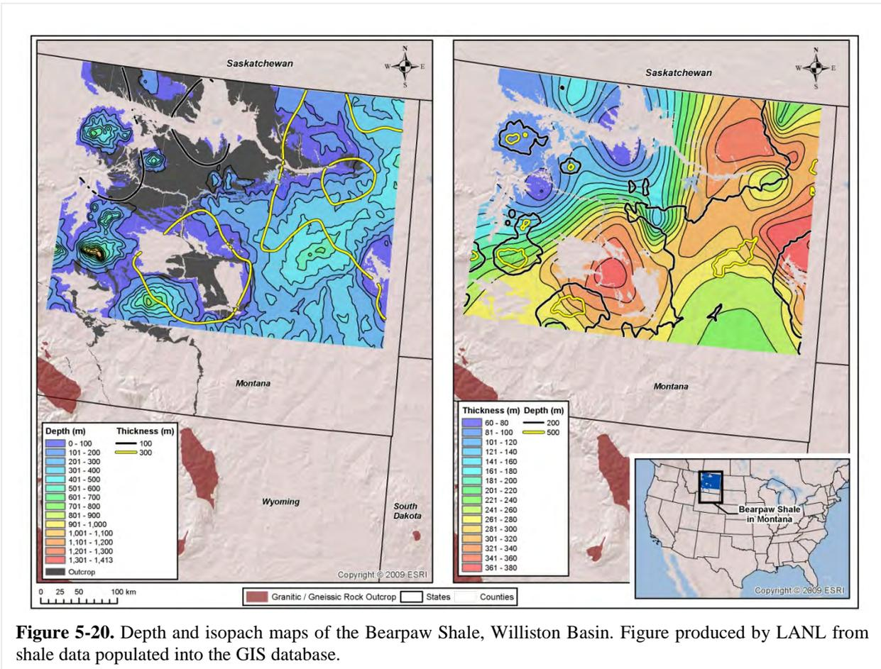
**Figure 5-20.** Depth and isopach maps of the Bearpaw Shale, Williston Basin. Figure produced by LANL from shale data populated into the GIS database.
