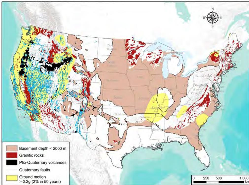
**Figure 6-16.** Location of crystalline basement in the contiguous US at a depth of less than 2000 meters. Included within this classification are exposed crystalline (“granitic”) rocks at the surface. Also shown are the distribution of Quaternary faulting, volcanism, and seismic hazard (yellow shading = 2% probability of exceeding 0.2 g in 50 years), which indicate areas of recent tectonic activity in the US.
