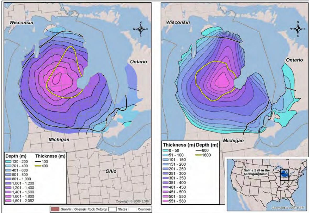
**Figure 4-5.** Depth to top and aggregate thickness of salt of the Salina Group in the Michigan Basin. Salt beneath Great Lakes is not shown. Depth of salt is depth to top of the F Salt, the youngest unit in the Salina Group.
