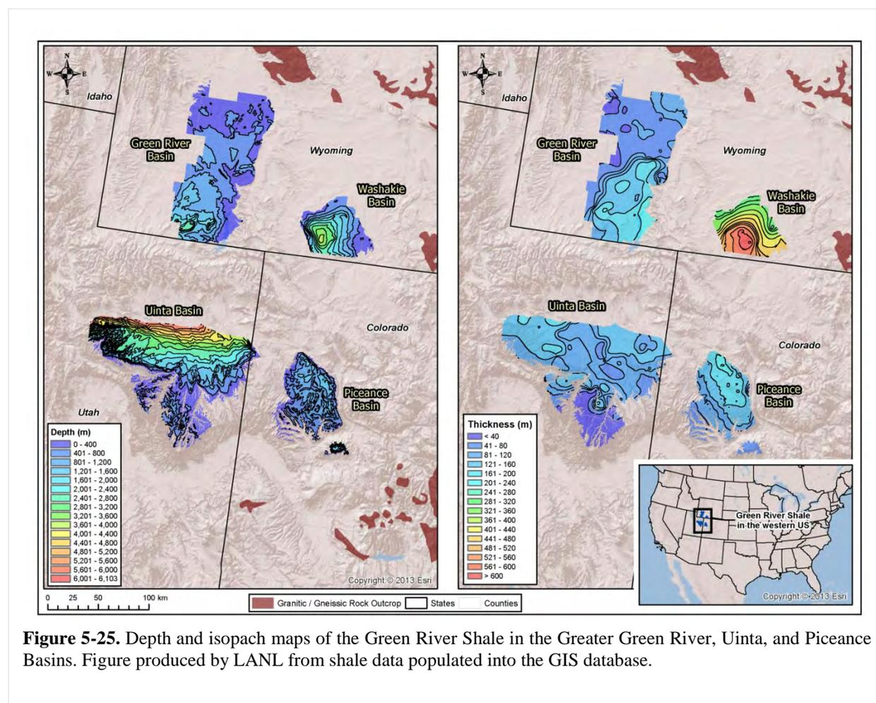
**Figure 5-25.** Depth and isopach maps of the Green River Shale in the Greater Green River, Uinta, and Piceance Basins. Figure produced by LANL from shale data populated into the GIS database.
