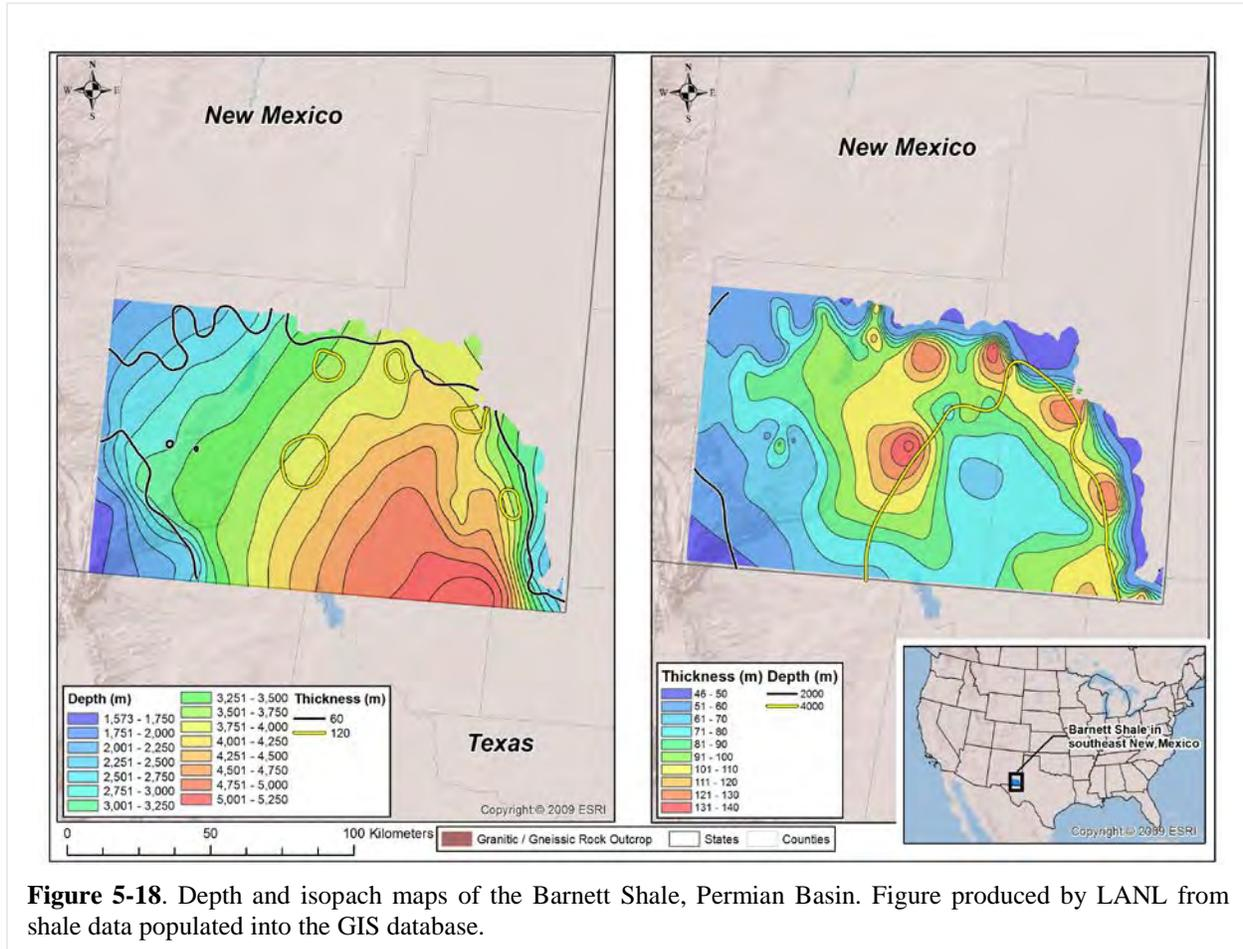
**Figure 5-18.** Depth and isopach maps of the Barnett Shale, Permian Basin. Figure produced by LANL from shale data populated into the GIS database.
