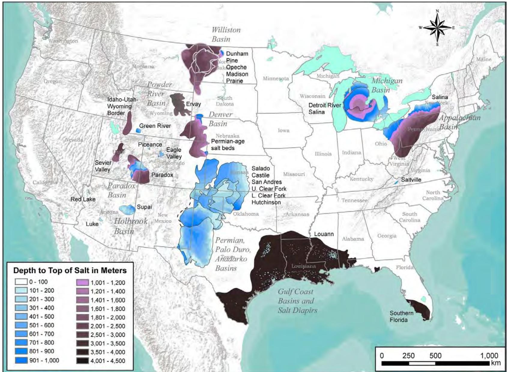
**Figure 4-2.** Distribution and depth to top of salt formations in major sedimentary basins of the U.S. White to blue shading indicates salt at depth of less than 1000 meters. Light to dark purple shading indicates salt at depth of greater than 1000 meters to as deep as 4500 meters. Salt formations are labeled by name or by common reference and listed in stratigraphic order where more than one salt formation is present in a basin.
