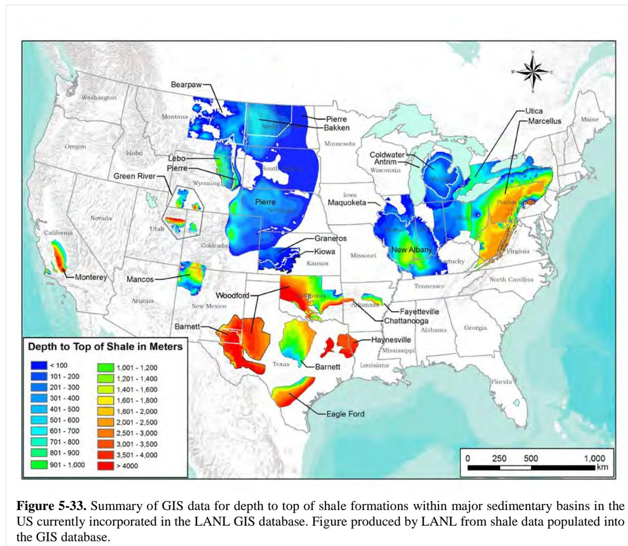
**Figure 5-33.** Summary of GIS data for depth to top of shale formations within major sedimentary basins in the US currently incorporated in the LANL GIS database. Figure produced by LANL from shale data populated into the GIS database.
