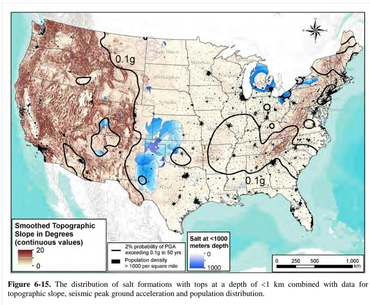
**Figure 6-15.** The distribution of salt formations with tops at a depth of <1 km combined with data for topographic slope, seismic peak ground acceleration and population distribution.
