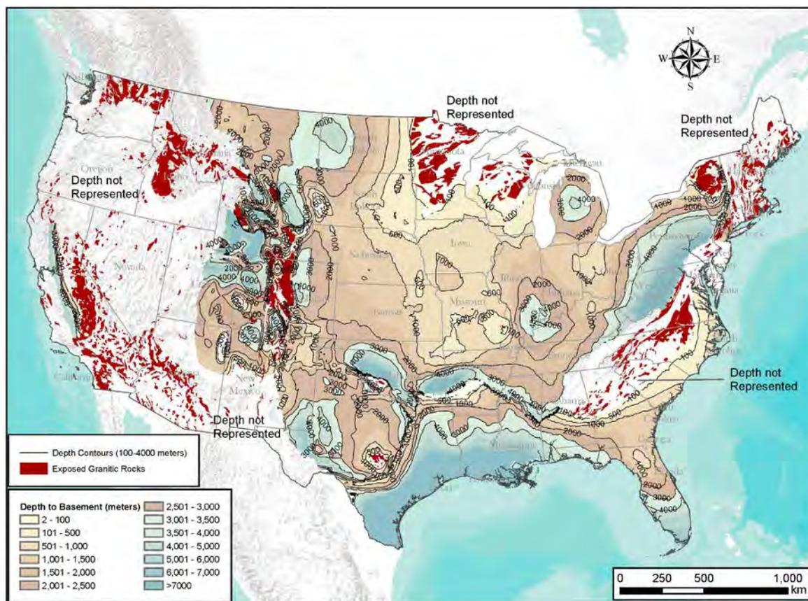
**Figure 6-9.** Depth to crystalline basement and distribution of granitic outcrop (red). Color-shading represents the depth to basement with yellow-brown representing depths of up to 3 kilometers and greens representing major basin areas with basement depth of greater than 3 kilometers.
