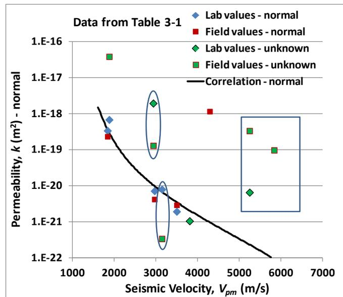
**Figure 5-10.** Permeability correlation normal to bedding (using Equations 5-2, 5-4, and 5-5) compared with measurements. Note: see text near end of this section concerning ovals and rectangle.
