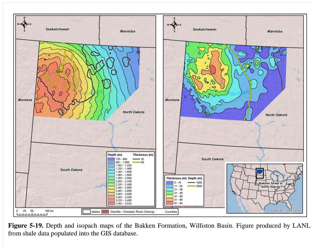
**Figure 5-19.** Depth and isopach maps of the Bakken Formation, Williston Basin. Figure produced by LANL from shale data populated into the GIS database.
