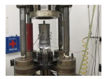
Figure 2-3. Test Apparatus with Reconsolidated Sample.
