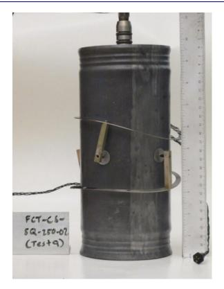
Figure 2-2. Instrumented Specimen Assembly Pretest.
