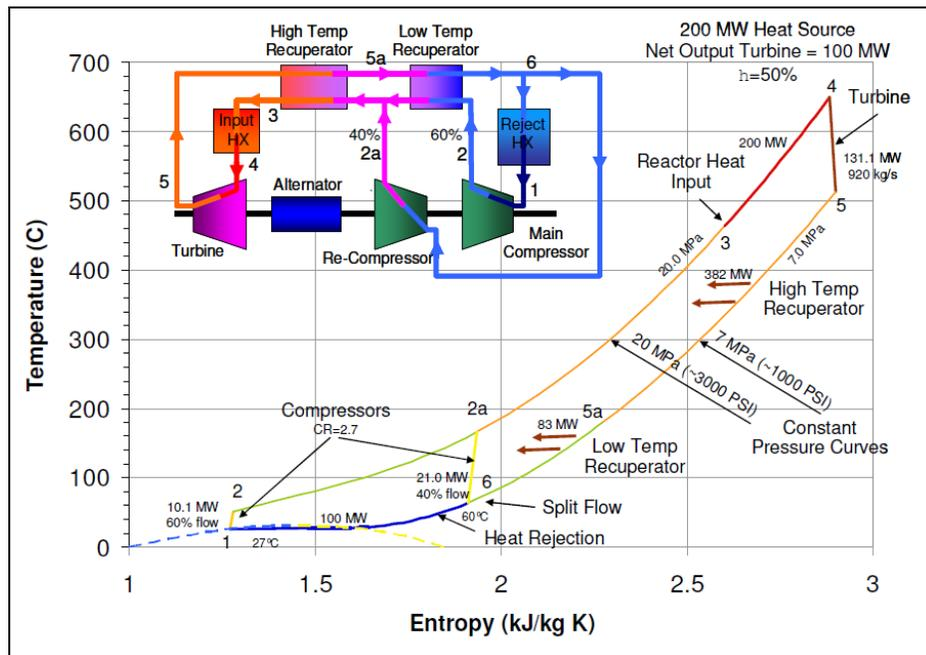
Figure 2. Diagram of SNL's sCO<sub>2</sub> Split Flow Recompression Brayton Cycle [23]
