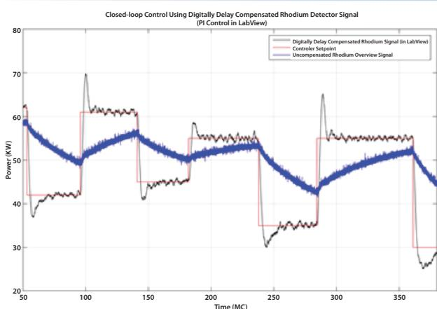
**Figure 5. Closed-loop reactor control using the accelerated Rhodium SPND signal (licensed control system in manual)**
