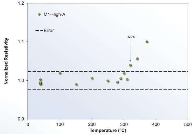
Figure 5. Resistivity data for BR2 M1-High-A.
