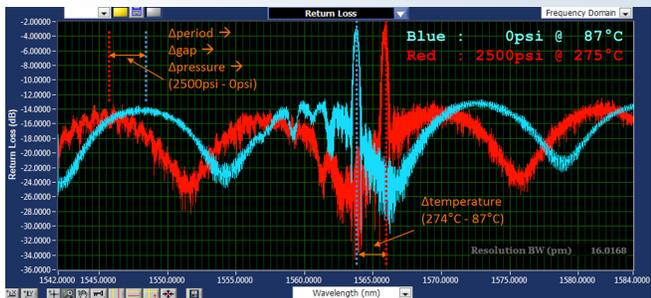
Figure 3. Two Luna OBR 4600 scans of an inline fsFBG and EFPI during pressure tests at Luna’s facility in Blacksburg, Va.
