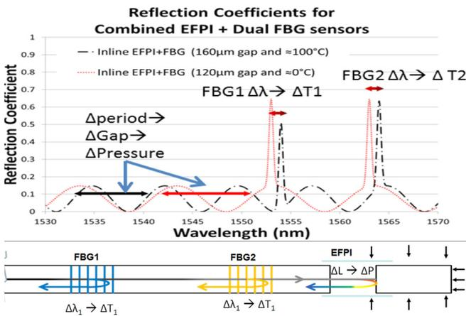
Figure 2. (Left) EFPI, FBG and combined EFPI+FBG sensor response for an EFPI gap of 120 µm and 0°C. (Right) The same sensor at the same conditions and the sensor undergoing a change in pressure that causes the EFPI cavity to transition from 120 µm to 160 µm with a change in temperature of 100°C.
