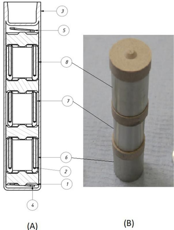
Figure 3. (A) Cross section of the aluminum irradiation capsule (3), stainless steel holders (6, 7, and 8) for SiC monitors (2). The holders are separated with ceramic discs (1) which are held in place with springs (4 and 5). (B) Photograph of the three holders and the three ceramic spacers before irradiation.
