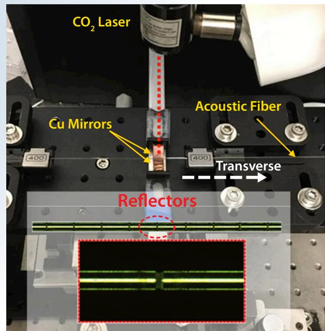
**Figure 3. Acoustic excitation and detection of “suspended core” acoustic fiber and reflection spectrum.**
