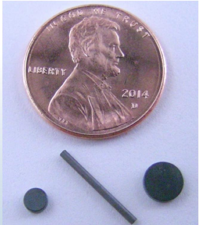
**Figure 1.** SiC temperature monitors available for use in irradiation testing include small rods and disks. Monitors photographed with U.S. penny for size perspective.
