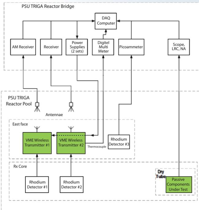
**Figure 2. PSBR test configuration.**
