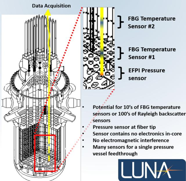
Figure 1. Concept diagram describing planned inline multipoint temperature and endpoint pressure fiber optic sensor.
