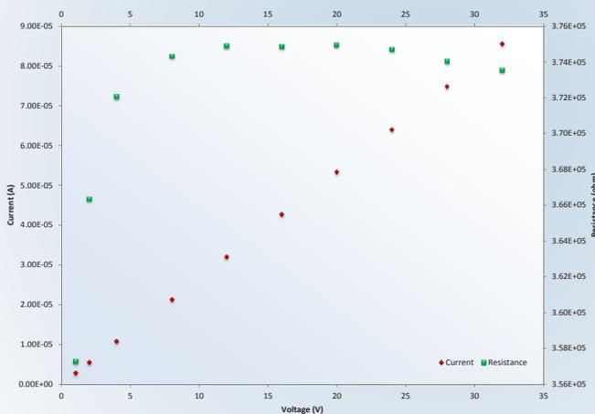
Figure 4. Typical ohmic response as demonstrated by SiC temperature monitor M1-High-A.
