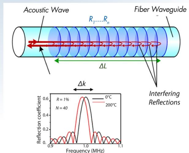
Figure 1. Schematic of AFBGs and temperature response.
