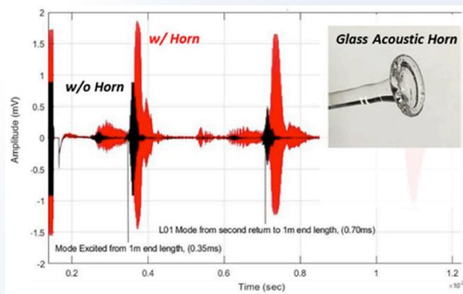
**Figure 3. Acoustic excitation and detection of “suspended core” acoustic fiber and reflection spectrum.**
