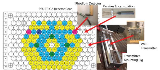
Figure 1. PSBR core hardware location.
