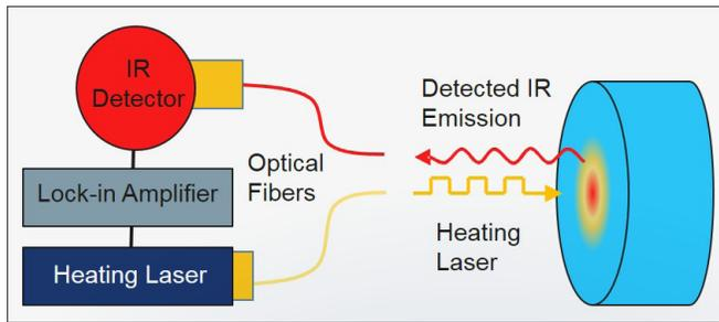
**Figure 3. Photothermal radiometry used to measure thermal diffusivity of nuclear fuel.**
