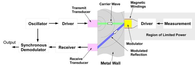
**Figure 5. Transducer reflection topology. One transducer transmits the carrier through the wall media. The ferrofluid transducer modulates the magnitude of the carrier, which is received at the receiving transducer. This signal is demodulated with a lock-in amplifier.**
