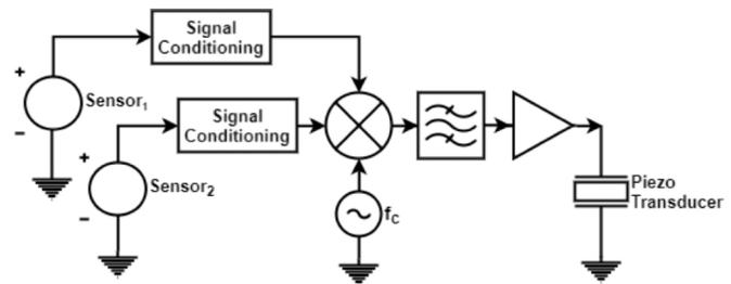
Figure 8. Direct sensor modulation with a carrier waveform of frequency  $f_c$ .
