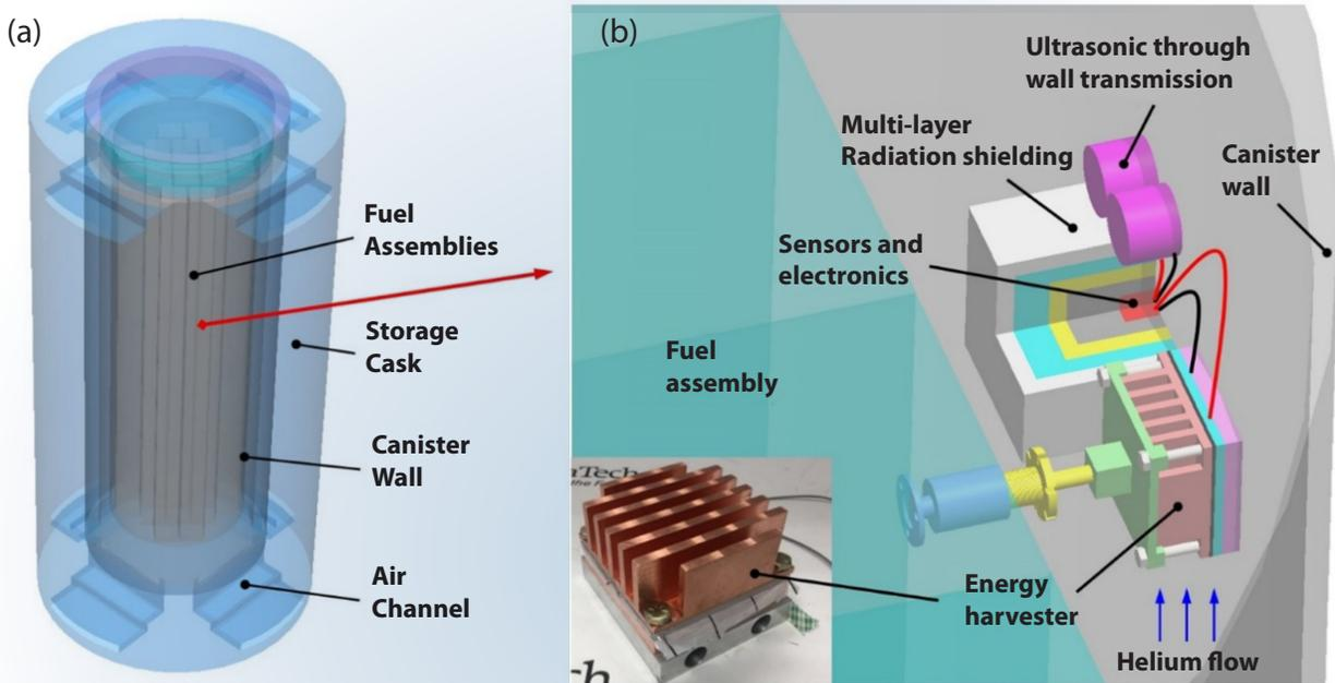
**Figure 1. System illustration of gamma heating thermoelectric energy harvesting and ultrasonic through-wall data communication for enclosed nuclear canisters.**
