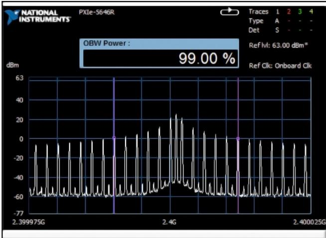
Figure 3. Spectral plot of a pulse-modulated signal.
