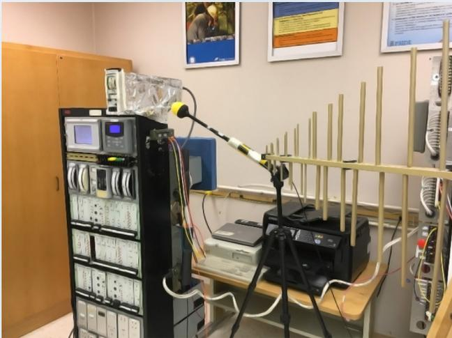
**Figure 5. Test setup for Immunity Testing in a laboratory at Nine Mile Point.**
