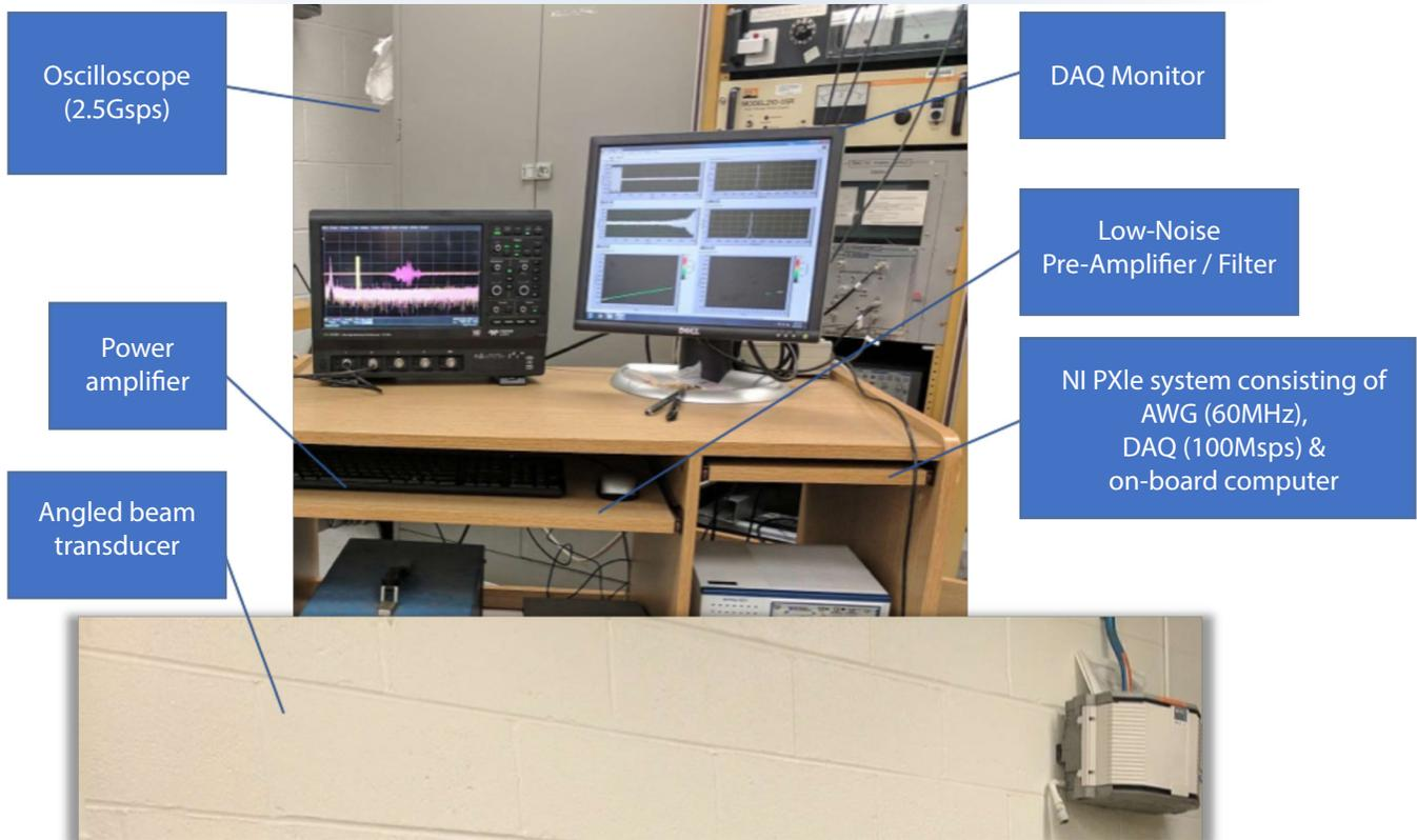
**Figure 1. Benchtop setup showing various components of the acoustic communication system. Displayed at the bottom is the pipe mounted with angled transducers.**
