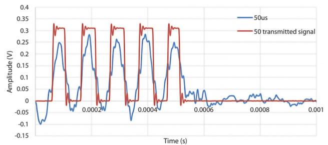
**Figure 2. Transmission and reception of a train of 50- $\mu$ s duration OOK pulses.**
