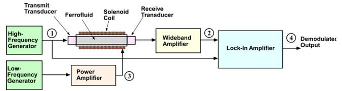
**Figure 4. Block diagram of the through fluid measurement characterization system**
