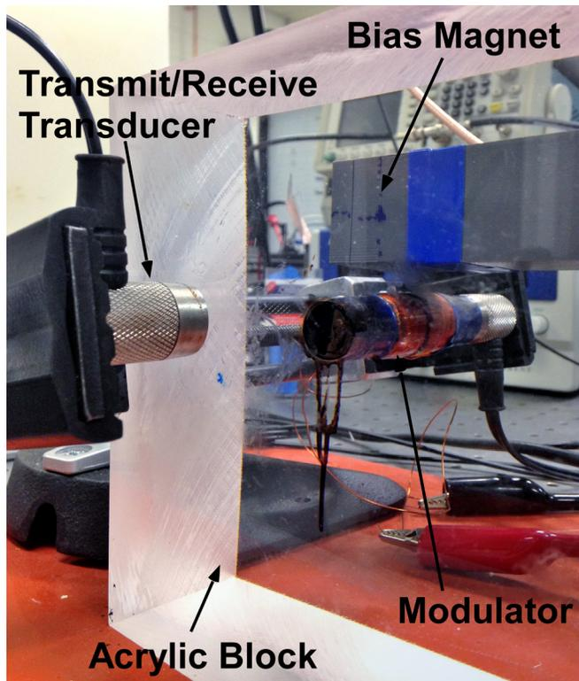
Figure 7. Dual element transducer system tested on the 4-in. acrylic block.
