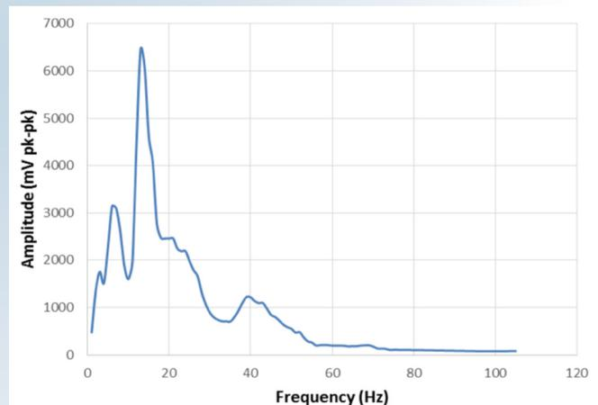
**Figure 6. Ferrofluid magnitude response of through-fluid communication system.**
