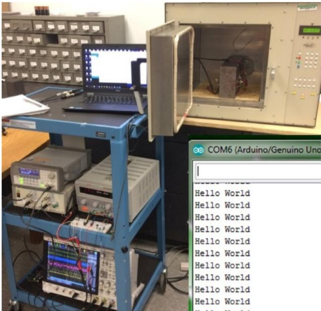
**Figure 3. Photograph of the experiment setup for through-wall communication at 300°C.**
