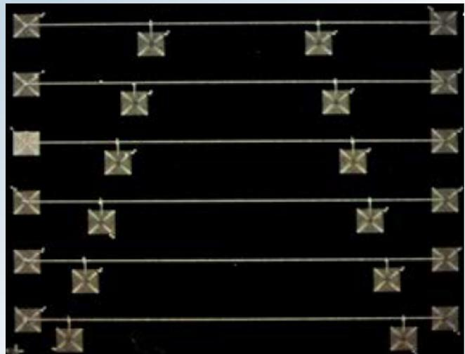
**Figure 2. Passive Temperature Melt Array. Four-point structure of iron printed on titanium coated sapphire (wire to wire distance ~ 1mm).**
