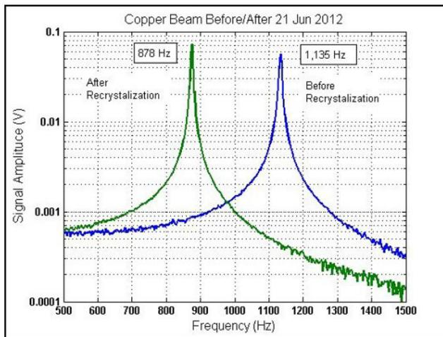
**Figure 4. Laser ultrasonics is used to monitor grain restructuring in cantilever samples made from metallic fuel surrogates.**
