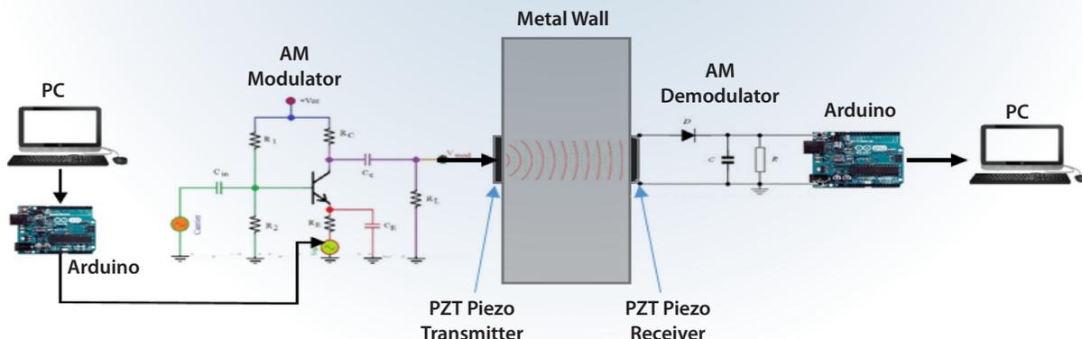
Figure 2. Schematic of ultrasound text transmission system
