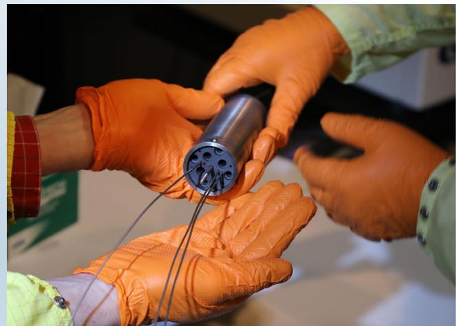
**Figure 2. Photograph of fiber sensors in metal tubes and capsule used at MITR for in-core lead-out testing.**
