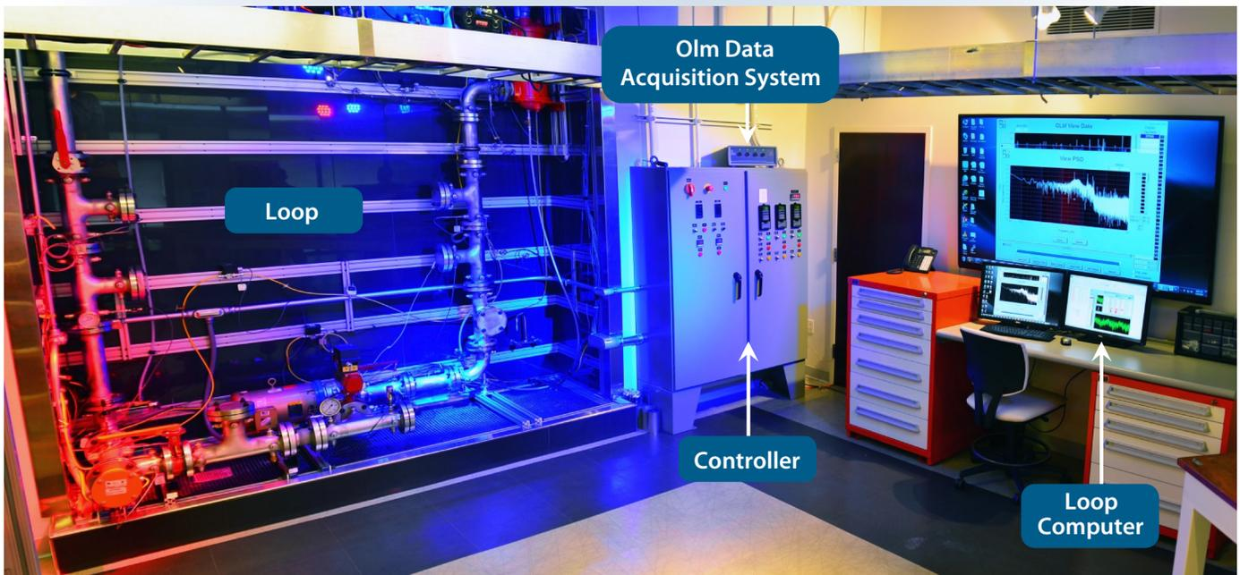
Figure 5. AMS flow loop and test facility.
