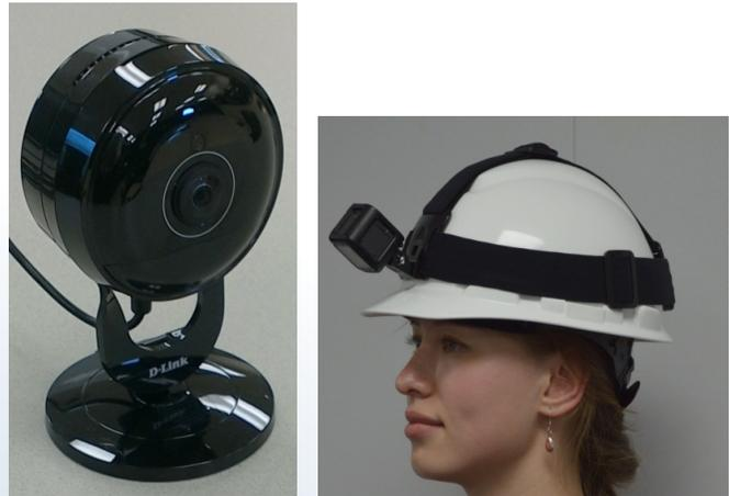
**Figure 12. Fixed (left) and helmet held (right) cameras.**
