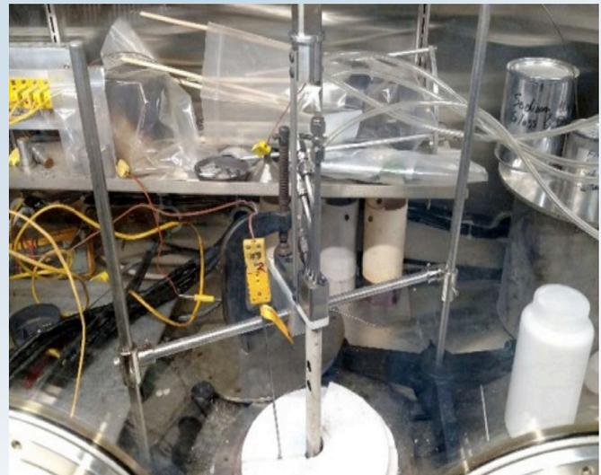
**Figure 6. Photo of the triple bubbler system immersed in molten salt.**
