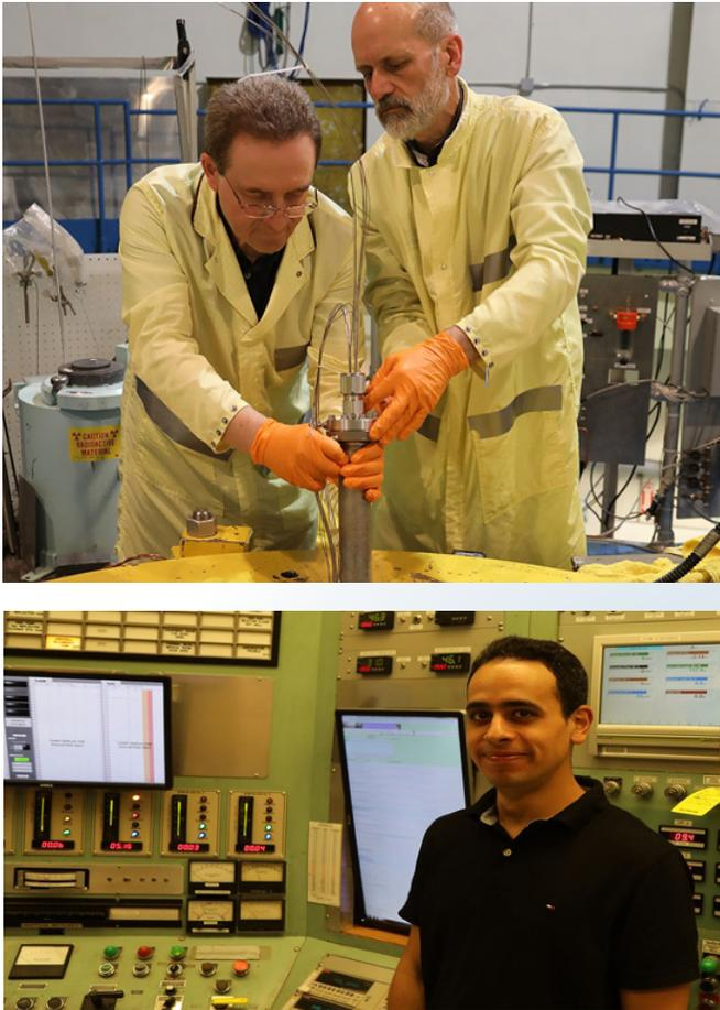
**Figure 3. (a) MIT scientists lower fiber sensor assembly into the reactor core. (b) University of Pittsburgh graduate student Mohamed Zaghoul in the reactor control room for remote monitoring.**
