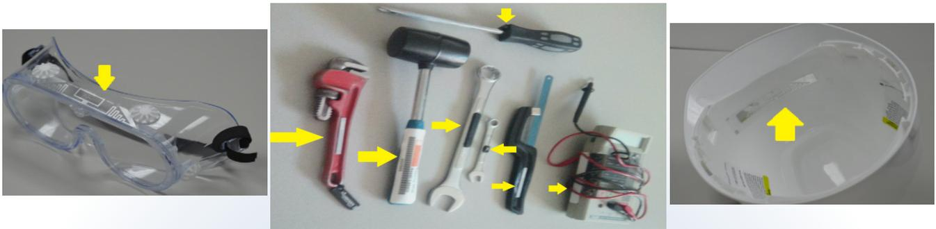
**Figure 6. Example radio frequency identification tags installation on materials, tools, and equipment.**
