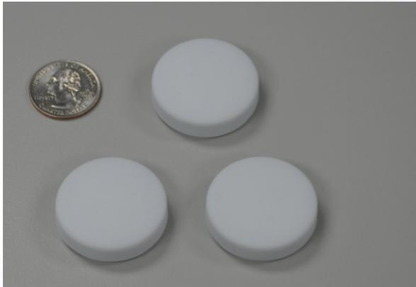
**Figure 8.** Bluetooth low energy beacons used for the pilot study.
