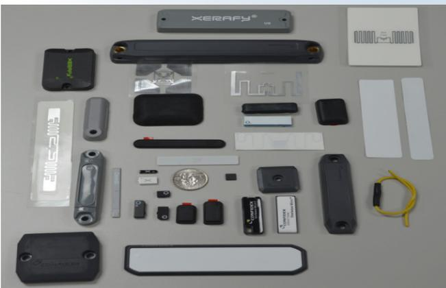
**Figure 4. Sample of radio frequency identification tags of various forms and designs studied.**
