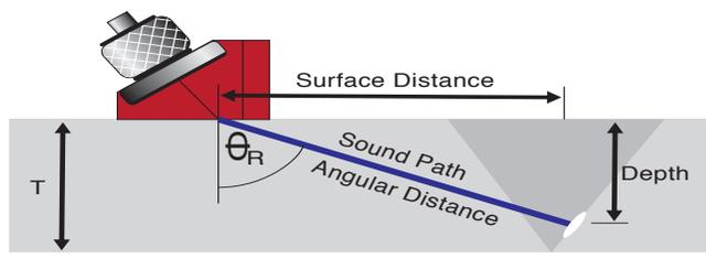
Figure 2. Potted angle beam transducer with a crystal cemented to a plastic wedge with specific angle.
