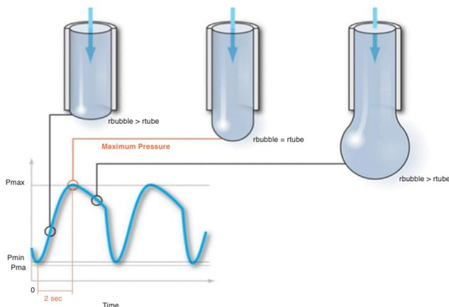
**Figure 3. Illustration of the bubble pressure with respect to its formation and time.**
