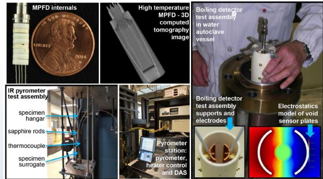
**Figure 4.** Advanced instrumentation development for transient irradiation experiments.
