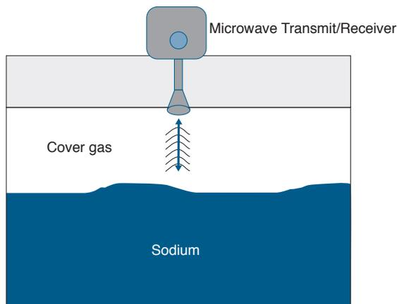
Figure 3. Proposed microwave/millimeter wave level sensor.
