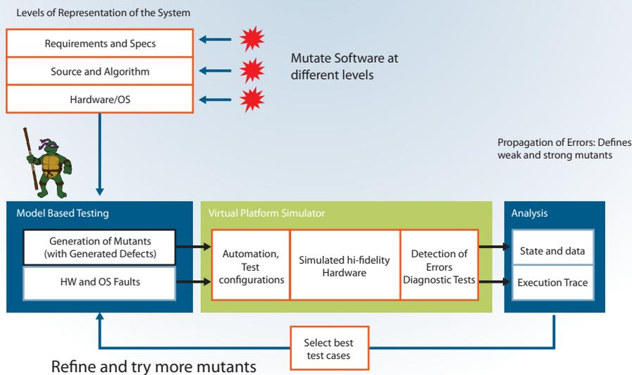
**Figure 1. Virtualized mutation testing: simplified view.**
