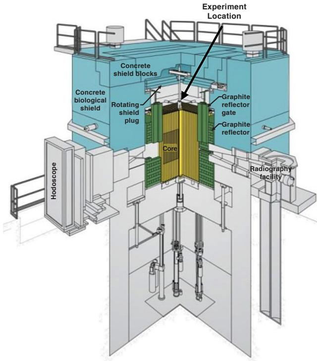
**Figure 1. Cutaway of the TREAT reactor and key facility diagnostics systems. The reactor core is dry allowing for relatively easy instrumentation access through the rotating shield plug and various ports located in the biological shielding.**
