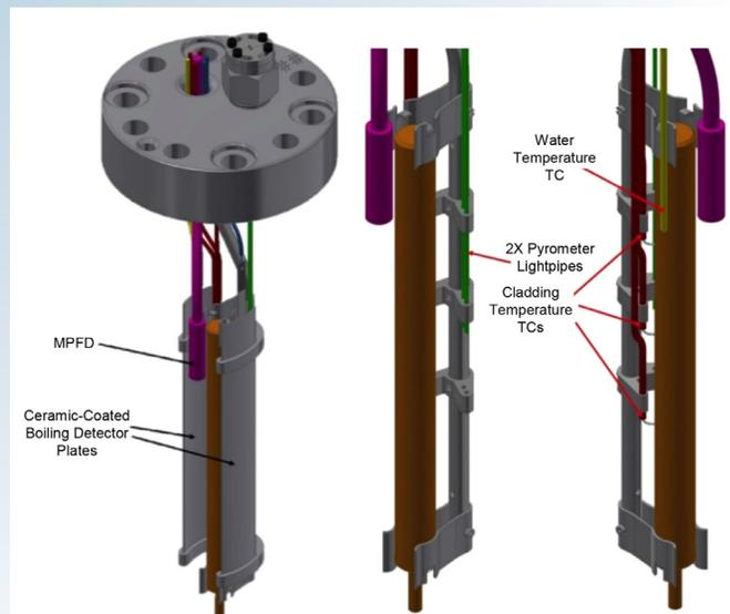
**Figure 3. Instrumentation design for each Multi-SERTTA capsule. (Left) Head unit assembly, (middle) right view of hangar rod showing IR pyrometer light pipes, (Right) left view showing thermocouples.**
