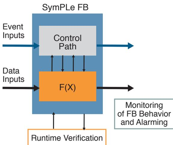
Figure 3. SymPLe Function Block Design.
