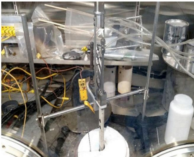
**Figure 6.** Photo of the triple bubbler system immersed in molten salt.
