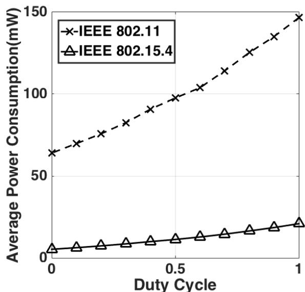
Figure 2. Expected power consumed by a WSN based on IEEE 802.11 and IEEE 802.15.4 communication protocols for different duty cycles.
