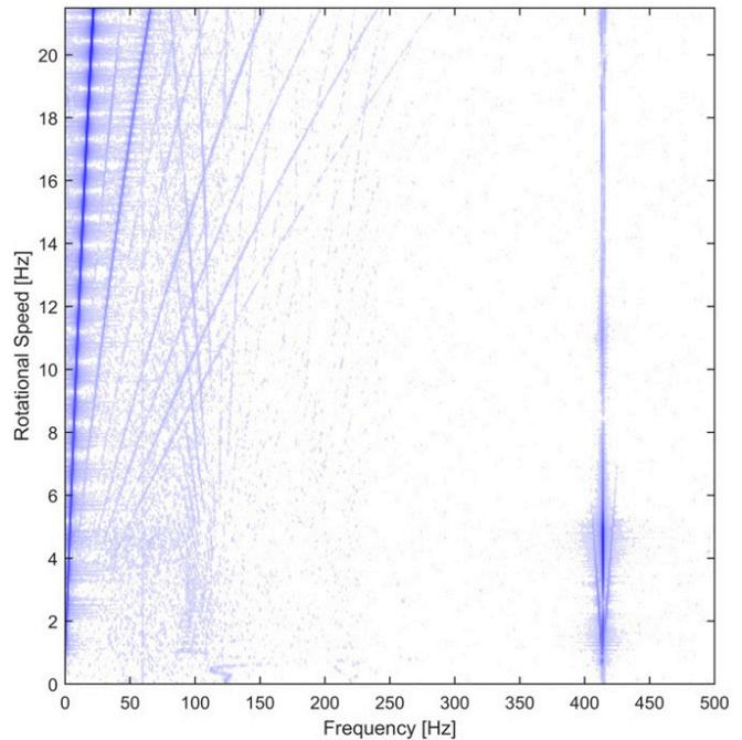
**Figure 6. Waterfall plot of rotordynamics**
