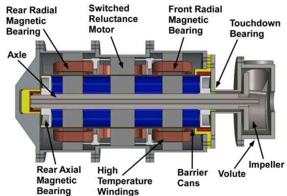
**Figure 2.** Concept drawing of a canned-rotor, magnetically suspended, reluctance drive motor-pump.
