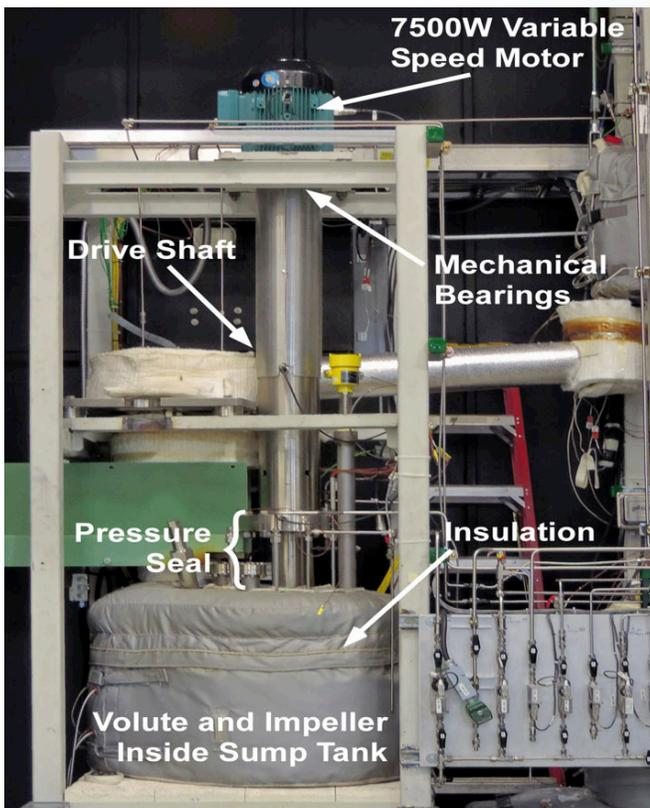
**Figure 1.** Overhung pump used in the ORNL molten salt loop experiment.
