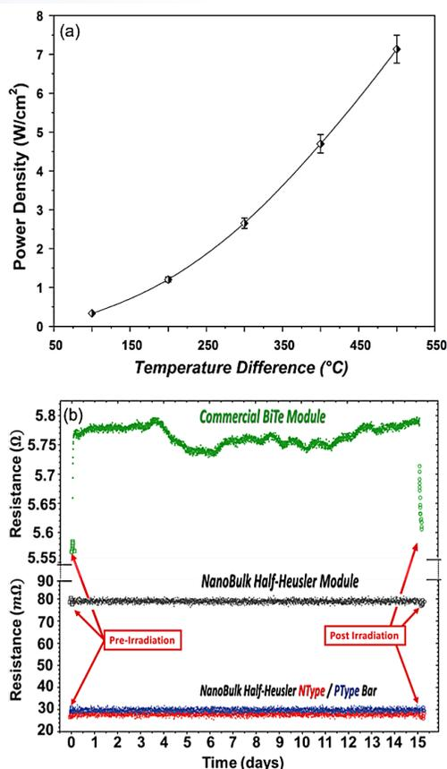
Figure 3. (a) Electric power density versus temperature difference of a nanobulk half-Heusler uncouple device at a constant cold-side temperature of 100°C. (b) Gamma radiation effect on the electric resistances of the nanobulk half-Heusler devices and a commercial BiTe device.
