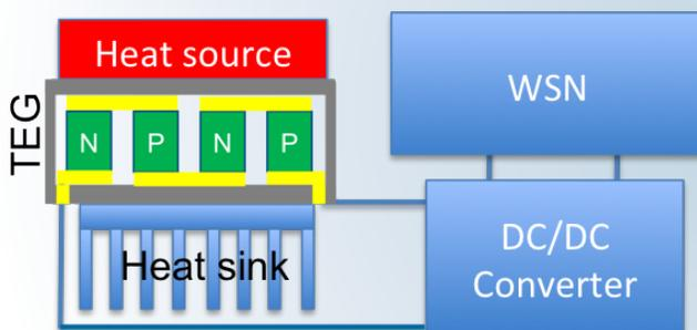
**Figure 1. Schematic of self-powered wireless sensor node (WSN) using thermoelectric generator (TEG).**
