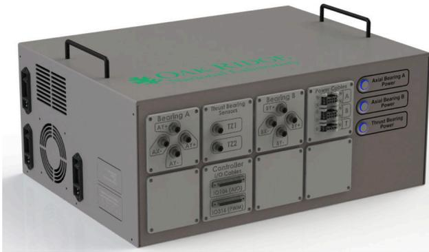
**Figure 4. Custom electronics enclosure for the power electronics and data acquisition.**
