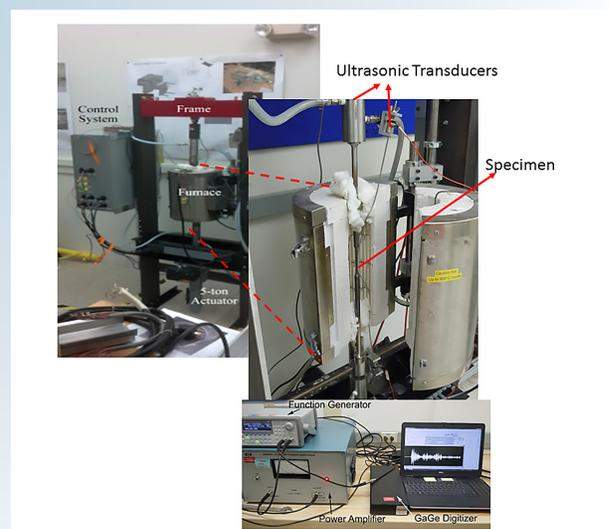
**Figure 1. Accelerated aging test-bed with in-situ online condition monitoring sensors.**
