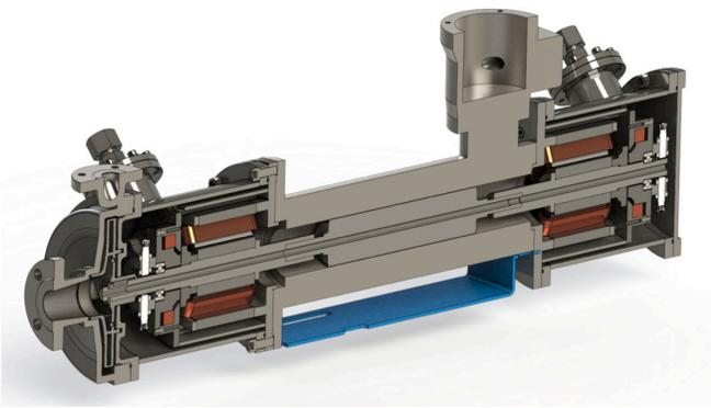
Figure 7. Loop-scale pump testbed final design.
