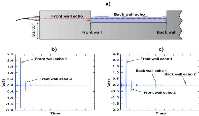
Figure 2. a) Illustration of ultrasonic energy propagating through a stainless steel baseplate and reflecting off of drain sump surfaces (i.e., front wall and back wall). Depiction of signals containing b) features of multiple front wall echo signals for the condition of an empty drain sump and c) features of multiple front wall and back wall echo signals for a drain sump containing water.
