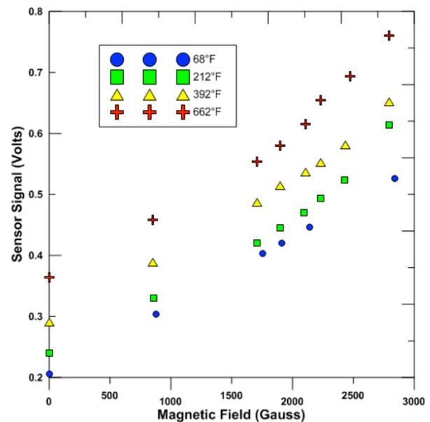
**Figure 2.** Response of Rod Position Sensor at varying temperatures.
