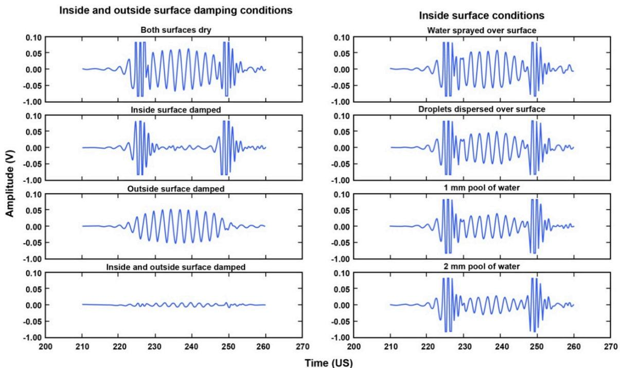
Figure 5. Receiver responses – left series: progressive waveforms for both sides dry, inside (top) surface damped, outside (bottom) surface damped, and both surfaces damped; right series: both sides dry, inside (top) surface droplets, 1 mm, and 2 mm of water on plate top surface.
