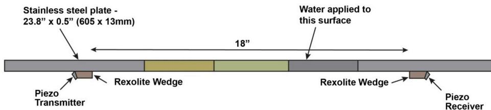
Figure 4. Illustration of experimental set-up used to demonstrate capability to detect small quantities of water on the surface of stainless steel plate opposite to the surface that transducers are mounted.
