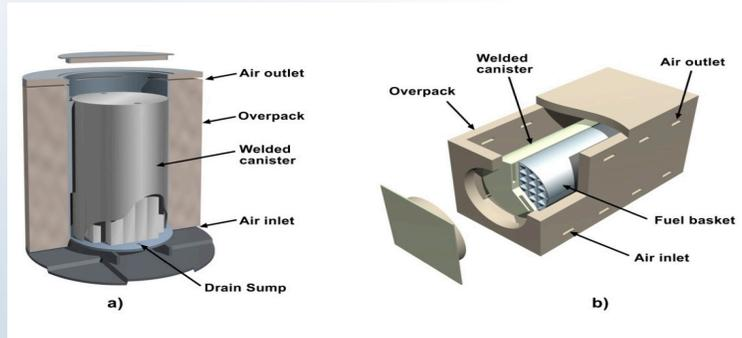
**Figure 1. Illustrations of generalized dry storage systems consisting of a welded stainless steel canister and concrete overpack. Two types of systems are distinguished by orientation of the canister a) vertically and b) horizontally.**
