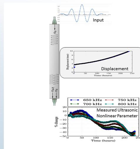
**Figure 2. Example of nonlinear ultrasonic parameter measured as a function of time as specimen was subjected to high-temperature creep. The graphic also shows the arrangement of the transducers for applying the excitation and recording the response.**
