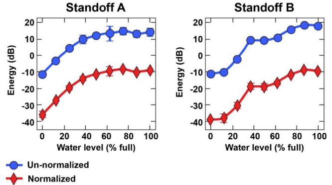
Figure 3. The back wall echo signal energy as a function of the water level in the sump at two different standoffs near the top of the drain sump. Results for back wall echo signal normalized to front wall echo signal are provided (red) along with the signal with no normalization (blue).
