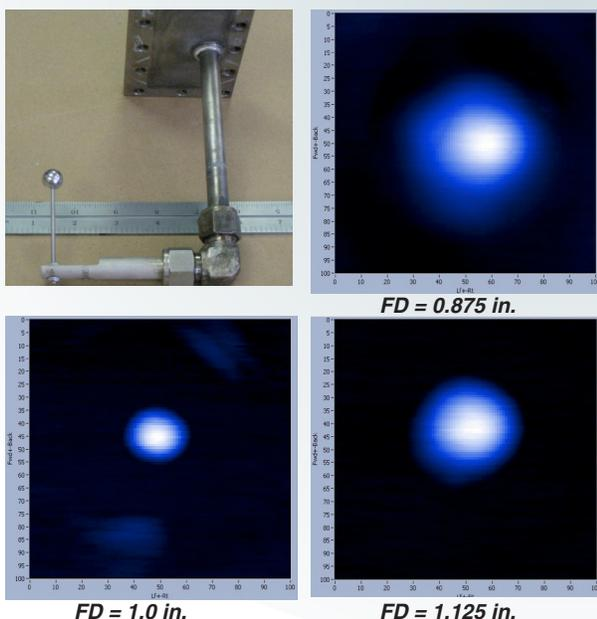
**Figure 10. Ball-bearing target sample and beam diameter.**
