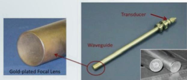
Figure 1. A UWT Prototype with a 1 in. focal lens.
