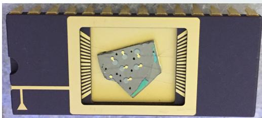
**Figure 1. Photograph of several detectors fabricated on a GaN wafer, mounted in a standard dual in line package for testing.**
