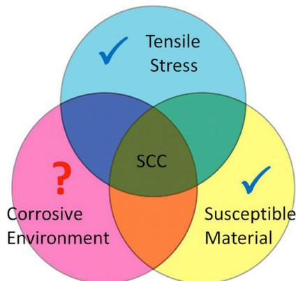
**Figure 5. Relationship between stress, material susceptibility, and environment. Some welded stainless steel UNF canisters may meet two-thirds of the requirements needed for CISCC to initiate. Residual tensile stress from welding the plates is present, and the stainless steel materials used are susceptible to CISCC. What is not well understood is if any canisters are in corrosive environments that could potentially lead to SCC.**
