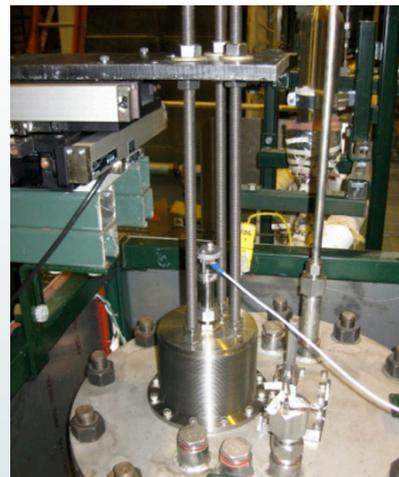
**Figure 4.** Experimental setup with a bellows mounting assembly of a UWT.
