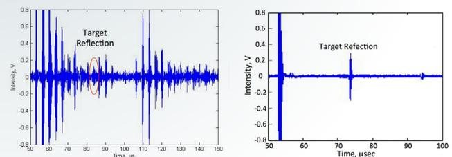
Figure 2. Ultrasonic radio frequency signals received from a smooth waveguide (left) and a UWT prototype (right) in water.
