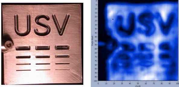
**Figure 5.** USV target sample and intensity image of the target sample at 177°C and FD = 19.05 mm.
