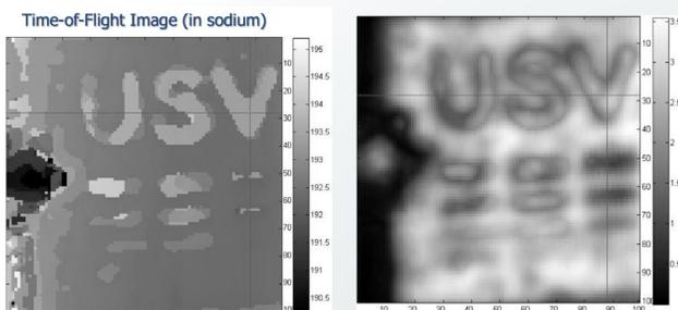
**Figure 6.** TOF (left) and intensity (right) images of the USV target sample at 177°C and FD = 25.4 mm.
