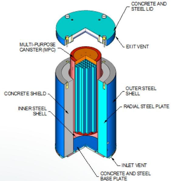
**Figure 3. A cutaway illustration of the Holtec International, Inc. Hi-Storm 100 storage system. Once installed on a storage pad, these systems provide radiation shielding protection for the UNF and a barrier against intrusion.**
