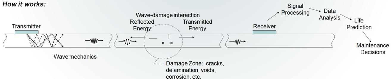
Diagram shows the through-transmission method; the pulse-echo method is similar but based on reflected energy.
