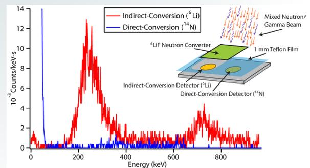
**Figure 2. Spectra obtained from GaN detector using Li-6 indirect-conversion material (red) and direct-conversion material of neutrons from N-14 (blue). Inset is a schematic of the experiment setup.**
