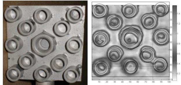
**Figure 7.** Fuel-pin target sample and intensity image of the target sample at 177°C and FD = 25.4 mm.
