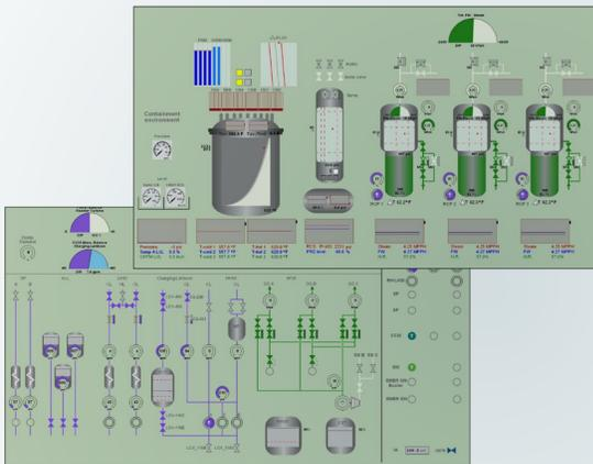
**Figure 4. Advanced overview displays to aid operator monitoring and troubleshooting.**
