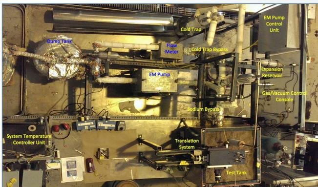
**Figure 3.** USV test facility.
