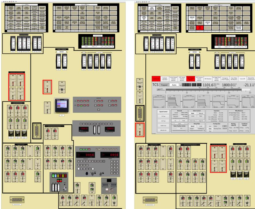
Figure 3. Example of legacy turbine control system computer (left) updated with a turbine HSI (right) on the glasstop panels of the Human Systems Simulation Laboratory.
