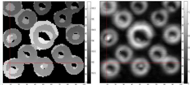
**Figure 8.** TOF (left) and intensity (right) images of the fuel-pin target sample at 177°C and FD = 25.4 mm.
