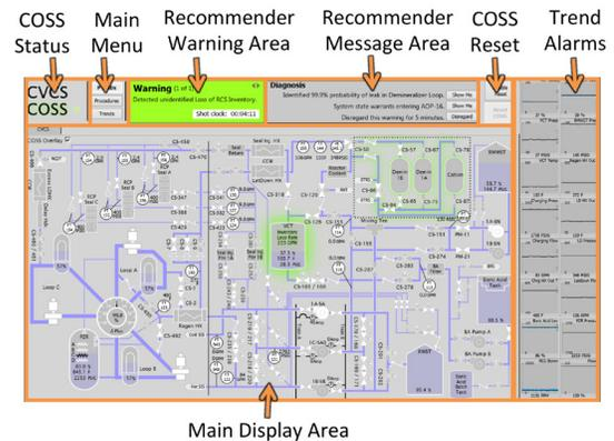
**Figure 5. Annotated COSS display featuring areas of concern, a recommender warning, and suggested mitigation action messages.**
