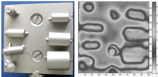
**Figure 9. Joyo-pin target sample and intensity image of the target sample at 177°C and FD = 25.4 mm.**
