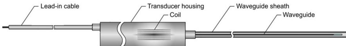
**Figure 1. Schematic of typical ultrasonic thermometer.**
