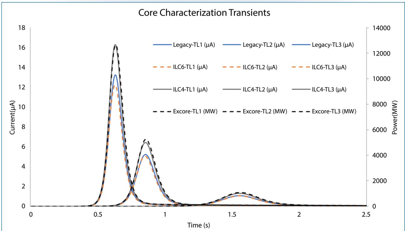
Figure 1. SPND signal trace comparison overlay with reactor power for three different pulse transients of varying peak power.
