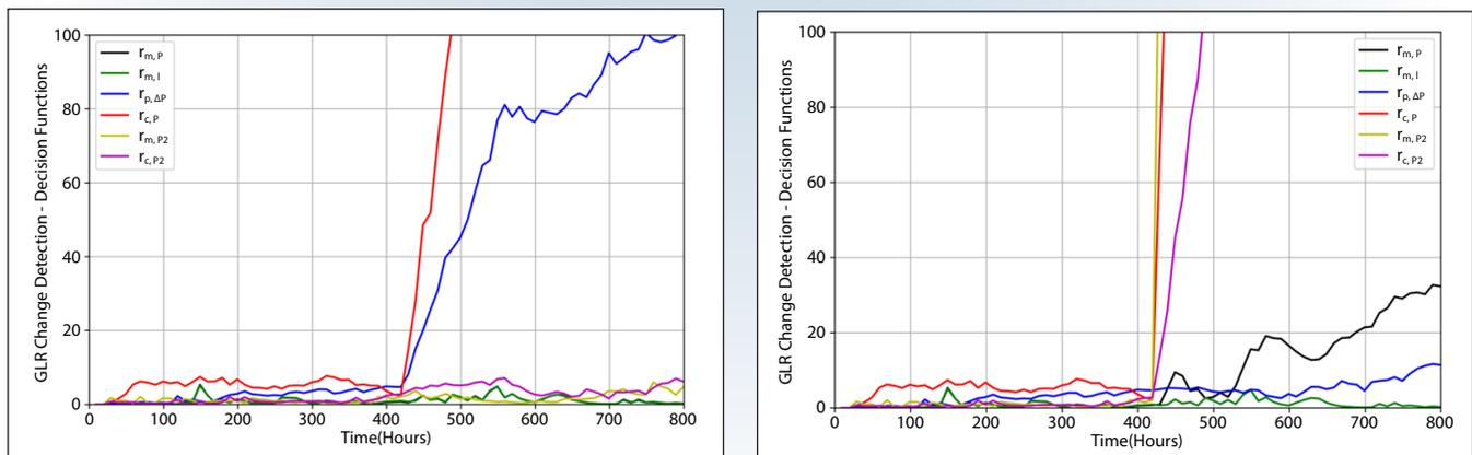
Figure 4. Successfully diagnosed feedwater flowrate (left) and motor power (right) sensor bias errors.
