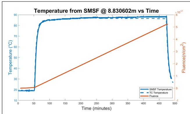
**Figure 4.** SMSF determined temperature as a function of time irradiated along with collocated thermocouple measurement.
