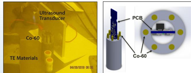
**Figure 4. Gamma radiation test in hot cell at Westinghouse.**
