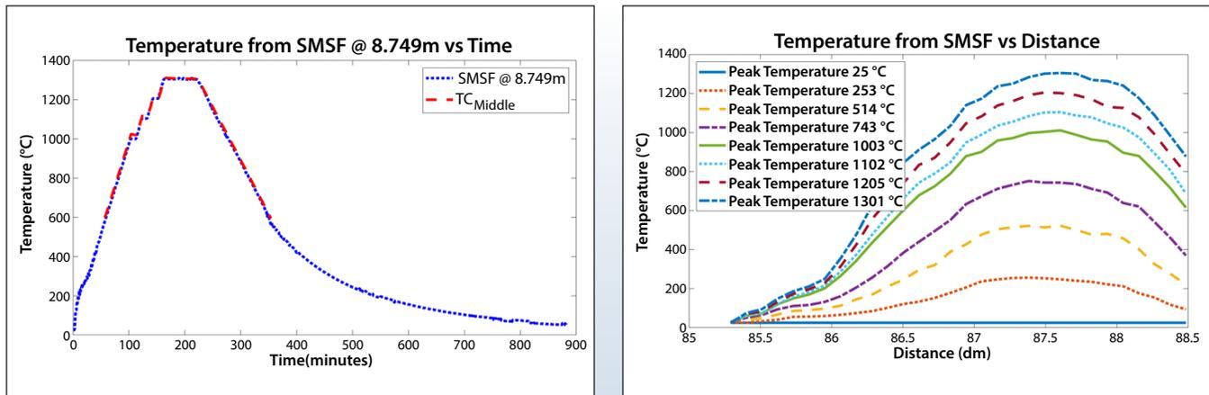
**Figure 3.** (Left) Temperature determined from spectral shift by a third order fit during descending temperature shift measured by Luna's OBR 4600 versus time at the point of peak furnace temperature is shown in blue. The dotted yellow line is the reading of a type-B thermocouple co-located at this point. (Right) Furnace temperature as a function of distance during several times as determined by the SMSF measurements. There are 30 gauges shown along this length of fiber.
