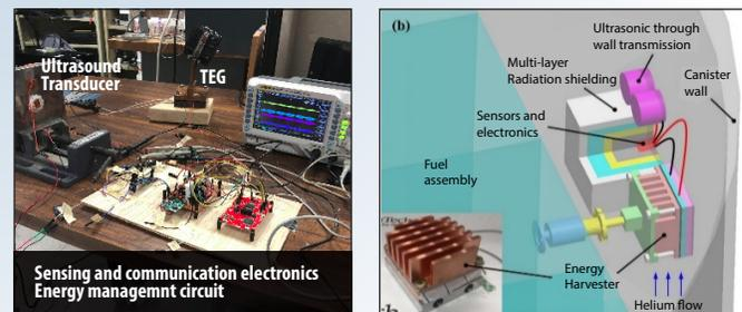
**Figure 1. The prototype system of the self-powered ultrasound data communication and sensing (upper-left) and illustration of its installation in the nuclear canisters (lower-right).**
