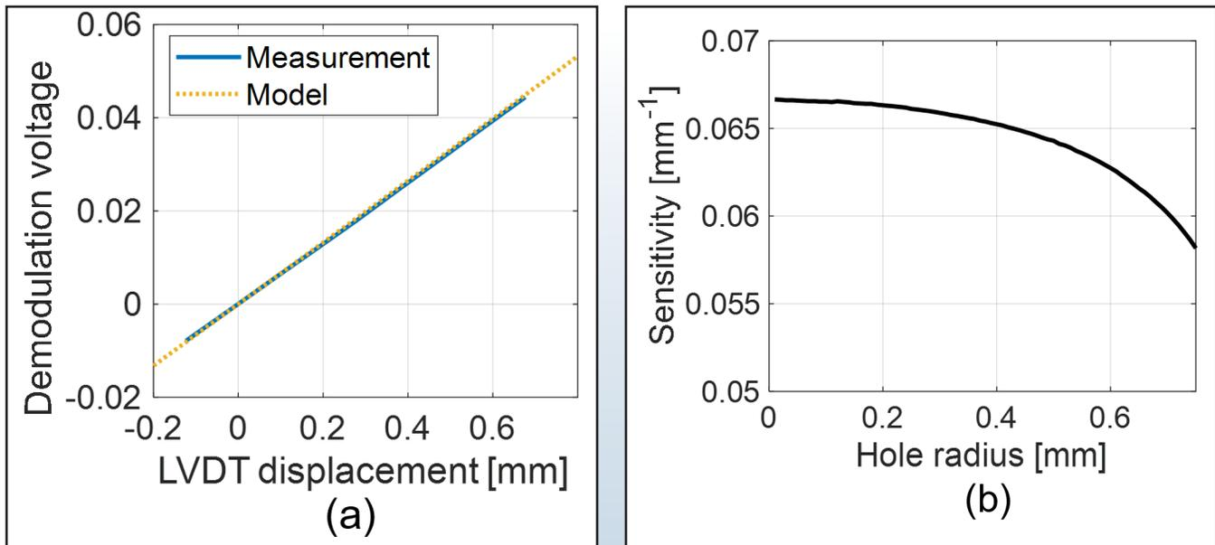
Figure 4 (a) Comparison of modeled and measured sensor performance. (b) LVDT sensitivity versus central hole radius.
