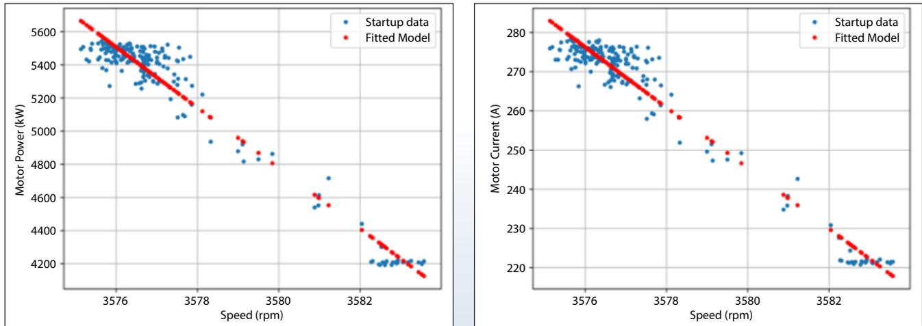
Figure 3. Calibration of motor input power model (left) and motor current model (right).
