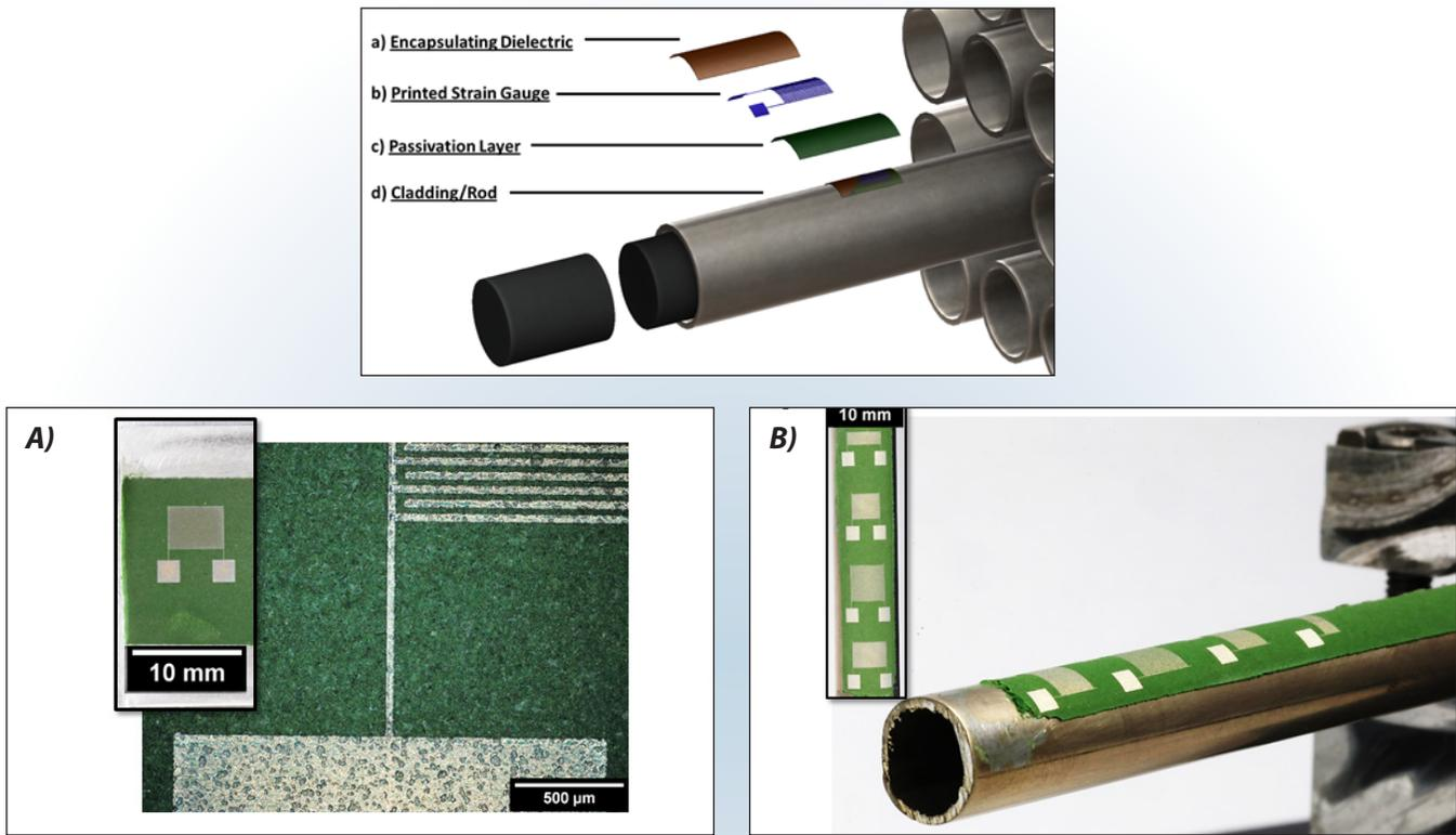
**Figure 1.** Schematic of AM strain gauge on fuel pin. (A) Close up of the aerosol jet printed capacitive strain gauge (AJP-CSG) and (B) the AJP CSG on a 9.5-mm-diameter fuel pin with an insulation layer.
