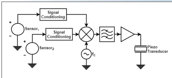
**Figure 3. Direct sensor modulation with a carrier waveform of frequency  $f_c$ .**
