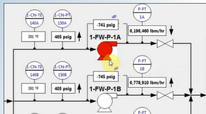
Figure 2. Process and instrument diagram for feedwater pump system.
