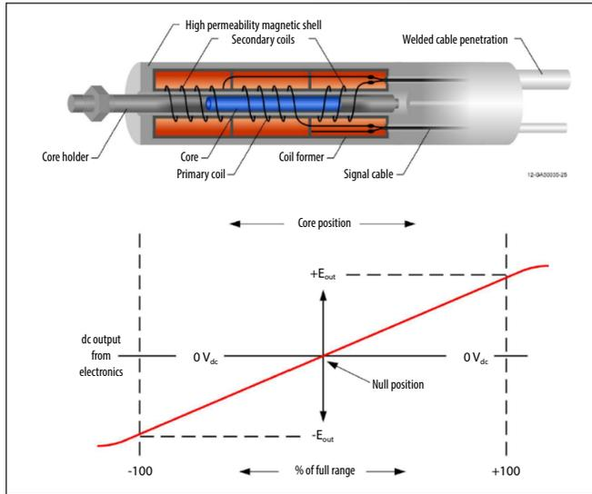
Figure 1. Cross section of basic LVDT design and displacement/electrical output curve.
