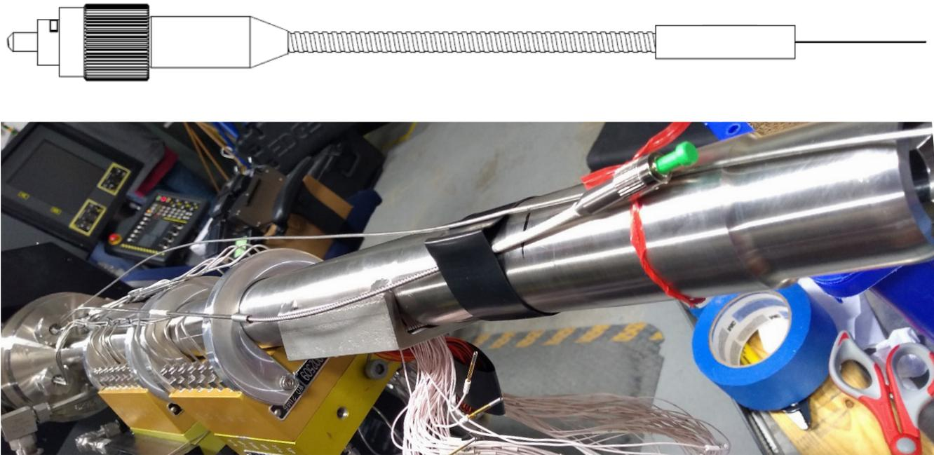
**Figure 2. Top: Schematic of optical fiber sensor. Bottom: One of the FBG sensors installed in the HDG-1 experiment.**
