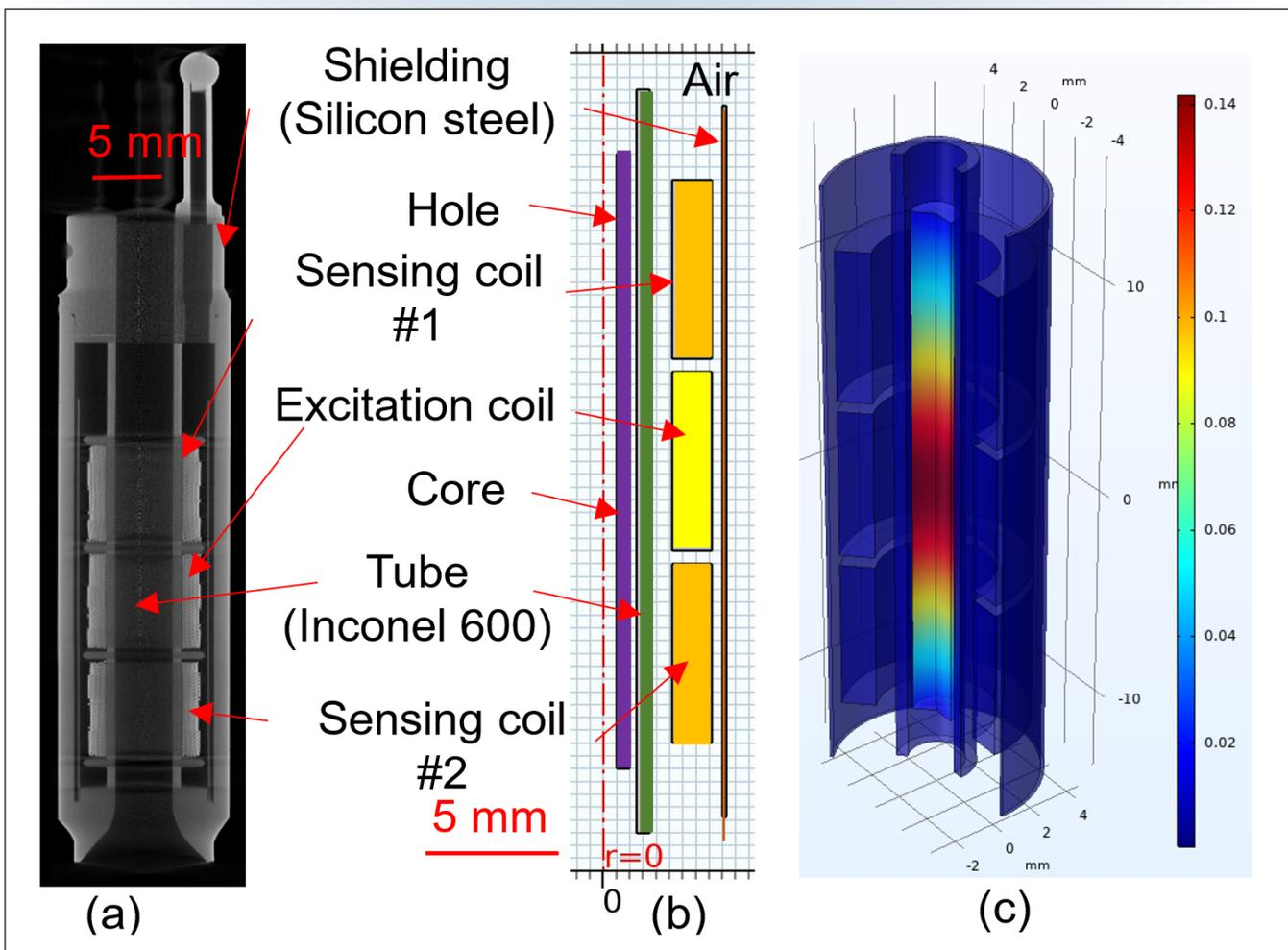
Figure 3 (a) A CT image showing the cross section of an IFE LVDT sensor. (b) 2D axisymmetric model configuration in COMSOL Multiphysics. (c) Magnitude of magnetic flux density in Tesla when the core is 1 mm away from the null position.
