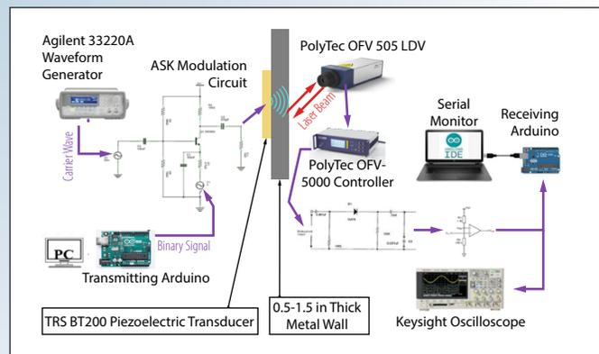
**Figure 2. Schematic of ultrasound text transmission.**
