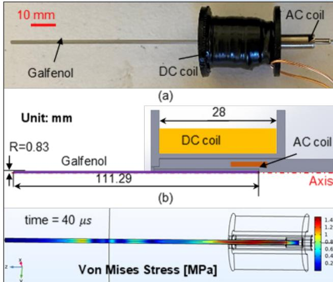
**Figure 3.** (a) Physical assembly of the pulse-echo mode ultrasonic thermometer with an additional DC bias coil. (b) 2D axisymmetric model layout in COMSOL Multiphysics. (c) Simulated compressive wave propagating in the Galfenol wire ( $40\ \mu\text{s}$  after excitation).
