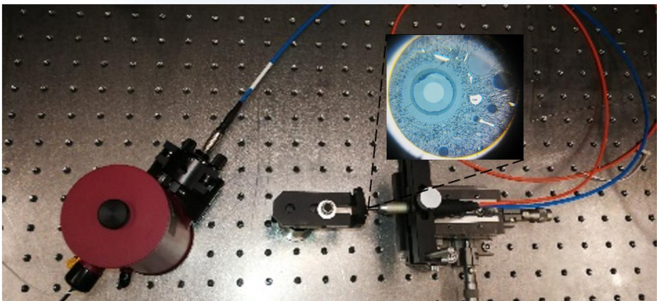
**Figure 1.** Proof of concept system using a fiber-optic to collect black body irradiation associated with transient laser heating. The inset shows an optical micrograph of the fiber end facing the sample.
