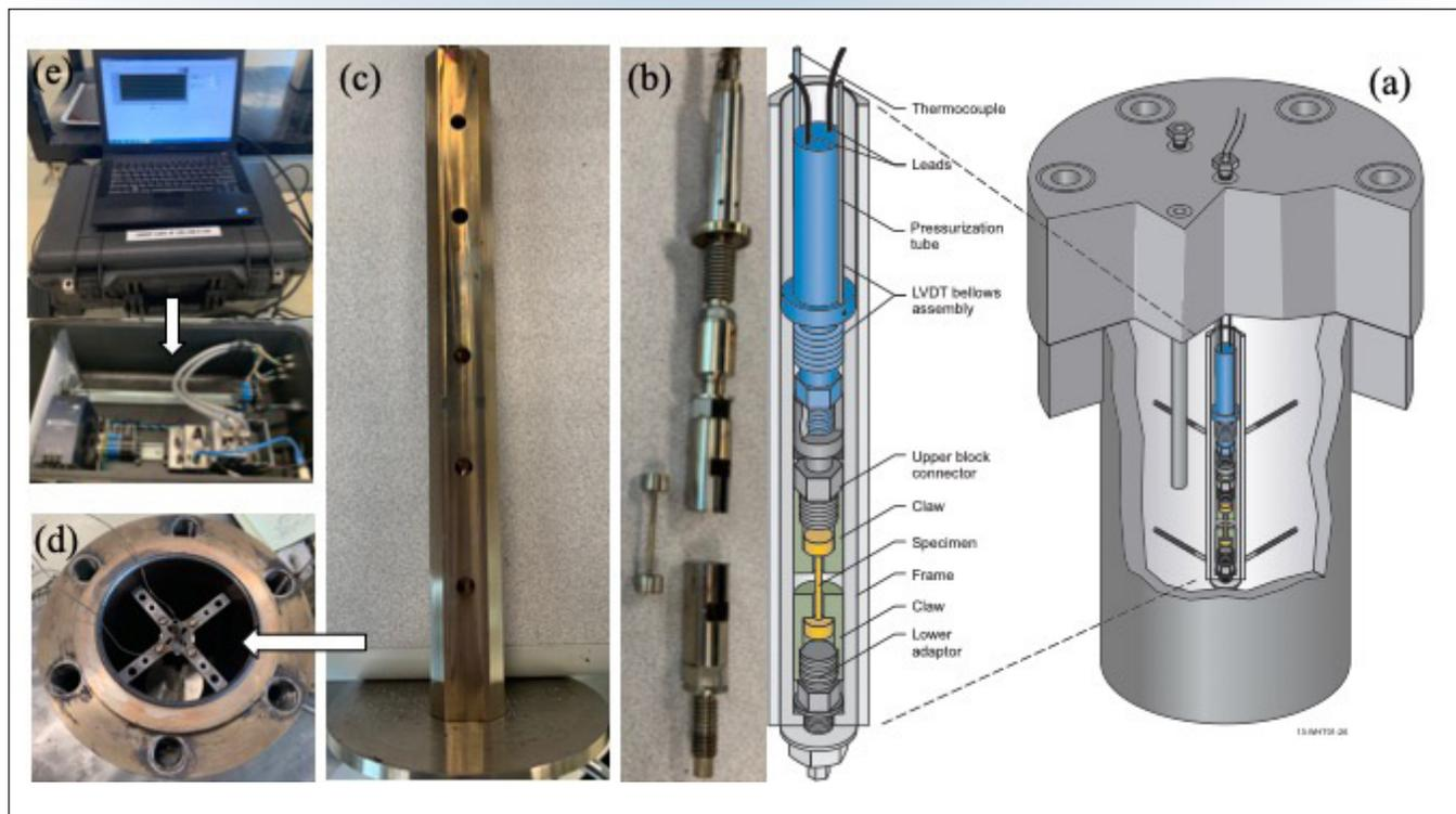
**Figure 1 – (a) schematic of the Creep Test Rig inside autoclave, (b) actual parts of the Creep Test Rig with SS 304 sample, (c) Creep Test Rig all together and ready for testing, (d) Creep Test Rig positioned in static autoclave, (e) NI data acquisition system for recording TC and LVDT signals. [3,5].**
