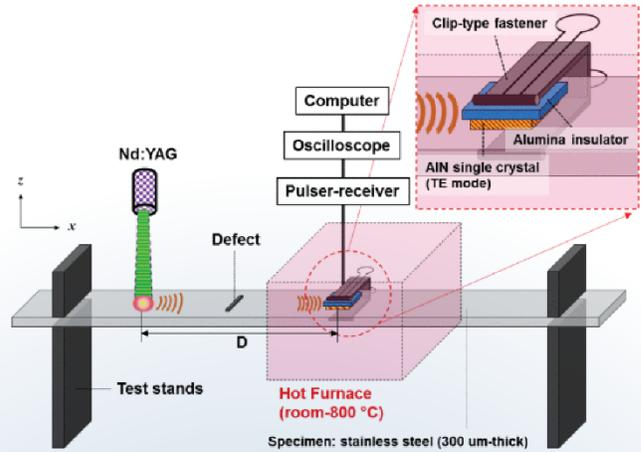
Figure 5. Laser-assisted HT damage detector [10].
