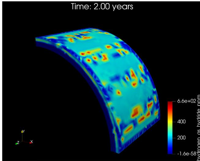
Figure 4. FE simulations of hydride evolution
