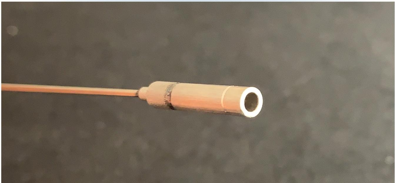
**Figure 3.** Image of prototype fiber optic pressure sensor.
