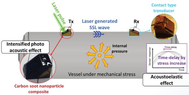
Figure 3. Laser assisted stress sensor [9].
