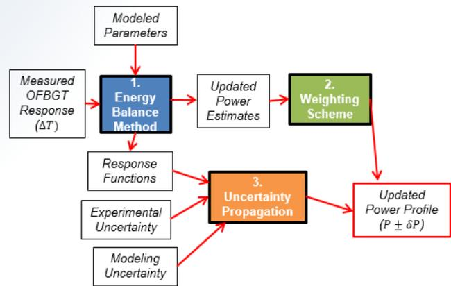
Figure 5. OFBGT data analytic methodology.
