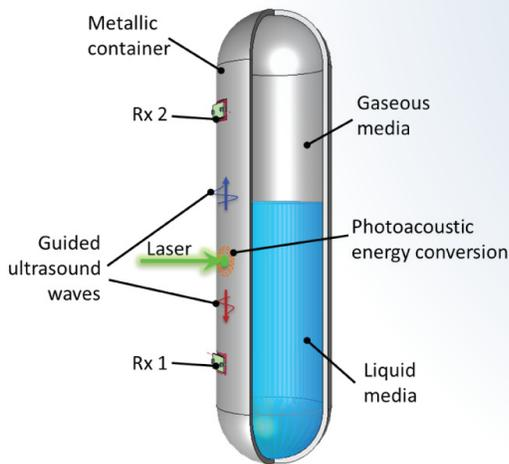
Figure 4. Laser-assisted HT liquid level sensor.
