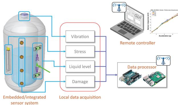
**Figure 1. Overview of HiTEIS with the wireless data communication.**
