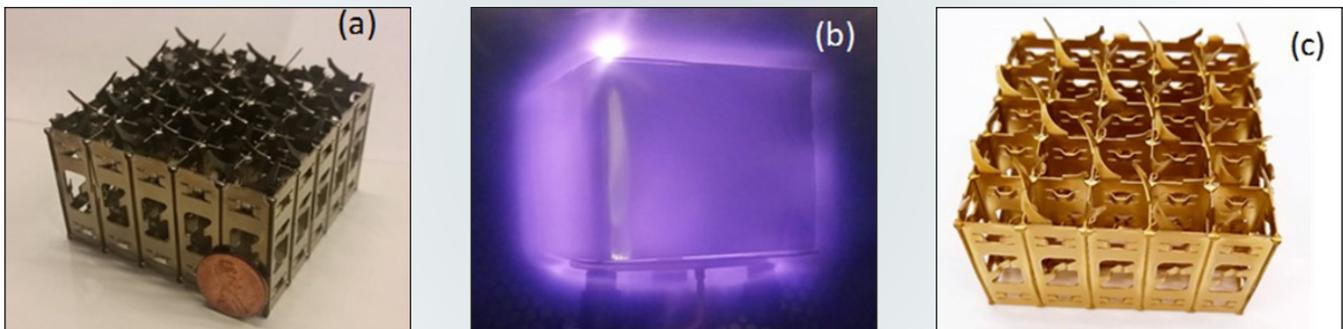
**Figure 3.** Images of Westinghouse fuel assembly spacer samples (a) before nitridation, (b) during the nitridation, and (c) after the nitridation. The golden color after nitridation comes from nitride layers forming on the surfaces.
