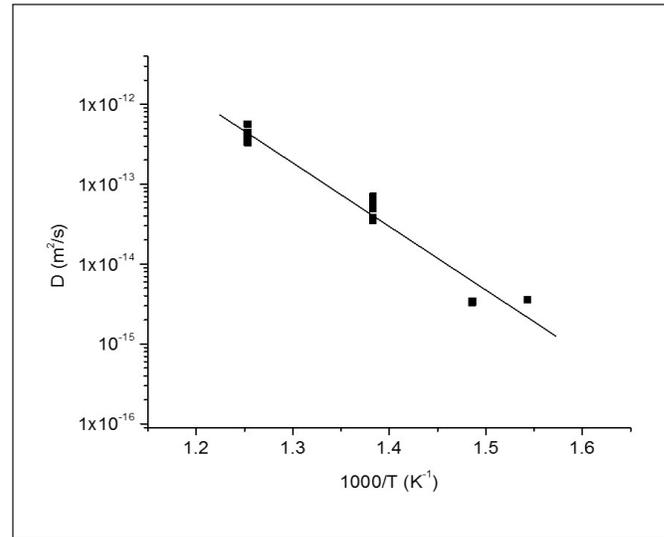
**Figure 2.** Extracted nitrogen diffusivities as a function of nitridation temperatures in nitrided 316L.
