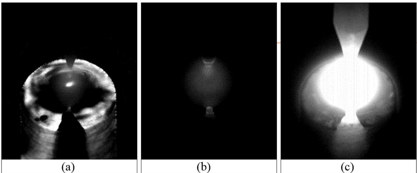
*Figure 2. VIS images obtained by: (a) short exposure time and laser illumination, (b) short exposure time without laser (c) long exposure time without laser.*
