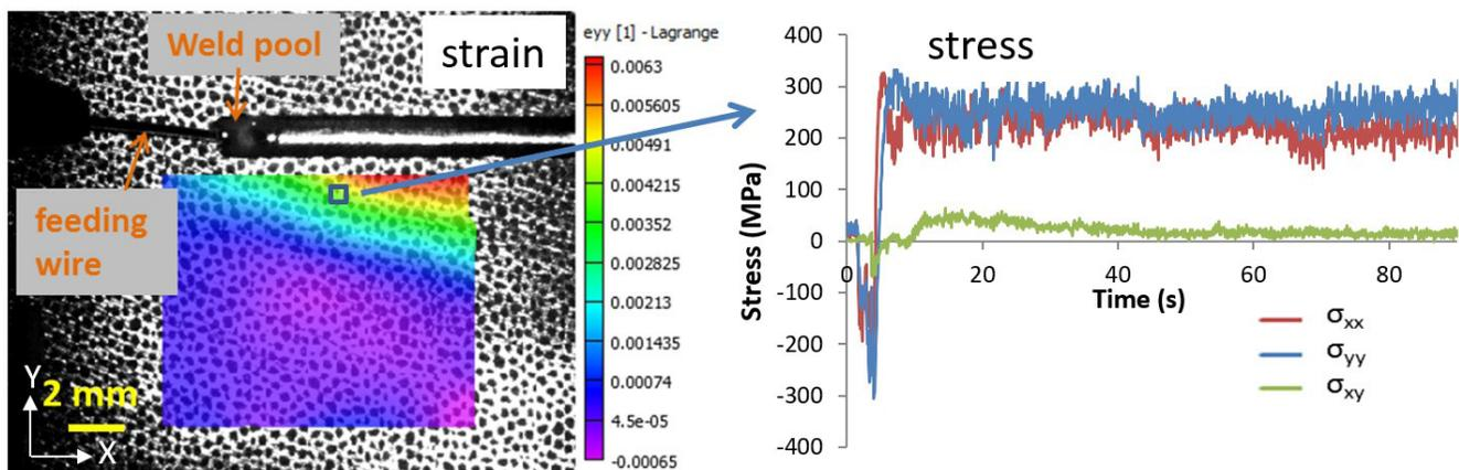
Figure 4. Transverse strain distribution and stress evolution during laser welding.
