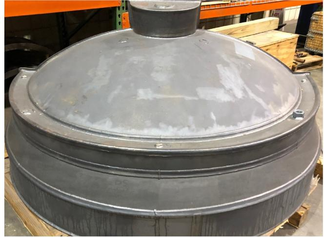
**Figure 3. A 2/3-scale, one-half diameter lower reactor head (~70 inches (1780mm) in diameter, 6910lbs (3135kgs) was also produced via PM-HIP.**
