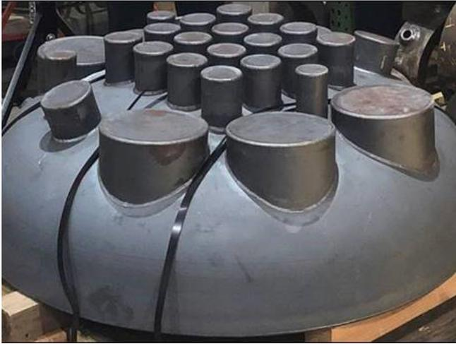
**Figure 2. A 44 percent diameter (50-inch, 1270mm) A508 Grade 3, Class 1 upper reactor head that includes 27 penetrations and weighs 3640lbs (1650kgs) was produced via PM-HIP**
