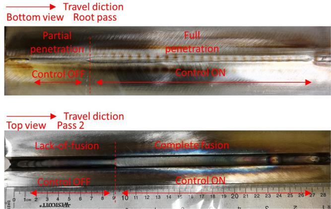
Figure 3. Adaptive control to achieve full-penetration on the root pass and complete side-wall fusion on the subsequent weld pass.
