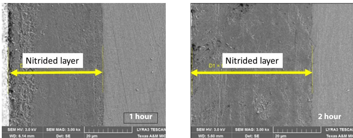
**Figure 1.** Scanning electron microscope images of nitrided 316L cross sections after nitriding at 525°C and 1.5 Torr for one hour (left) and two hours (right). The dark contrast regions are nitrided layers due to plasma nitridation.
