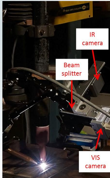
*Figure 1. Multi-optical sensing system.*
