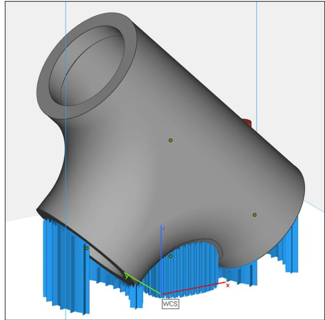
**Figure 2.** The pipe tee fitting is shown in a supported condition as it will be additively manufactured.
