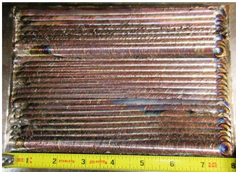
**Figure 1. 304 SS piece cladded on A516 substrate by FSAM**
