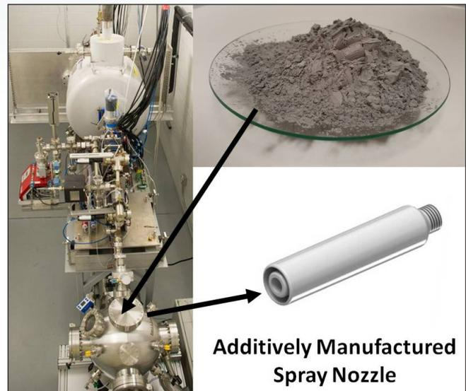
**Figure 1. Additive manufacturing of steel components, such as spray nozzles, from powder for SMRs using Mainstream's high-energy, high-power EBEAM facility.**
