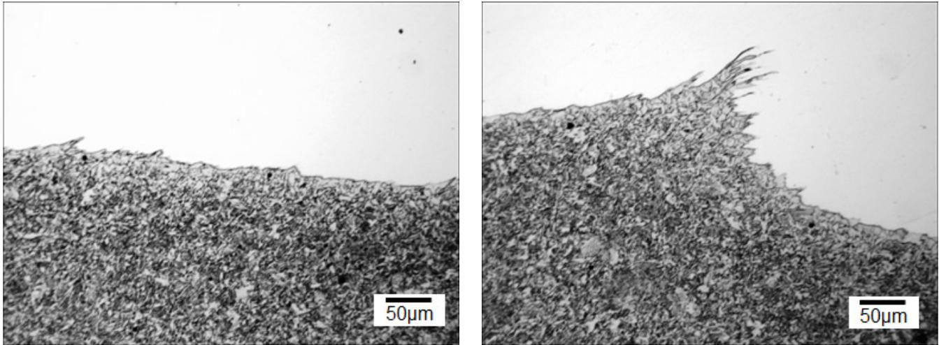
**Figure 2. Bonded 304 SS and A516 PVS interface after FSAM**
