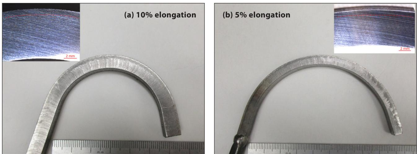
**Figure 3. Mandrel bend test with different elongation at the FSAM interface**
