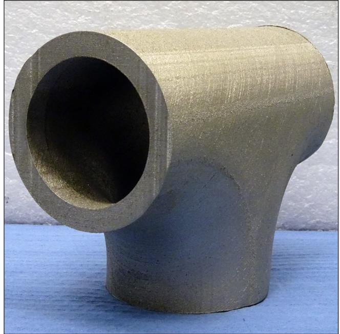
**Figure 4. A 316L SS pipe tee fitting produced by LPB-AM.**
