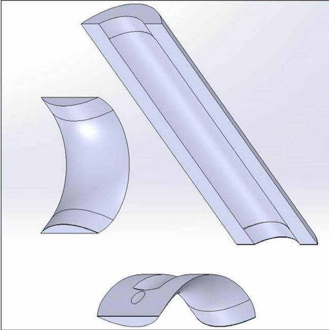
**Figure 3. Critical sections of the 316L SS pipe tee fitting have been produced by LPB-AM for characterization.**
