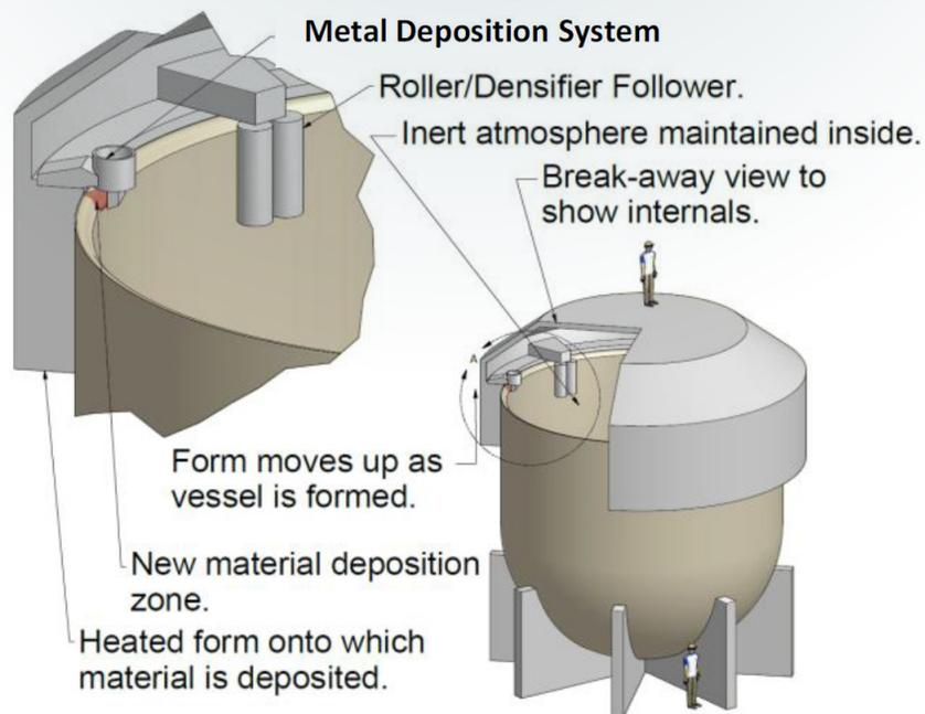
*Figure 1. Concept of fabrication of large pressure vessel.*
