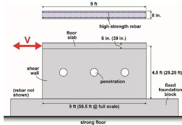
Figure 5. Preliminary cross-section (top) and elevation (bottom) views of reduced-scale capstone shear wall specimens.
