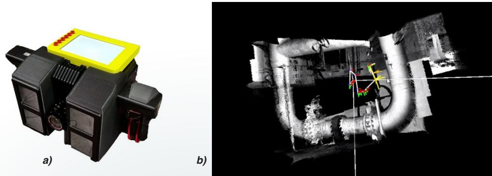
**Figure 2.** Phase II handheld 3D video camera (a) will be coupled with optimized registration software to create near real-time as-built models of large plant areas. Preliminary testing with DotProduct's Phi3D software created a registered point cloud (b) in less time than it took to take the data (4 sec registration for 10 sec of data).
