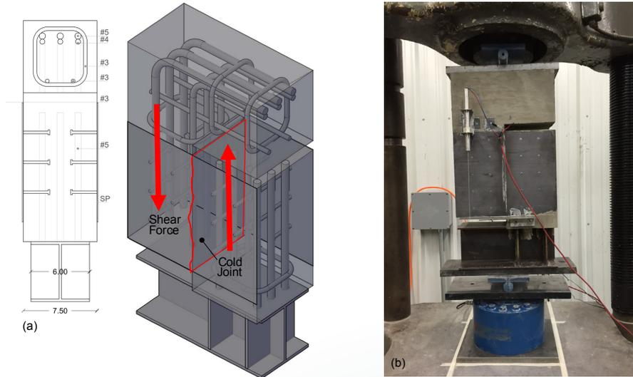
**Figure 2. Small-scale push-off specimen: (a) specimen consists of two L-shaped concrete placements with a cold-joint boundary running vertically, with the two placements joined by steel composite plates on two opposite sides of the specimen and (b) the specimen is loaded in a compression fixture, which generates shear across the cold-joint boundary. The slip along the cold-joint boundary is measured with two linear variable differential transformers.**
