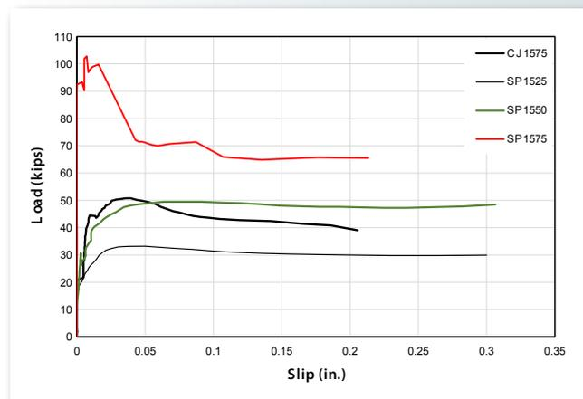
**Figure 3. Load versus slip relationship for four different specimen configurations and tested as shown in Figure 2. Specimen CJ1575 (solid line) is a baseline specimen that is reinforced with internal concrete reinforcement. SP1525, SP1550, and SP1575 represent steel plate composite specimens with 0.25%, 0.50%, and 0.75% external reinforcement.**
