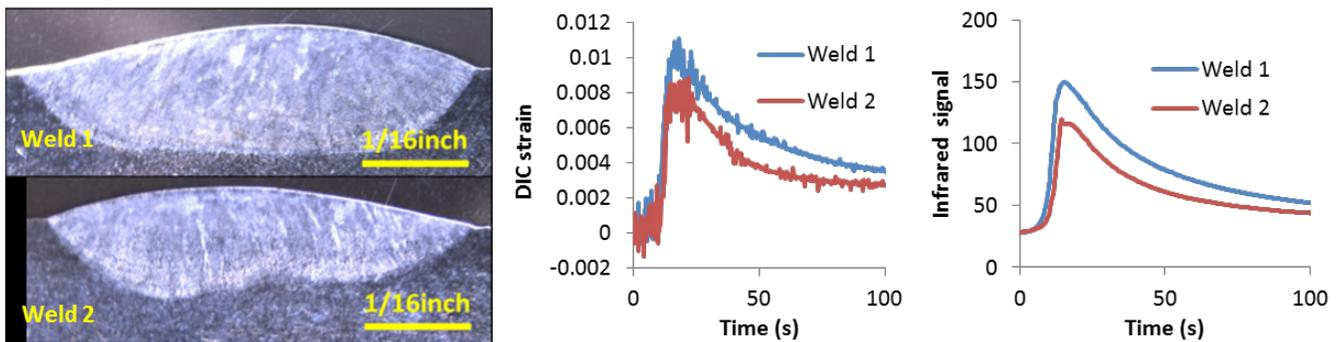
**Figure 2. Variation of in-situ strain and IR signals positively correlates to a certain weld defect (Weld 1 - normal size; Weld 2 - undersize).**
