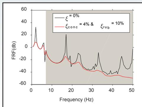
Figure 5. Attenuation zones of Unit Cell 3.
