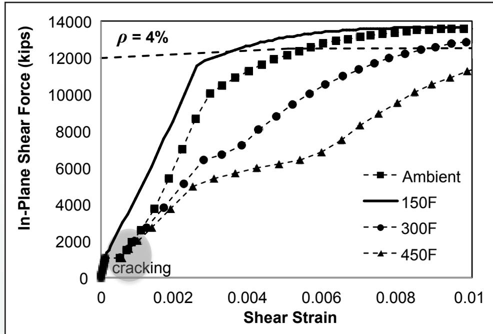
Figure 3. Effects of accident thermal loading on the in-plane shear behavior of SC walls.
