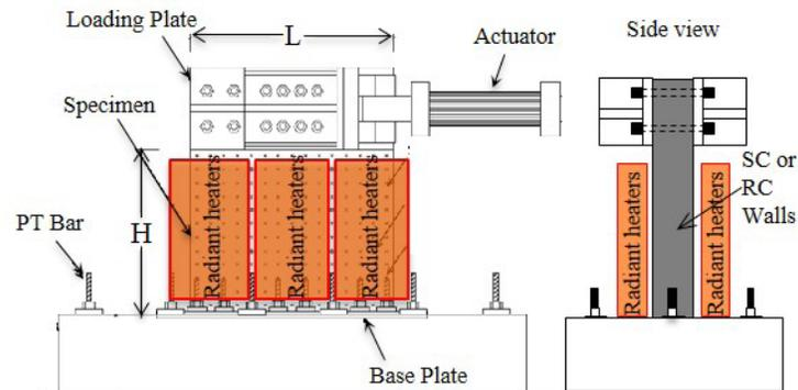
**Figure 2. Test setup for conducting accident thermal plus lateral loading tests.**
