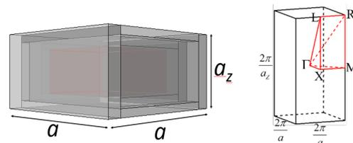
Figure 2. (a) Suppressed unit cell in vertical direction and (b) first irreducible Brillouin zone.
