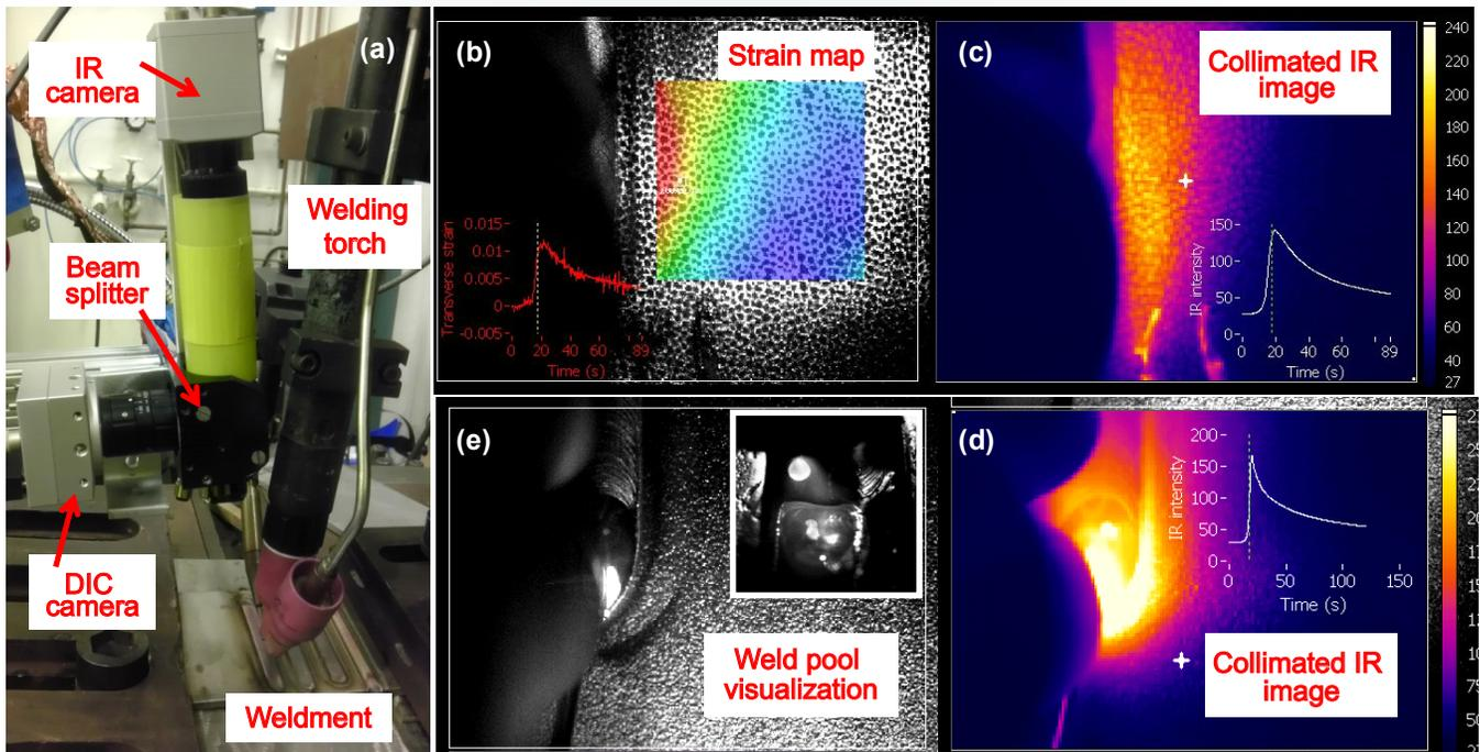
Figure 1. Integrated optical sensing technology for welding in-situ monitoring.
