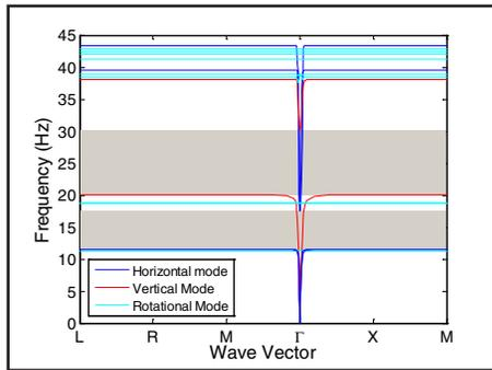
Figure 3. Dispersion curve of unit cell suppressed in the vertical direction.
