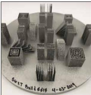
**Figure 7. Hastelloy® X thin wall test builds.**
