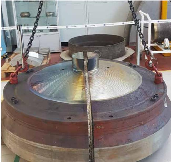
**Figure 4.** A completed EB weld joining two halves of the lower reactor vessel head. Note that the head is upside down and final machining has yet to be completed.
