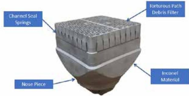
Figure 4. Monolithic additive manufactured BWR lower tie plate.
