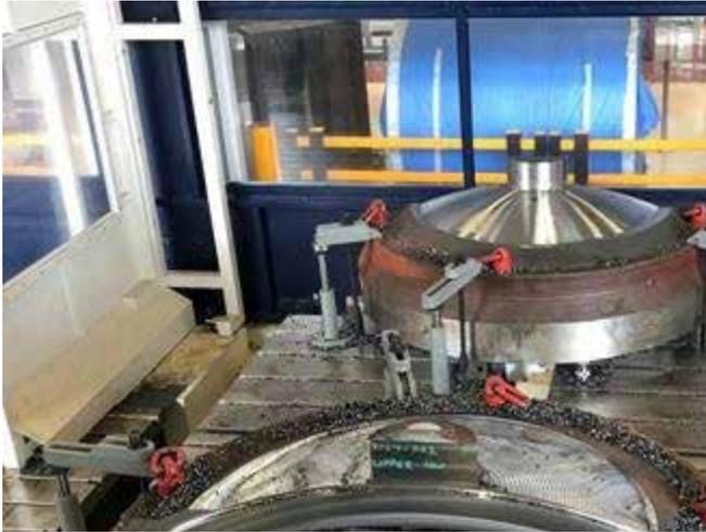
**Figure 2. Machining of two halves of the lower head in preparation for EB welding at the Nuclear-AMRC.**
