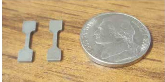
**Figure 2. Sub-miniature tensile test specimens.**
