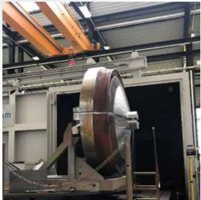
**Figure 3. Removal of the lower reactor head from the Nuclear-AMRC's EB welding chamber.**
