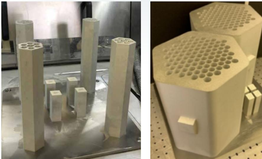
**Figure 2. (a) Four 280 mm tall 7-hole test articles on the build plate and (b) two 292-mm-tall 37-hole pipe test articles on the build plate.**
