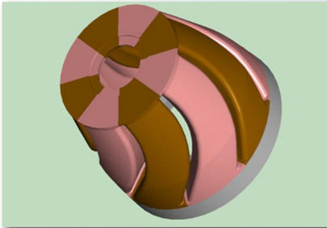
Figure 3. ALWR steam separator inlet swirler model.
