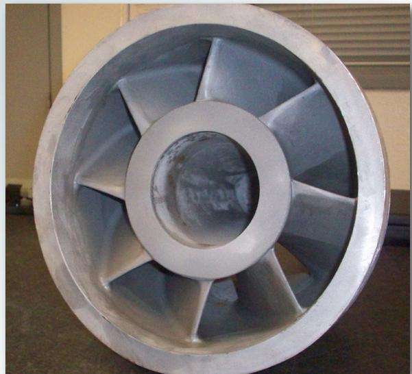
Figure 2: ALWR steam separator inlet swirler.
