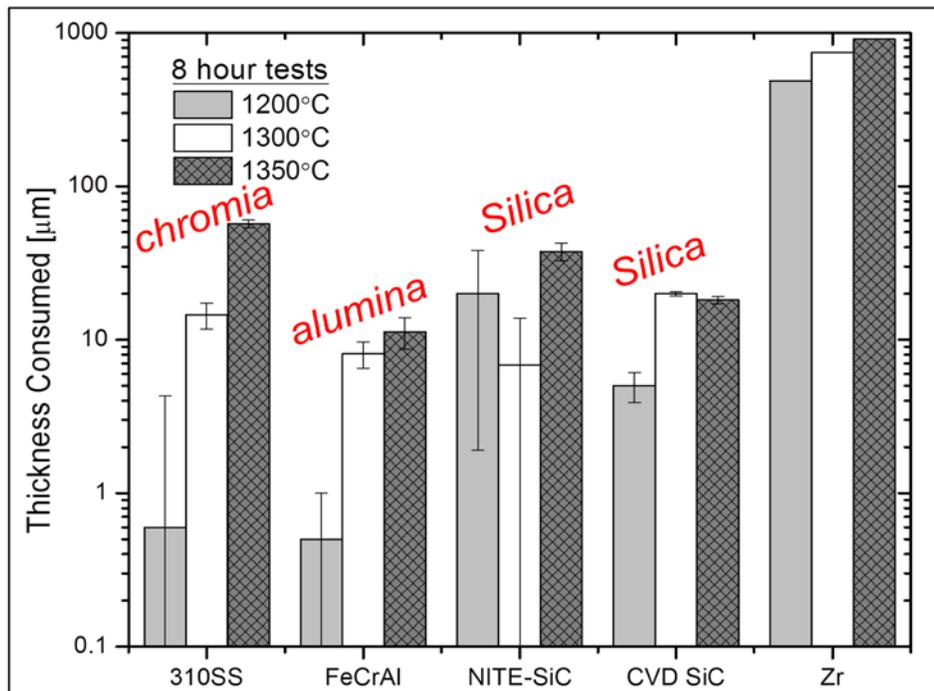
Figure 3. Clad thickness loss for candidate materials in flowing steam at 1 MPa [4].
