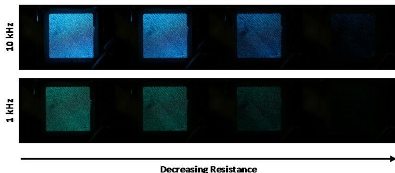
Figure 2. Optical response of 3D-printed ‘smart coating’ with decreasing resistance at various levels of excitation.
