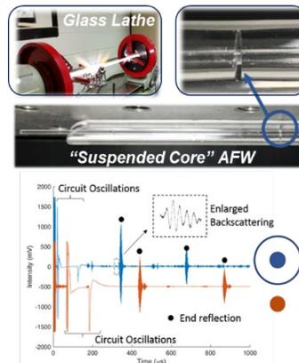
Fabrication and testing of “Suspended Core” fused silica AFW.
