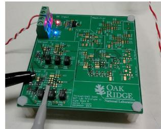
The electronics system PCB (partially populated) used to collect sensor signals and drive the through-wall communications.
