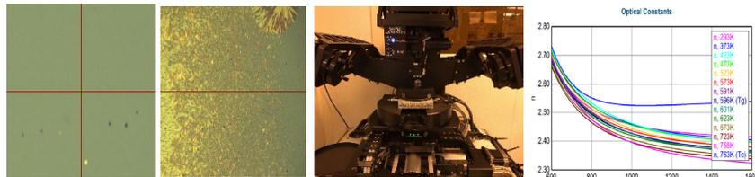
Figure 1. Amorphous and crystallized films after reaching crystallization temperature; Test equipment for in situ optical characterization; Measured optical performance of the films.
