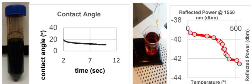
Figure 2. Powder ink; Contact angle of ink measurement; fiber top cleaning; Optical data as a function of temperature.
