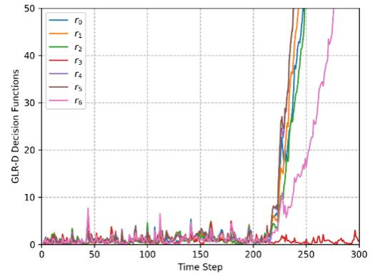
Decision functions for change detection for a sensor fault.
