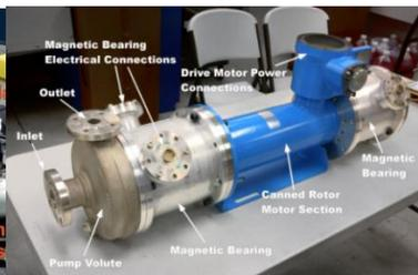
*Loop-Scale Magnetic Bearing Test Bed.*
