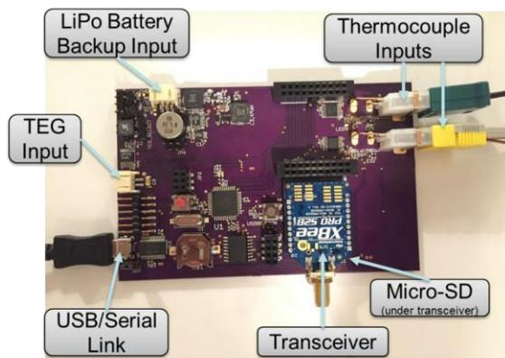
*Thermoelectric generator powered wireless sensor node prototype.*
