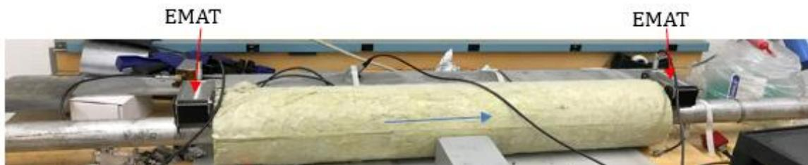
*Setup of Lamb Wave EMAT to EMAT signal transmission along a stainless steel schedule-160 pipe with thermal insulation.*
