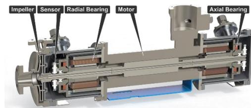
*Cross-Section of 10 hp Magnetically Suspended Canned Rotor Motor.*
