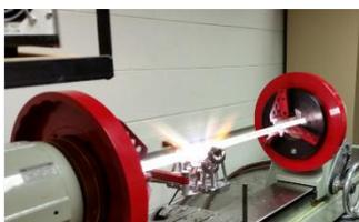
Automated glass working lathe for fused silica AFW fabrication
