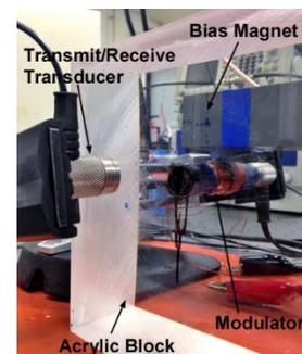
*Dual element transducer system tested on the 4 inch acrylic block.*
