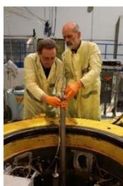
Fiber sensor lowered into the test react
