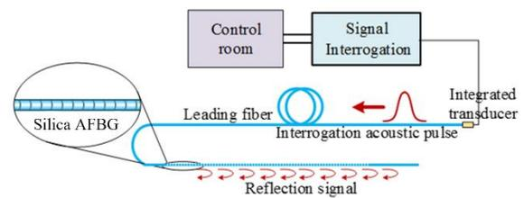
Schematic of AFBG sensing system.
