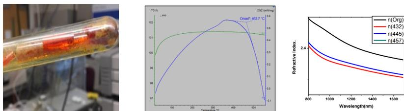
*Figure 1. Ampoule with  $Ge_{30}Se_{70}$  glass; Differential scanning calorimetry and refractive index data.*
