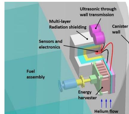
*Energy harvesting for sensing and communicating system powering.*
