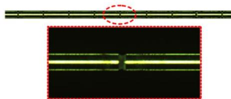
Optical micrograph of silica AFBG array.
