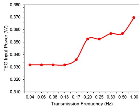
*TEG input power versus frequency of data transmission.*
