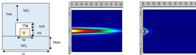
*Figure 2. Device structure; light propagation in amorphous and crystalline states.*
