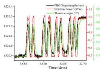
FBG in (black) response to neutron power change (red) compared with thermocouple measurements (green).
