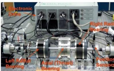
*Bench-Scale Magnetic Bearing Test Bed.*
