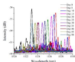
FBG peak shift in the reactor from Day 0 to Day 50 for specially design radiation-harden fibers
