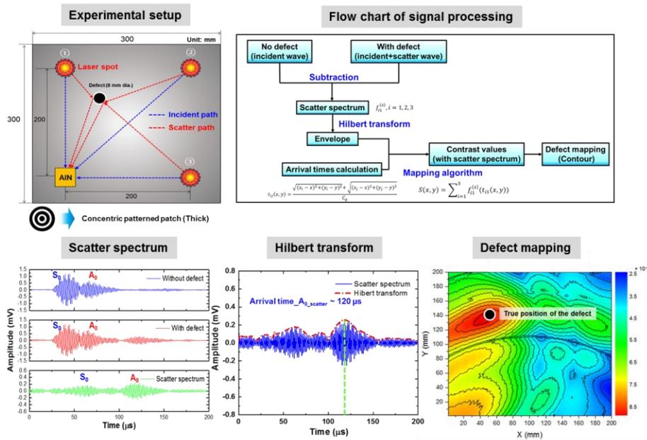
*Photoacoustic Lamb wave non-destructive testing technique with candle soot/PDMS patches.*
