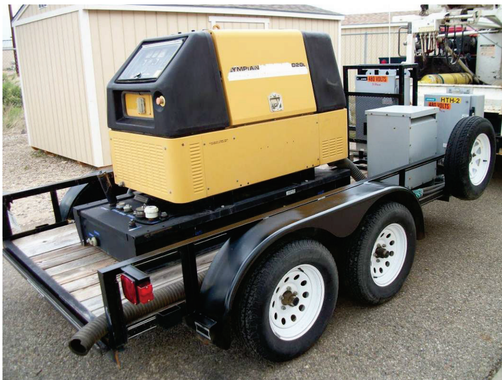
Figure 1. Olympian 20-Kilowatt Generator
