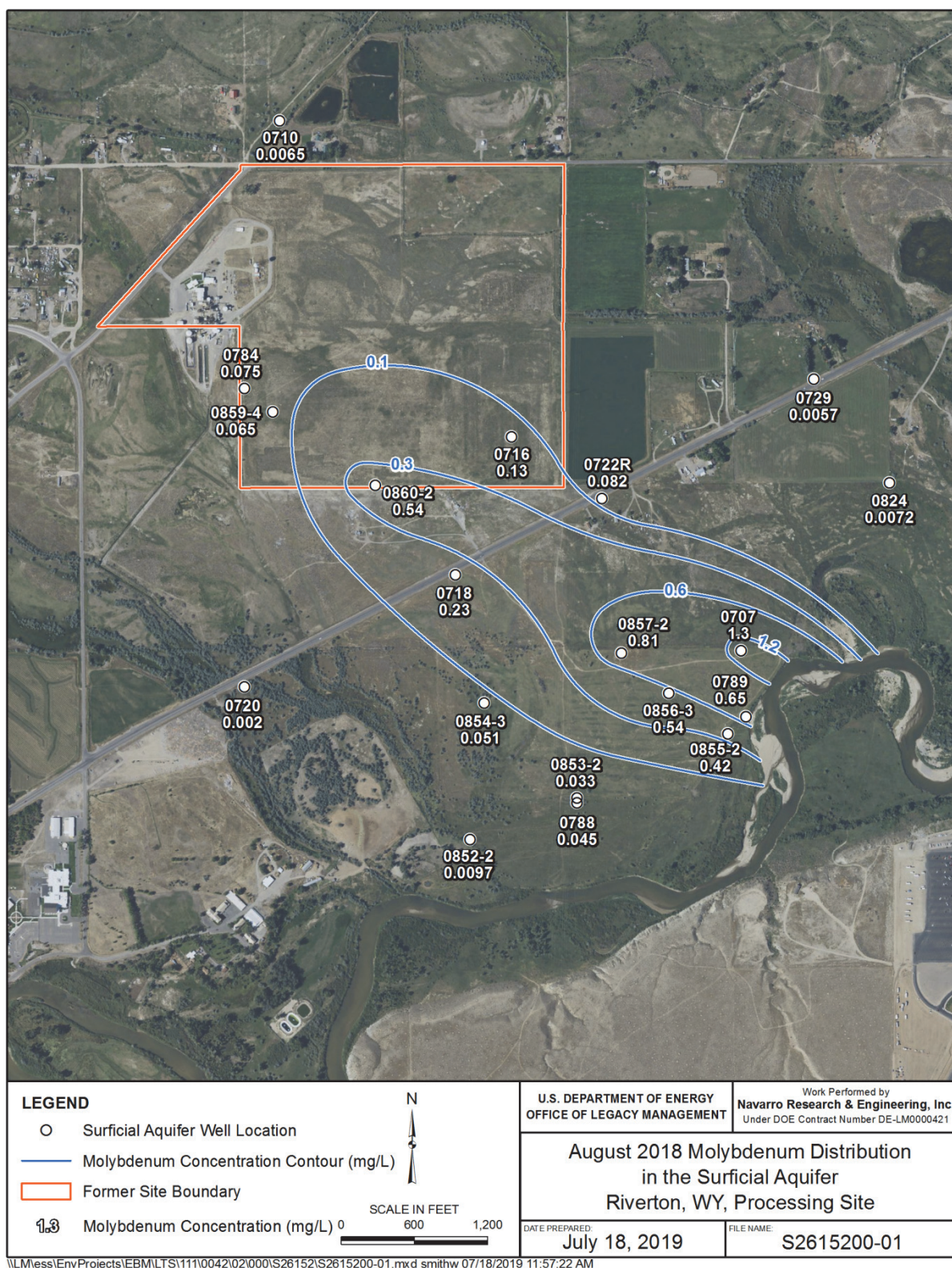
Figure 5. Molybdenum Distribution in the Surficial Aquifer at the Riverton Site in August 2018 (after DOE 2019)
