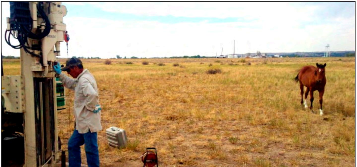
*A member of the field team operates a geoprobe machine for sampling.*
