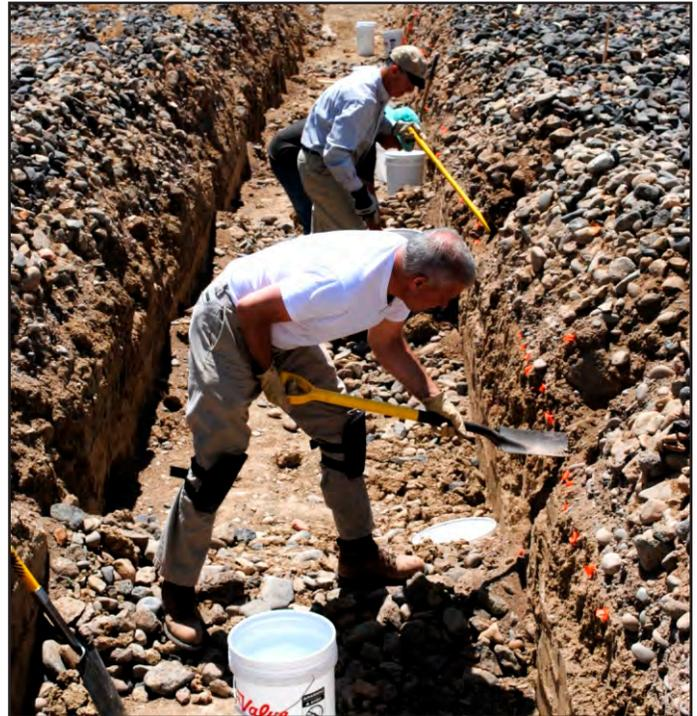
Figure 3. ECAP collaborators collecting bulk samples as part of an evaluation of cover enhancement alternatives.
