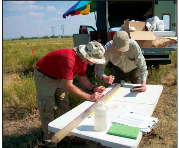
*Bill Dam, on detail from U.S. Geological Survey, and an LM contractor employee examine a soil core collected inside a plastic tube.*
