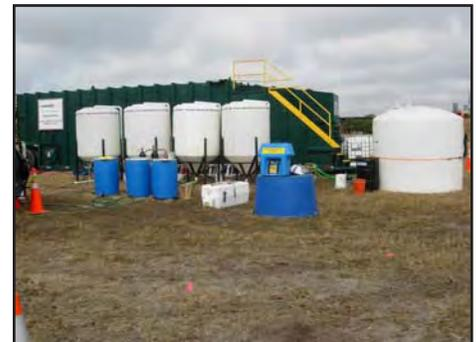
Figure 2. Photo of mixing and injection setup.
