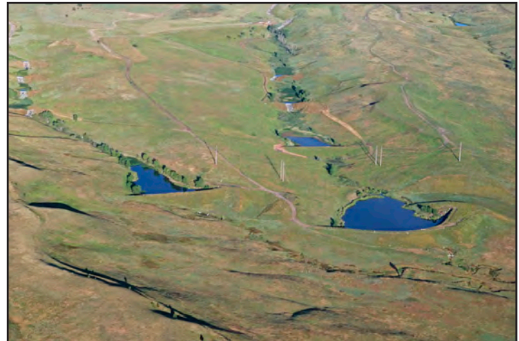
The terminal pond dams B-5 on south Walnut Creek, left, and A-4 on north Walnut Creek, center front, will be breached in the 2018 to 2020 timeframe. The A-3 dam, center back, and the Present Landfill pond, far right back, are scheduled to be breached in the fall of 2011. The armored channels upstream of the A and B ponds indicate locations where smaller dams were breached in the past.
