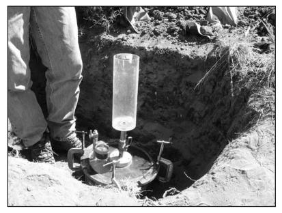
Results of air-entry permeameter tests conducted at the Lakeview, Oregon, Disposal Site were used to evaluate the permeability of the disposal cell cover.
