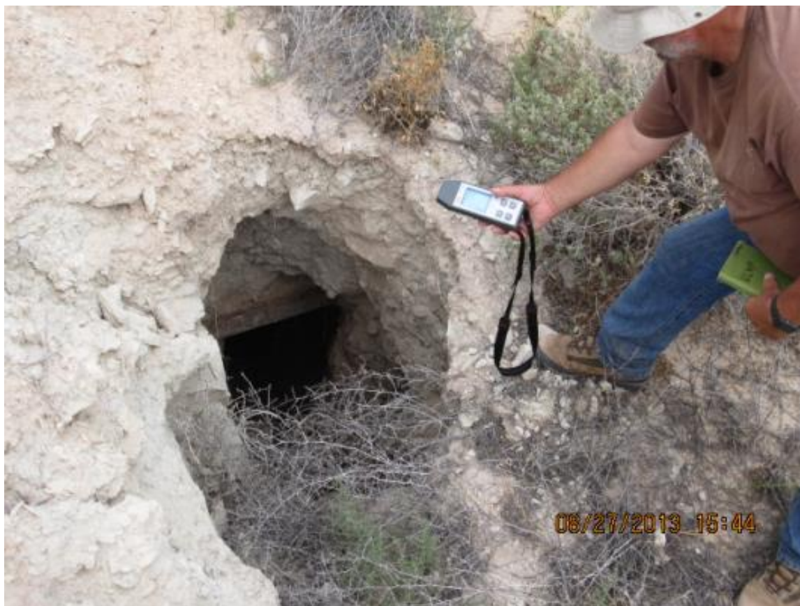
Figure 18. Collecting Gamma Measurements at Mine Opening, Yellow Cat District, Utah
