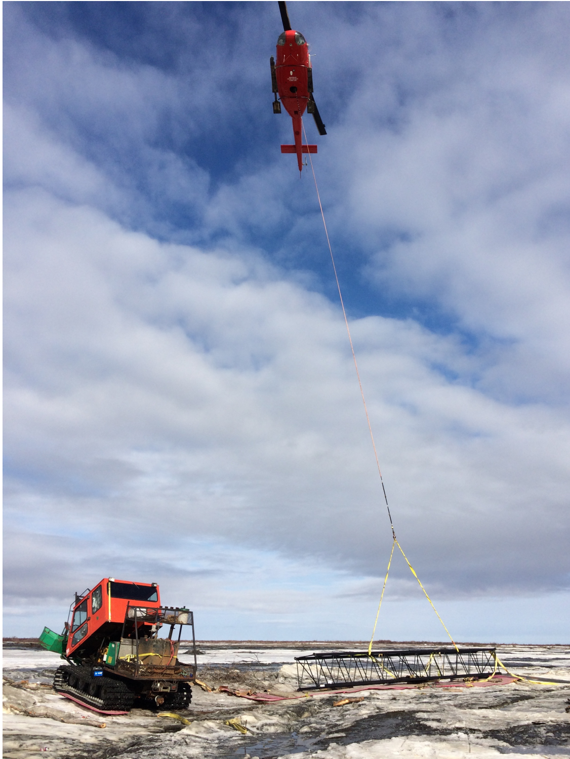
Sno-Cat and helicopter pictured transporting the crane boom to Kongiganak
