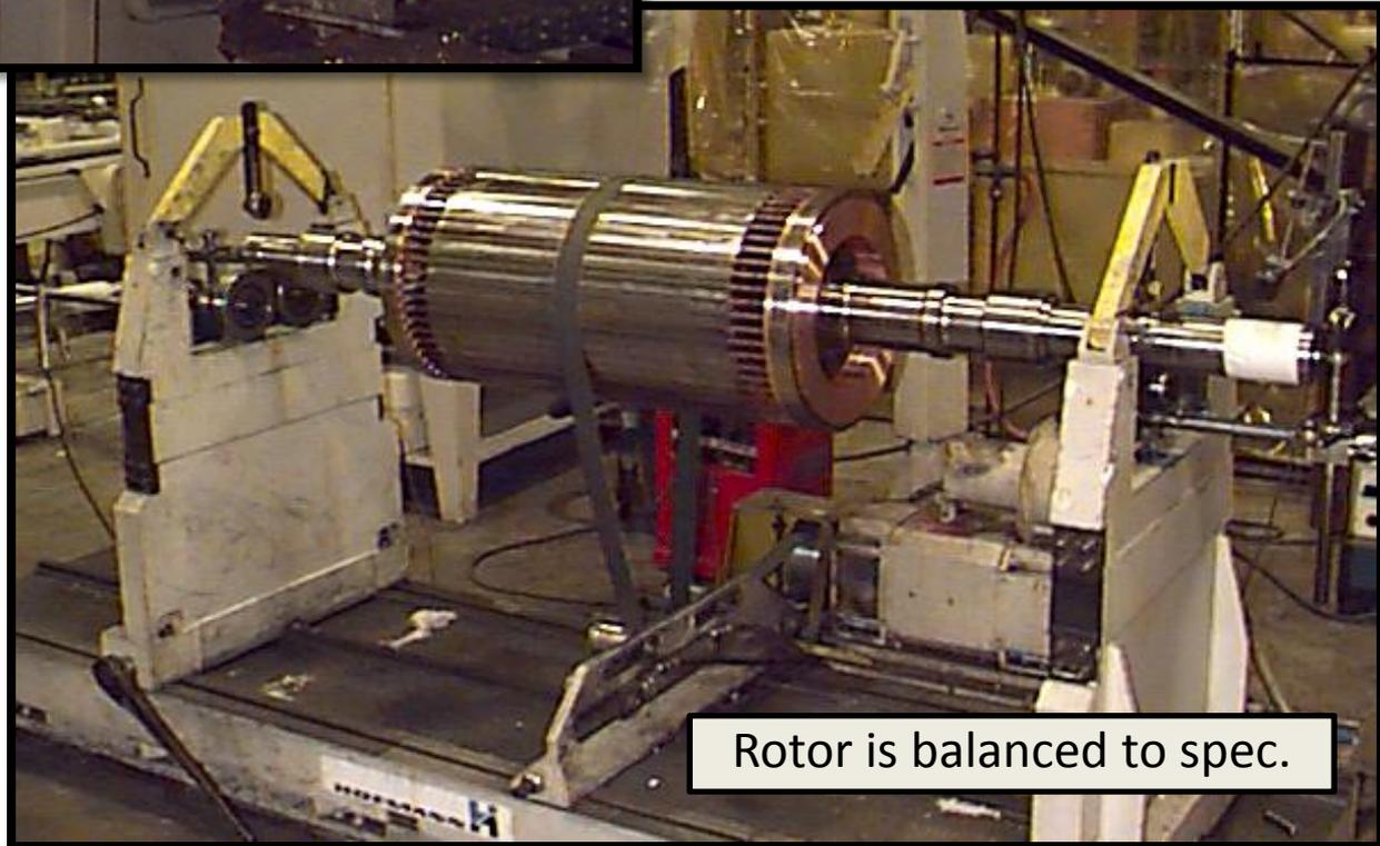
Rotor is balanced to spec.
