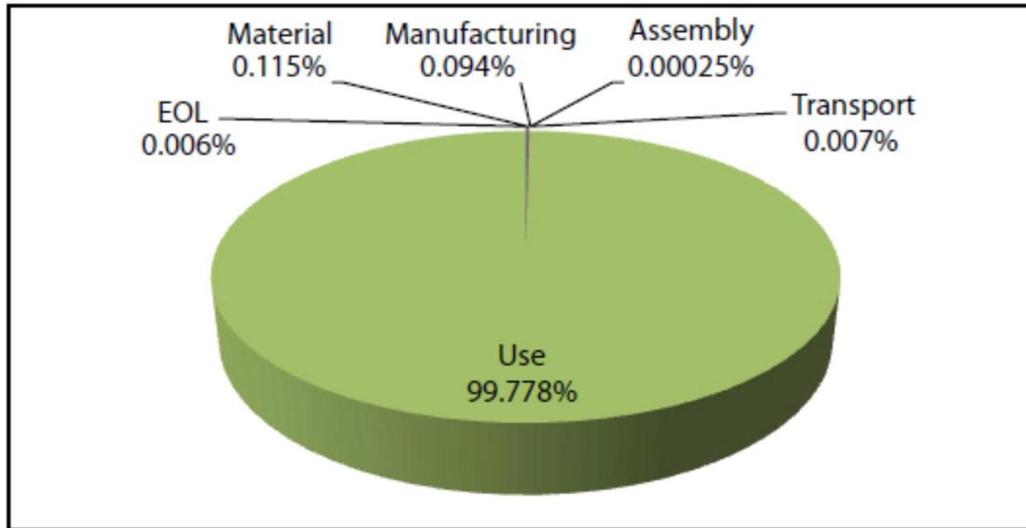
**FIGURE 20.** Overall life impact (GWP Impact, mean value) for a 25 HP NEMA premium motor
