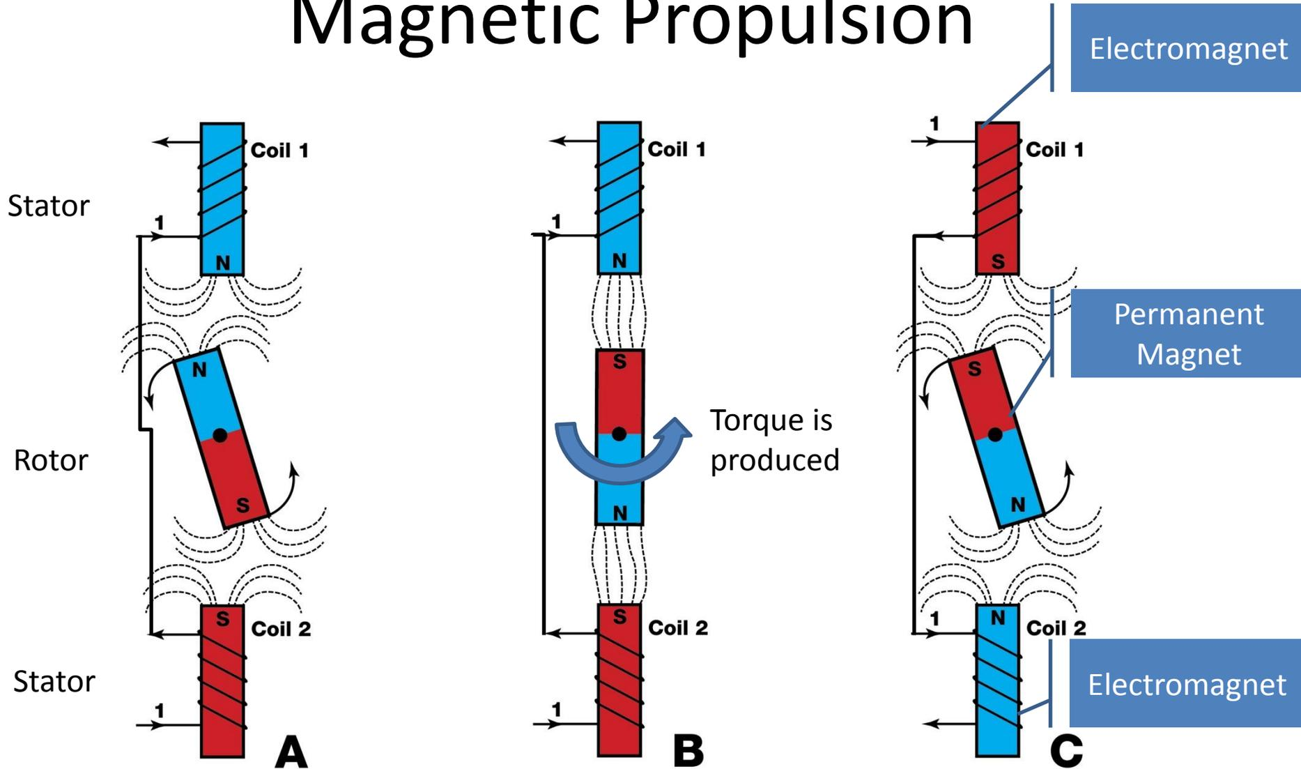
The principle of an induction motor is to induce magnetic forces into the rotor of the motor. A new generation of motors has permanent magnets imbedded in the rotor
