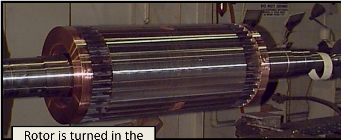
Rotor is turned in the lathe to size.
