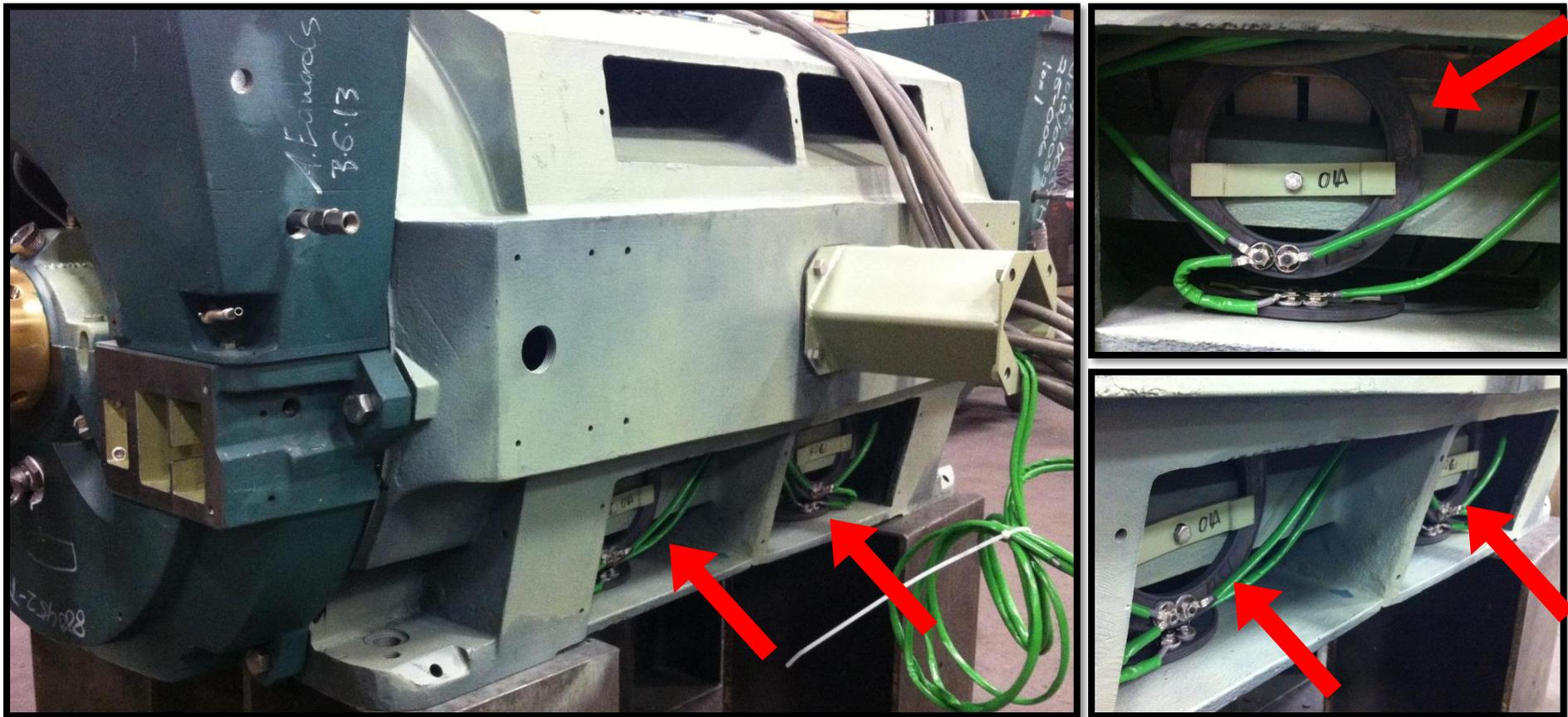
Ring Type Replaceable Heater installed in frame stringers.
